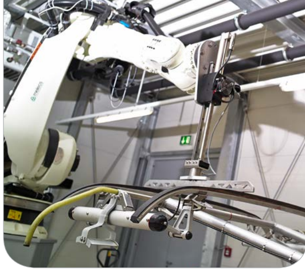
Dynamic pantograph testbed with realtime catenary simulation
