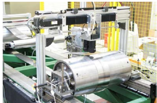
Test bed for assessing the operating performance of process belts
