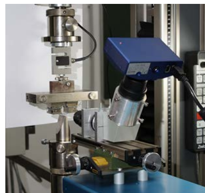
Bending tester with microscope to study crack propagation in PE-UHMW
