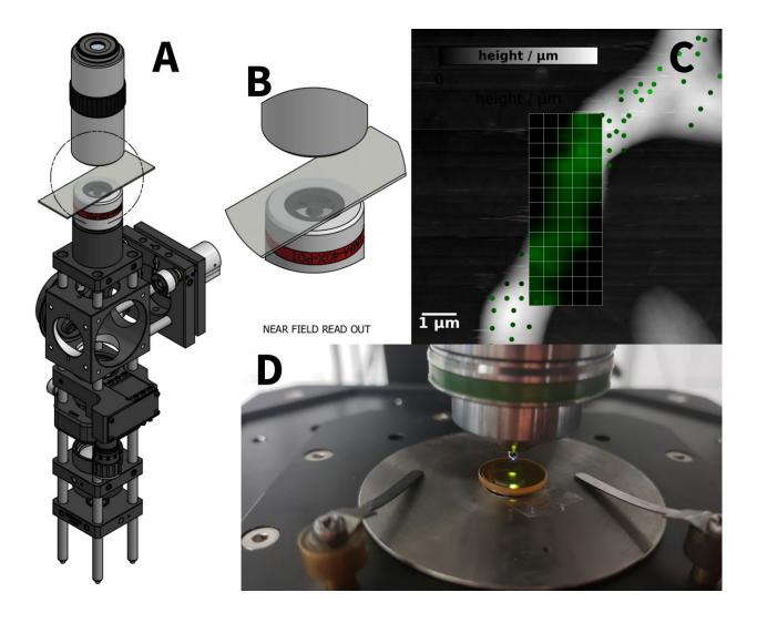
A) sketch of super resolution imaging system. B) Detail view of confocal read out C) Computational staining of fungal hypha at 100 nm spatial resolution D) Chemical and scanning probe imaging in the same location
