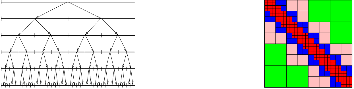
Figure 5.1: Left: organizing the degrees of freedom in a tree structure in 1D. Right: block structure for the 1D example
