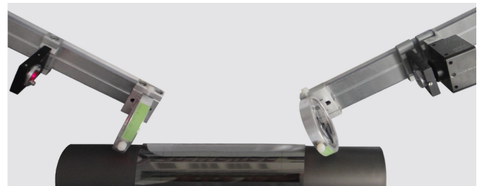
Inline measuring system without moving parts (basic concept)
