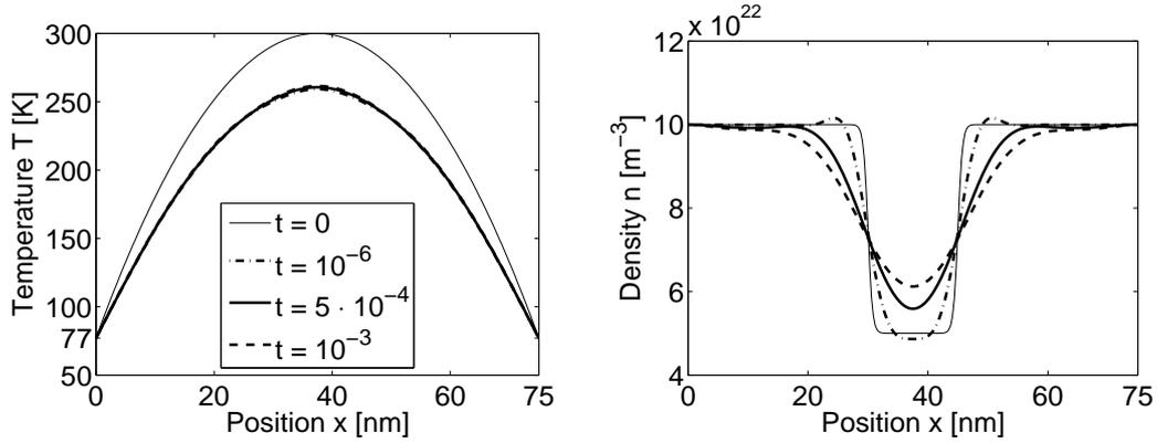
FIGURE 4. Dirichlet-Neumann boundary conditions, case (ii),  $U = 0$ : Electron temperature (left) and electron density (right) at various times.
