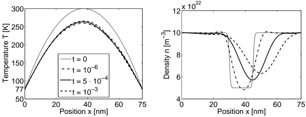
FIGURE 6. Case (ii), Dirichlet-Neumann boundary conditions,  $U = 1$  V: Electron temperature (left) and electron density (right) at various times.
