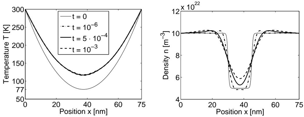
FIGURE 3. Dirichlet-Neumann boundary conditions, case (i),  $U = 0$ : Electron temperature (left) and electron density (right) at various times.
