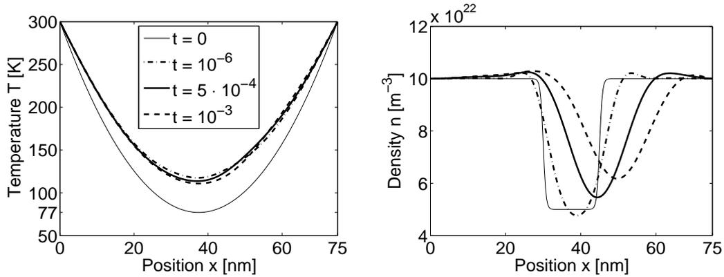
FIGURE 5. Case (i), Dirichlet-Neumann boundary conditions,  $U = 1$  V: Electron temperature (left) and electron density (right) at various times.
