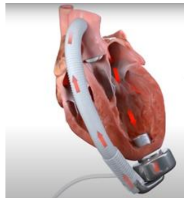
Figure 1. Schematic diagram of an implanted rotodynamic blood pump.
