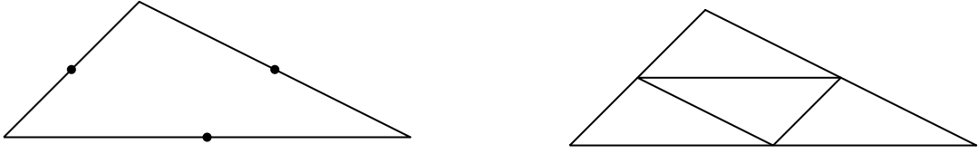
FIGURE 4.3. Red-refinement: If all edges of a triangle T \in \mathcal{T}_\ell are marked (left), T is refined into four similar triangles T_1, T_2, T_3, T_4 \in \mathcal{T}_{\ell+1} (right).
