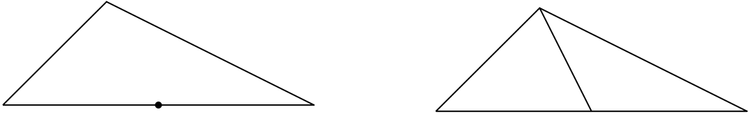
FIGURE 4.4. Green-refinement: If only the longest edge of a triangle T \in \mathcal{T}_\ell is marked (left), T is refined into two new triangles T_1, T_2 \in \mathcal{T}_{\ell+1} (right).
