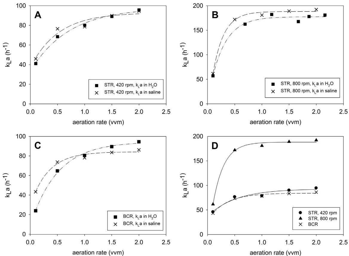
**Fig. 2.** Volumetric mass transfer coefficient  $k_L a$  depending on liquid, reactor type and stirrer speed. (A), (B) and (C): Comparison of  $k_L a$  values in saline medium and deionized water in STR and BCR. (D): The effect of the reactor type and stirrer speed on  $k_L a$  values in saline medium (150 g/L NaCl).
