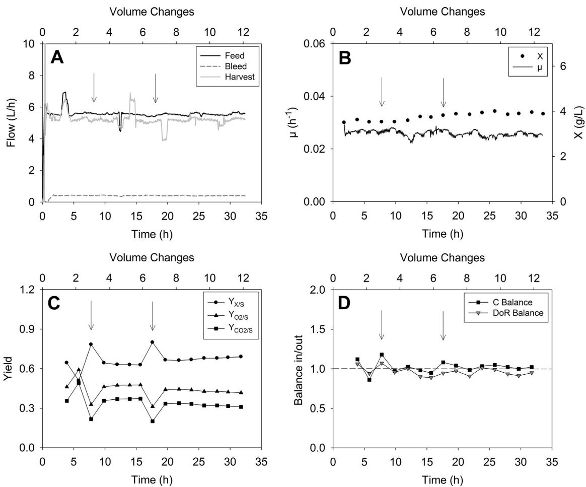
**Fig. 4.** Time dependent profile of flows (A), yields (B), specific growth rate  $\mu$  and biomass concentration X (C) and carbon and degree of reduction balance (D). Continuous cultivation of *H. mediterranei* on glycerol in BCR. Arrows indicate pressure reduction due to addition of antifoam.
