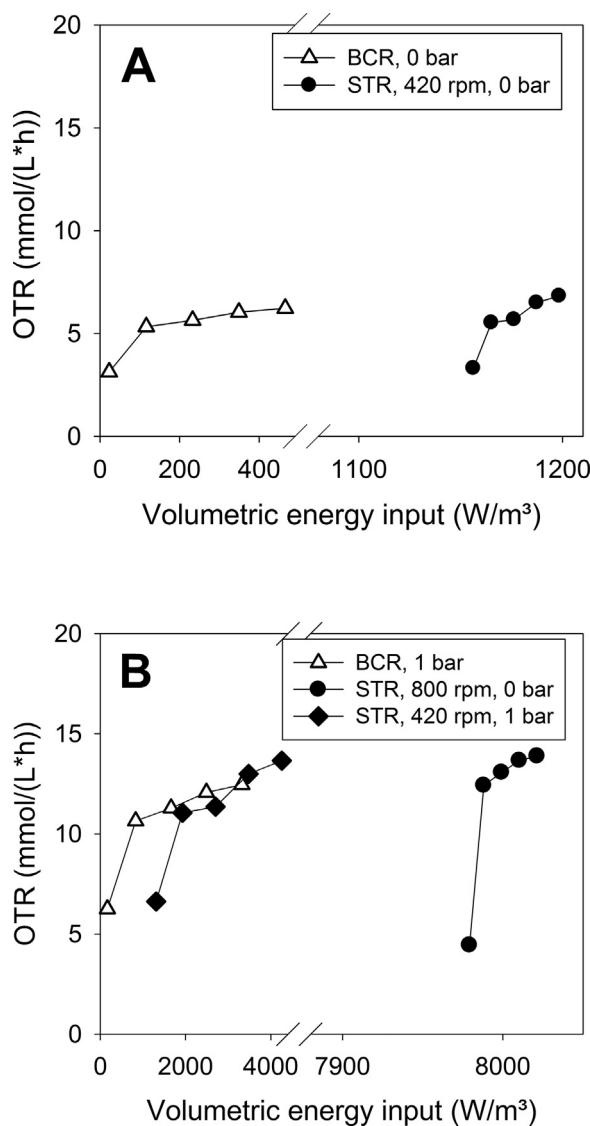
**Fig. 3.** Oxygen transfer rate depending on the volumetric energy input for the two reactor systems STR and BCR at ambient pressure (A) and elevated reactor pressure (B).
