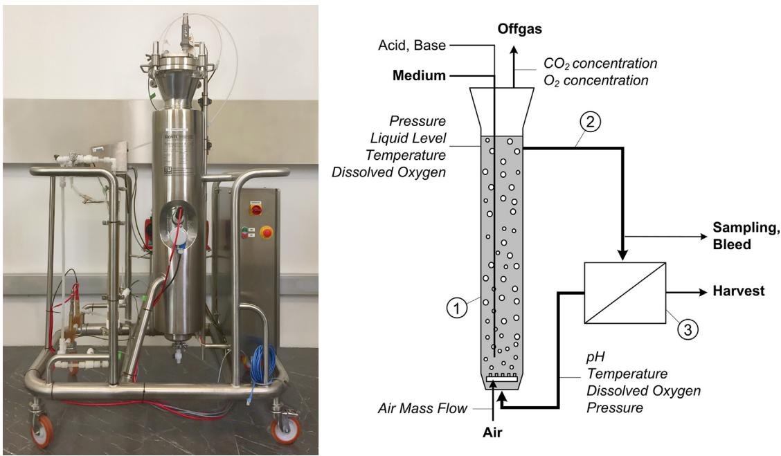
**Fig. 1.** Schematic diagram of the BCR: 1) Pressure resistant bubble column vessel, 2) continuously circulating loop driven by a diaphragm pump and 3) microfiltration unit for cell retention. Probes indicated in italic, continuous fluid flows indicated in bold.
