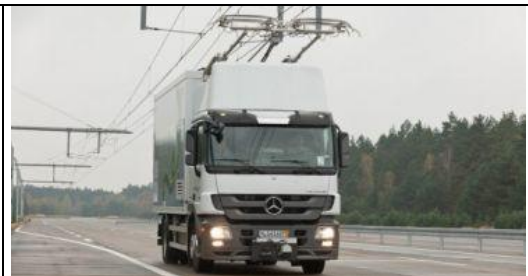
Motorways equipped with catenaries by SIEMENS
