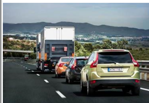
Car platoon autonomously following head truck close to Barcelona
