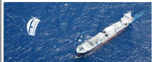
MS Beluga cargo ship is equipped with kite sails
