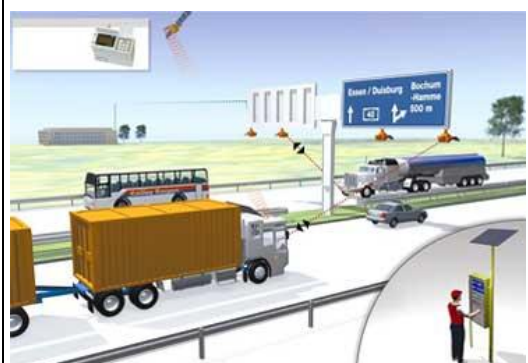
Scheme of smart truck road charging in Germany - LKW Maut
