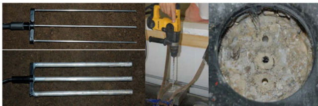
FIGURE 3 Left: Time-domain reflectometry (TDR) probes in original (top) and modified form (bottom). Centre: Drilling 8-mm access holes using a template. Right: Open 8-mm access holes for modified TDR rods
