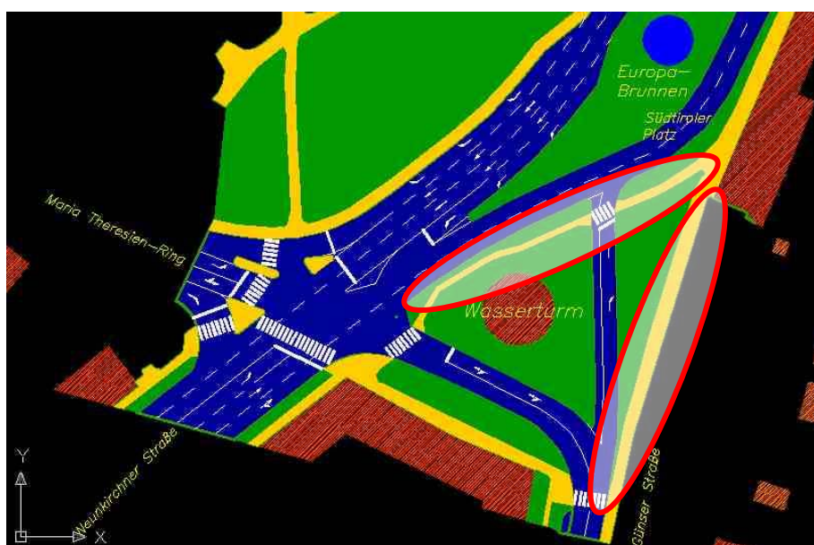
Figure 13 Map of planning solution number 3 (southern part), encircled in red improvements for pedestrians and/or cyclists.
