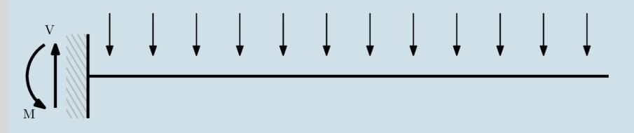
The maximal bending moment is equal to 111.3 aNm and the associated maximal axial stress is 446 Pa.
