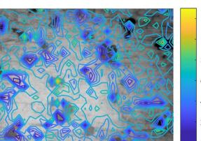
Stiffness gradients correlate with surface pores. Similar gradients in the lignin reveal pores below the surface.
