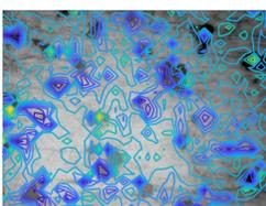
Stiffness gradients correlate with surface pores. Similar gradients in the lignin reveal pores below the surface.
