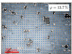
The pressing process introduced a porous microstructure with a different porosity for each lignin.
