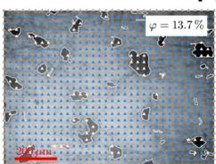
The pressing process introduced a porous microstructure with a different porosity for each lignin.
