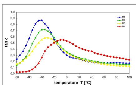
Validity of WLF theory is confirmed by comparison of experimental results (max.  $\mu$ ), e.g. for compounds M1 and M4
