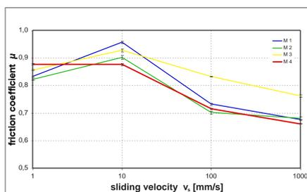
Experimental parameter: concrete surface, tread geometry G0, pressure  $p = 2$  bar, temperature  $T = 18$  °C
