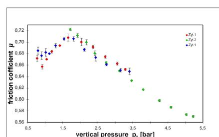
Experimental parameter: compound M1, concrete surface, tread geometry G0, sliding velocity  $v = 100$  mm/s, temperature  $T = 18$  °C
