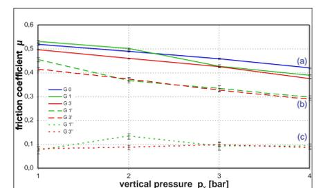
Experimental parameter: compound M1, asphalt surface, sliding velocity  $v = 1000$  mm/s, temperature  $T = 9$  °C
