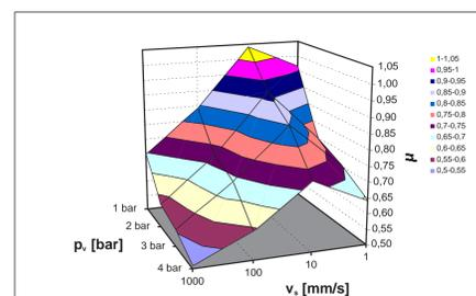
Experimental parameter: compound M1, concrete surface, tread geometry G0, temperature  $T = 18$  °C
