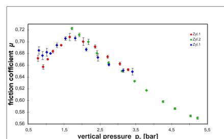
Experimental parameter: compound M1, concrete surface, tread geometry G0, sliding velocity  $v = 100$  mm/s, temperature  $T = 18$  °C
