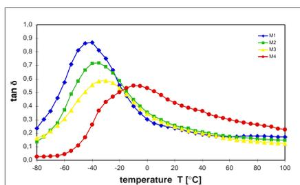
Validity of WLF theory is confirmed by comparison of experimental results (max.  $\mu$ ), e.g. for compounds M1 and M4
