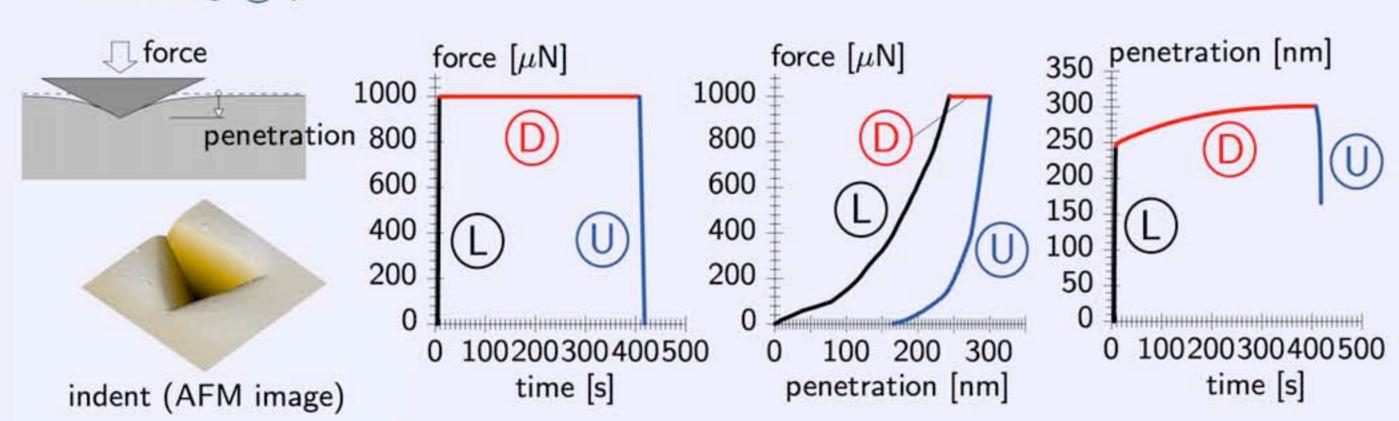
The load-time and penetration-time curves allow ...
