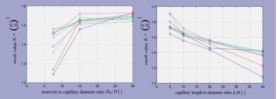
With the measured swell values various statements of the elastic behaviour of the investigated rubber blends are possible. From the rheological point of view the die swell occurs as a result The flow chart shows all required steps for the use of the generalized Newton-Raphson procedure. A validation for this method is done by means of a genetic algorithm.
