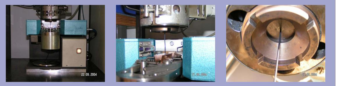
Alternative to the high-speed camera the strand diameter has been investigated by means of a laser beam with the so-called swell value measuring unit. The diameter of the investigated rubber blends increases after the capillary entry up to 16 % of the capillary diameter D.
