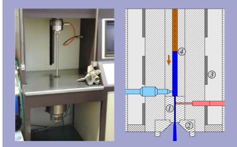
testing melt test stamp pressure sensor temperature sensor (1) capillary 2 capillary nut  $\bigcirc$  radiator 4 testing chamber
