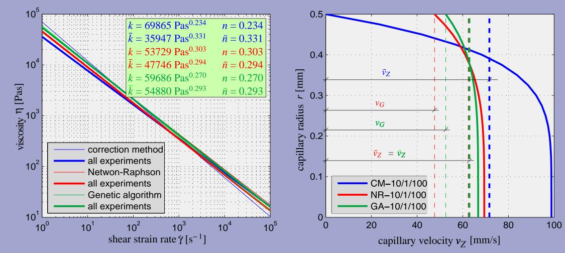
The comparison of the obtained viscosity curves leads to a good conformity. The nonlinear coupling between the viscosity and
