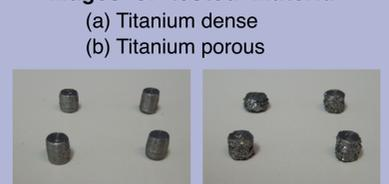
For resulting strength data, see figures in Micromechanics Box.
