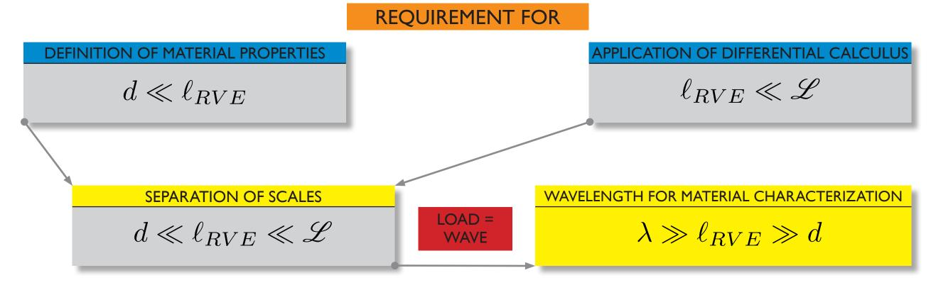
$d \dots$  inhomogeneity [mm]  $\ell_{RVE} \dots$  characteristic length of RVE [mm]
