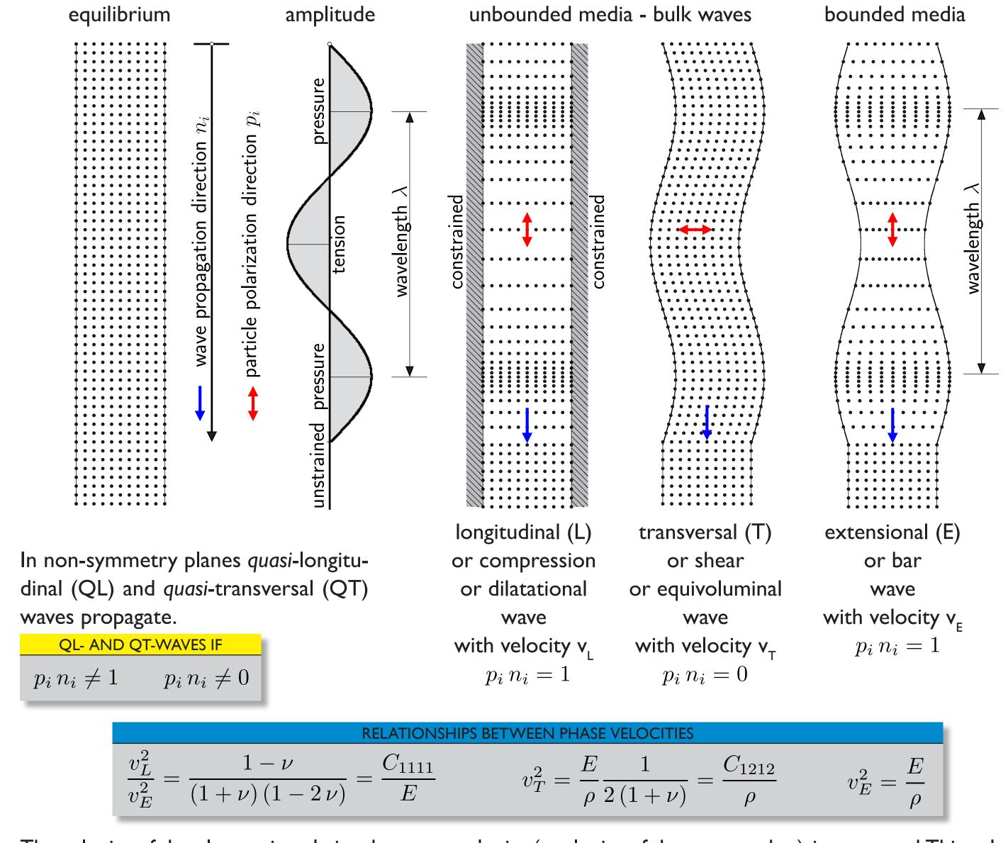
The velocity of the ultrasonic puls, i.e. the group velocity (=velocity of the wave packet), is measured. This velocity is only equal to the phase velocity in isotropic materials and in symmetry planes of anisotropic materials.
