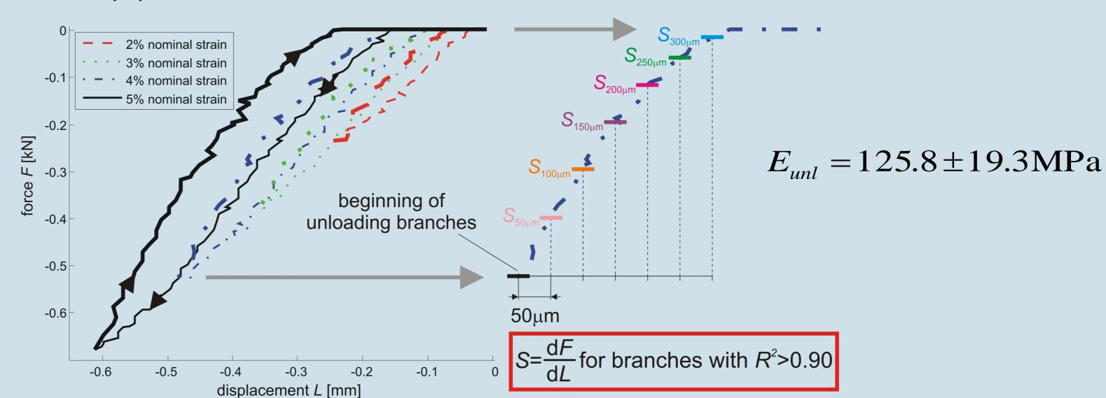
FE simulations and unloading tests deliver consistent values for Young's modulus
