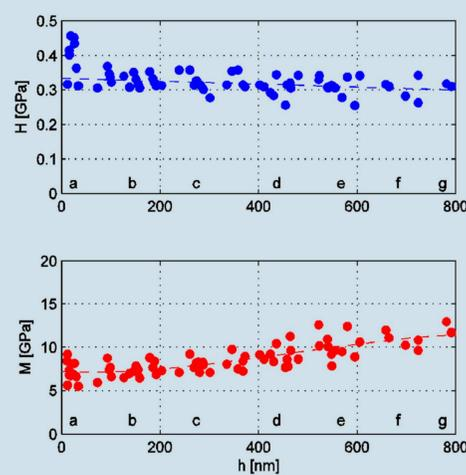
H in CCML showed a slight overall decrease, which did not become significant ( $p > 0.01$ ). M remained at the same level until indentation depths  $h$  of ~250-300 nm and then showed an increase with higher indentation depths. Consequently, suitable indentation depths would lie in the range of 150-180 nm.
