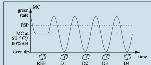
Four cubes were subjected to repeated wetting and drying cycles resulting in a series of 1 to 4 cycles (D1 to D4) next to the untreated reference (REF).
