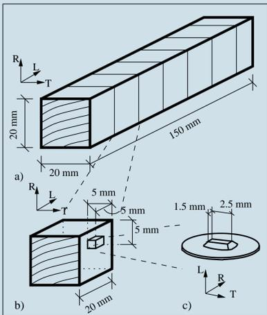
A piece of Norway spruce (*Picea abies* [L] Karst.) wood (a) was cut in five cubes (b). After four of these cubes faced further processing, specimens for nano-indentation were pre-prepared (c) from all five cubes.
