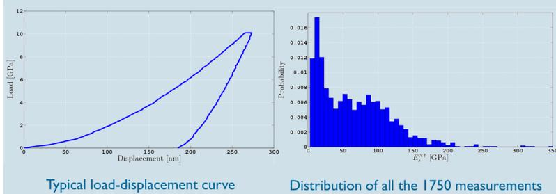
The nanoindentation tests were performed with a Berkovich tip with a loading- unloading rate of 30 mN/min, a holding time of 10 s, and four different maximum loads: 10, 15, 20 and 30 mN. The 1750 measurements were evaluated according to the method of Oliver and Pharr [3].
