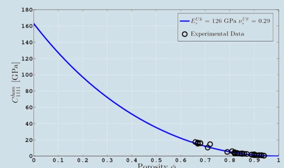
The minimization of the mean absolute error between the model-predicted and the experimentally determined stiffness delivered the elastic properties of pure (dense) baghdadite:  $E_s = 126 \text{ GPa}$  and  $\nu_s = 0.29$ .
