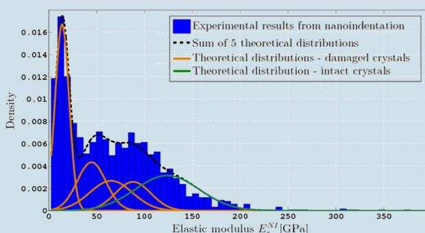
The 1750 nanoindentation results were optimally represented by the superposition of five Gaussian distributions: four corresponding to damaged or broken crystals, and the fifth corresponding to intact crystals. The mean value of the latter is  $\bar{E}_s^{NI} = 124 \text{ GPa}$ , which agrees almost perfectly with  $E_s = 126 \text{ GPa}$  obtained from the micromechanical evaluation of the ultrasonic tests.
