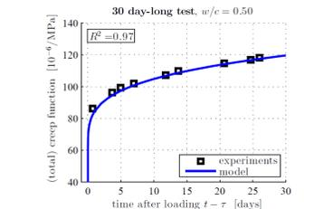
30 days-long tests on 30 years-old paste ( $\rightarrow$ nonaging) from Tamtsia and Beaudin [11] corroborate the micromechanics model
