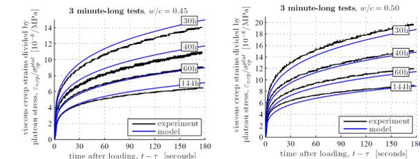
3 min-long tests on young paste are used for identification of hydrate creep properties, optimization routine yields Power-law constants:  $\mu_{c,hyd} = 20.7$  GPa,  $\beta_{hyd} = 0.25$ , model predictions nicely capture the aging-induced reduction of creep activity
