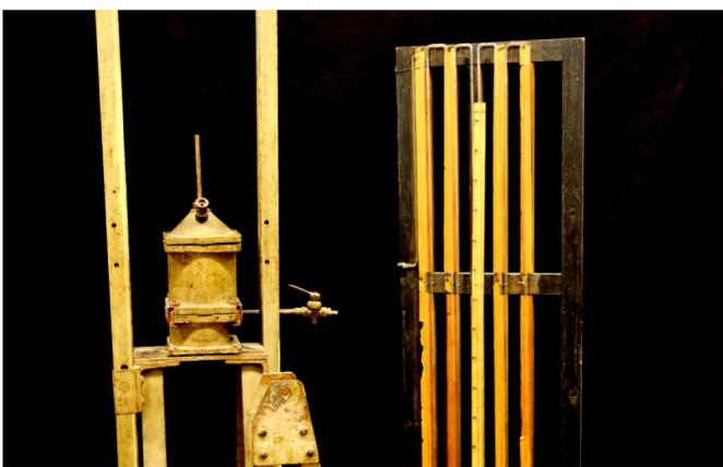
Triaxial compression test apparatus, combined with pore water pressure measuring equipment, 1937.
