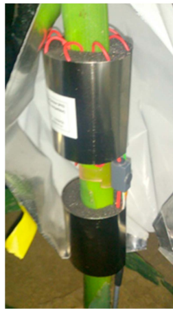
Figure 2. Example of sap flow system EMS 62, consisting of a heating element installed in the upper section (red wires) and two insulated thermocouples inserted 15 cm apart.
