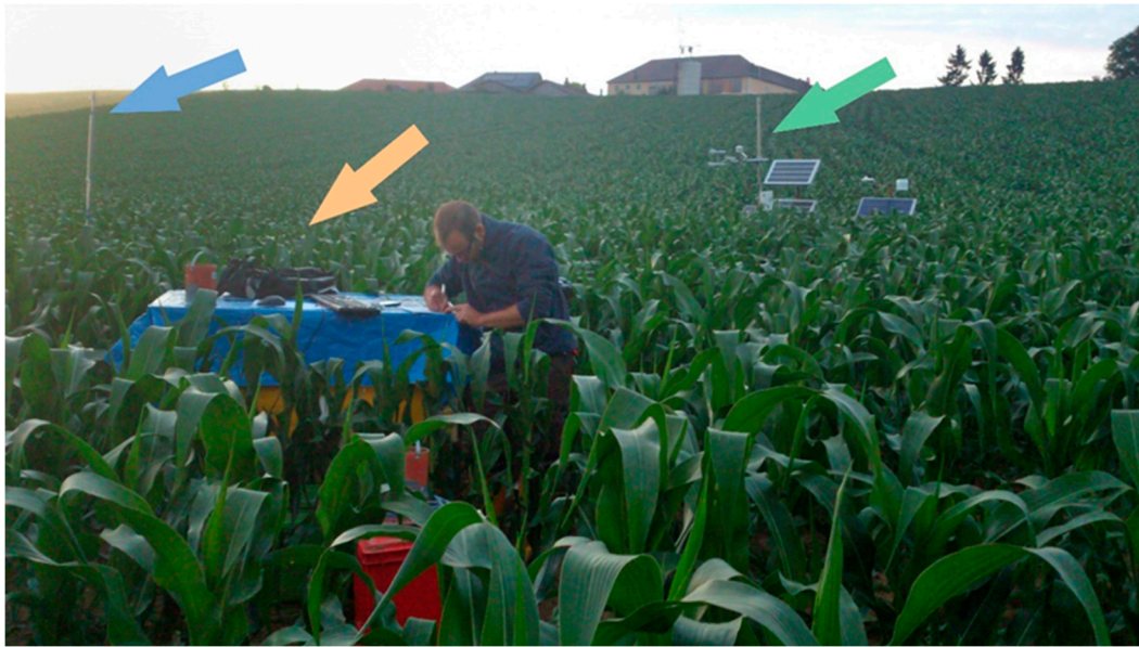
Figure 1. Experimental setup for the field campaign, showing the location of the measurement profile pole (blue arrow), the Picarro isotope analyzer (orange arrow, under blue tarp), and the eddy covariance station (green arrow).
