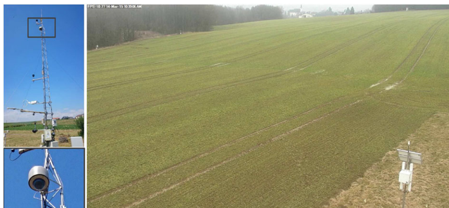
FIGURE 2 On-site camera set-up. Left: Installation on the weather station mast. Right: Camera view
