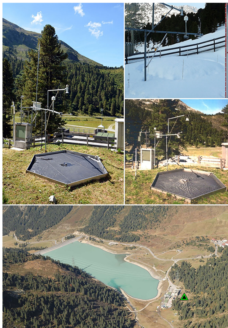
Figure 1. Kühtai snow monitoring station. (top left) September 2016; (top right) March 2015 when snow water equivalent was 345 mm; (middle right) September 1990. A comparison of photos shows that the station setup remained almost unchanged in the period 1990–2015. (bottom) Setting of the station. The triangle indicates location of the station.
