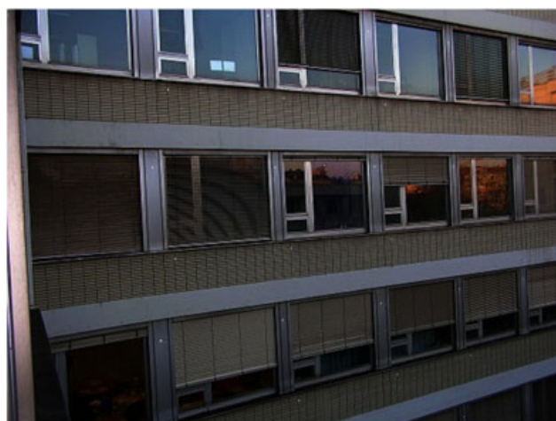
Figure 4. Part of the calibration test field with retro-reflecting targets mounted on the wall of the I.P.F building of the Vienna University of Technology
