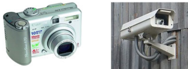
Figure 3. Camera CANON Powershot A70 camera (left) and its implementation inside the outdoor case (right)
