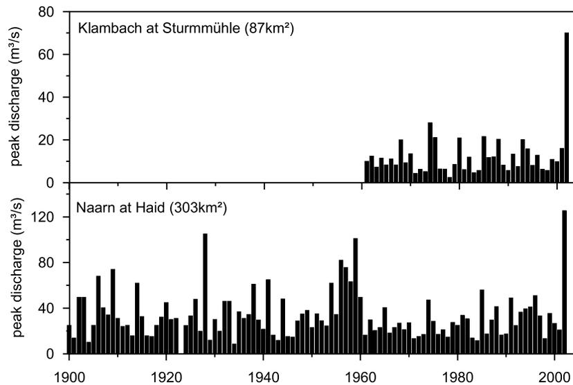
**Figure 1.** Time series of observed maximum annual peak discharges of (top) Klambach at Sturmmühle (87 km<sup>2</sup> catchment area) and (bottom) Naarn at Haid (303 km<sup>2</sup> catchment area).
