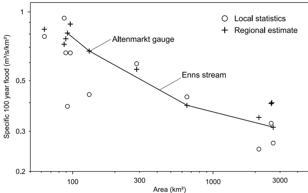
**Figure 4.** Discharge-area diagram of the upper Enns valley. Specific 100-year flood discharges derived from locally observed data are shown as open circles. Regional estimates using flood data from neighboring stations are shown as plusses.
