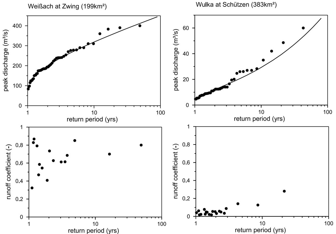
**Figure 9.** (top) Flood frequency plots and (bottom) runoff coefficients of the associated flood events for (left) Weißbach at Zwing (199 km<sup>2</sup> catchment area) and (right) Wulka at Schützen (383 km<sup>2</sup> catchment area).
