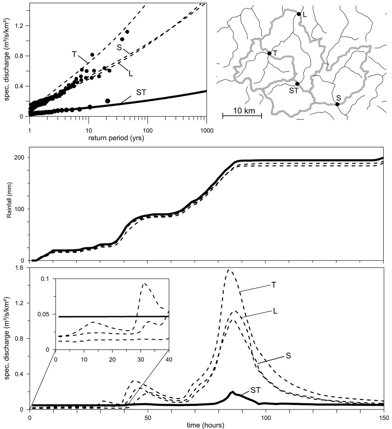
**Figure 6.** Flood frequency plots of (top left) the Unrechtstraisen at St. Aegydt (ST) (54 km<sup>2</sup> catchment area) and (top right) neighboring catchments (Traisen at Türnitz (T) (103 km<sup>2</sup> catchment area), Traisen at Lilienfeld (L) (333 km<sup>2</sup> catchment area), and Schwarzau at Schwarzau (S) (128 km<sup>2</sup> catchment area)). (middle) Hyetographs and (bottom) hydrographs of the flood event 4 July 1997 to 10 July 1997.
