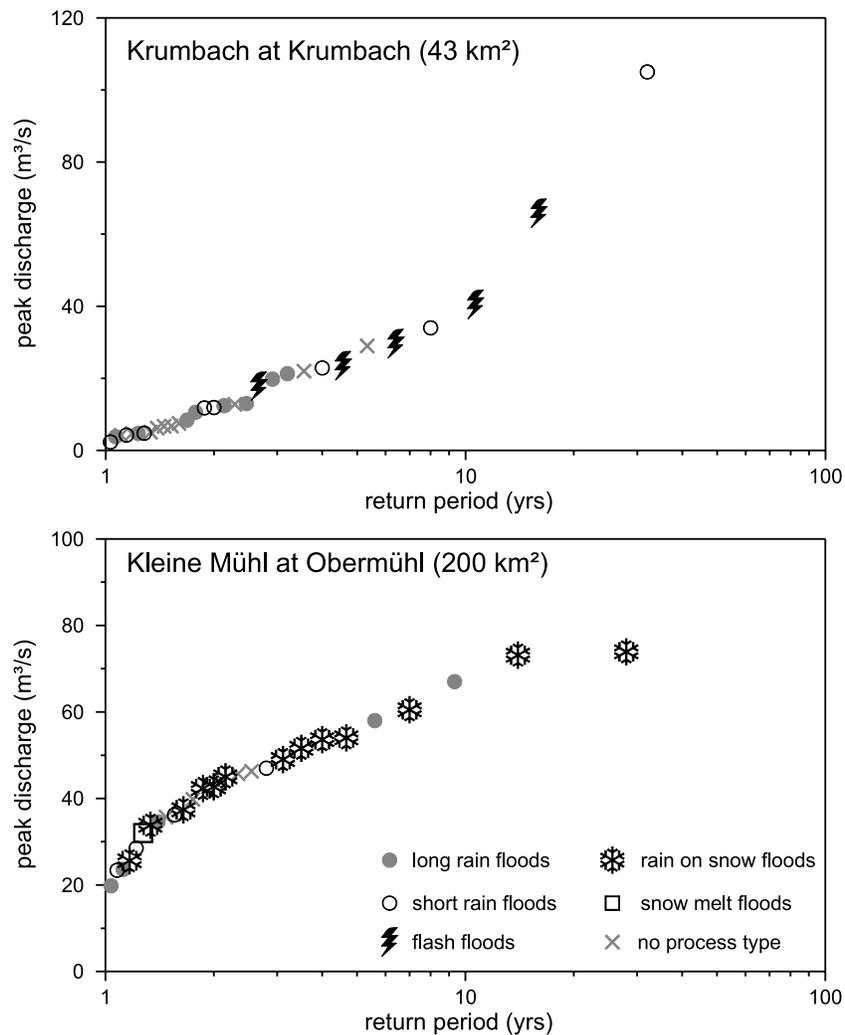
**Figure 10.** Flood frequency plots with the process types indicated. (top) Krumbach at Krumbach (43 km<sup>2</sup> catchment area). (bottom) Kleine Mühl at Obermühl (200 km<sup>2</sup> catchment area).
