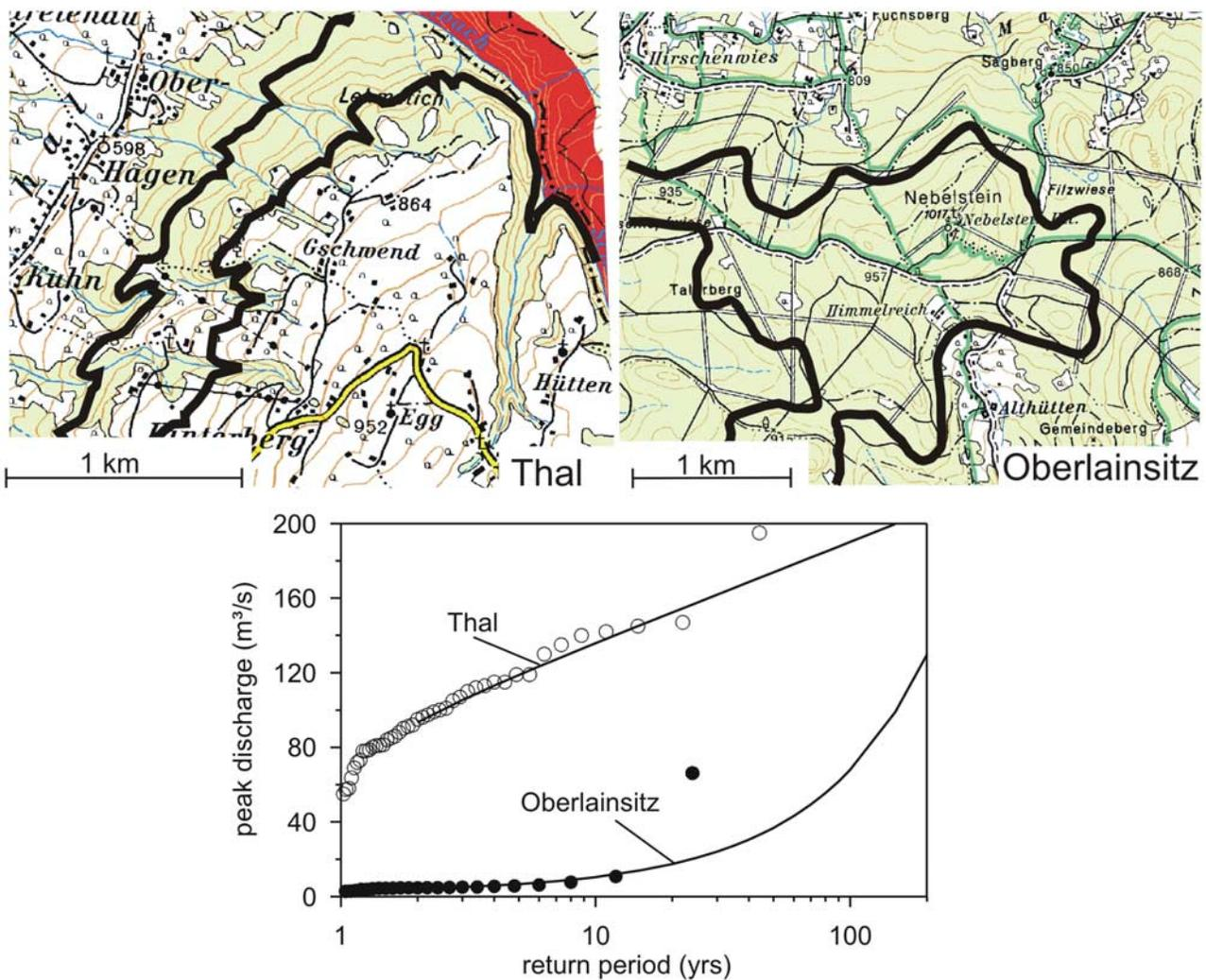
**Figure 11.** (top) Topographic maps of representative landforms of (left) the Rotach at Thal (90 km<sup>2</sup> catchment area) and (right) the Lainsitz at Oberlainsitz (81 km<sup>2</sup> catchment area) catchments. Two contour lines are marked as thick black lines to demonstrate the degree of incision of the streams. (bottom) Flood frequency plots of observed flood data in the two catchments.
