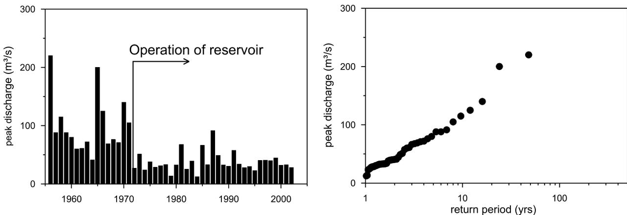
**Figure 3.** (left) Time series of observed maximum annual peak discharges of the Zemmbach at Sausteinaste (225 km<sup>2</sup> catchment area). The upstream Schlegeis reservoir was built in 1972. (right) Flood frequency plots of the Zemmbach at Sausteinaste.
