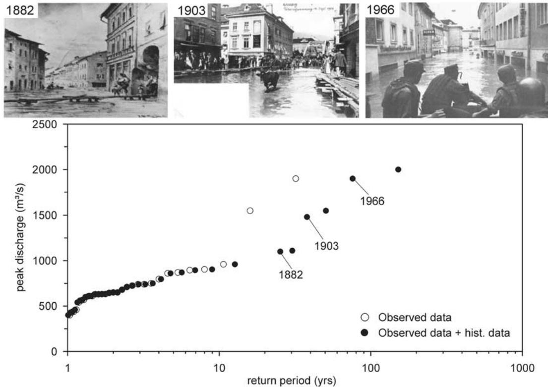
**Figure 2.** (top) Painting and photographs of historical (1882 and 1903) and observed flood (1966) water stages at the Lederer Gasse near the Drau cross section at Villach. (bottom) Flood frequency plot of the Drau at Villach based on observed flood data (open circles) alone and observed and historical flood data (black circles) derived from flood marks and photographs.
