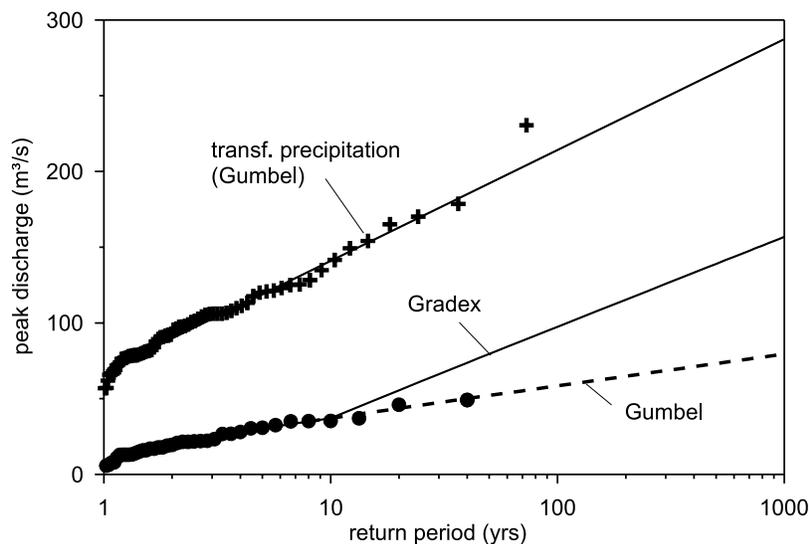
**Figure 8.** Gradex method for the Trisanna at Galtür (97 km<sup>2</sup> catchment area). Transformed precipitation data of the station Partennen are shown as pluses.
