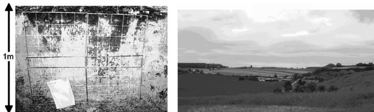
Figure 3. Dye flow patterns observed at the Weiherbach irrigation site and view of the Weiherbach catchment.
