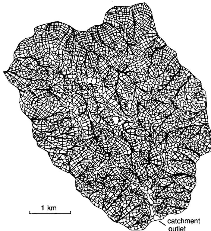
Figure 1. Element network for the Coweeta topography, North Carolina, USA. The elements are defined by adjacent flow paths and contours
