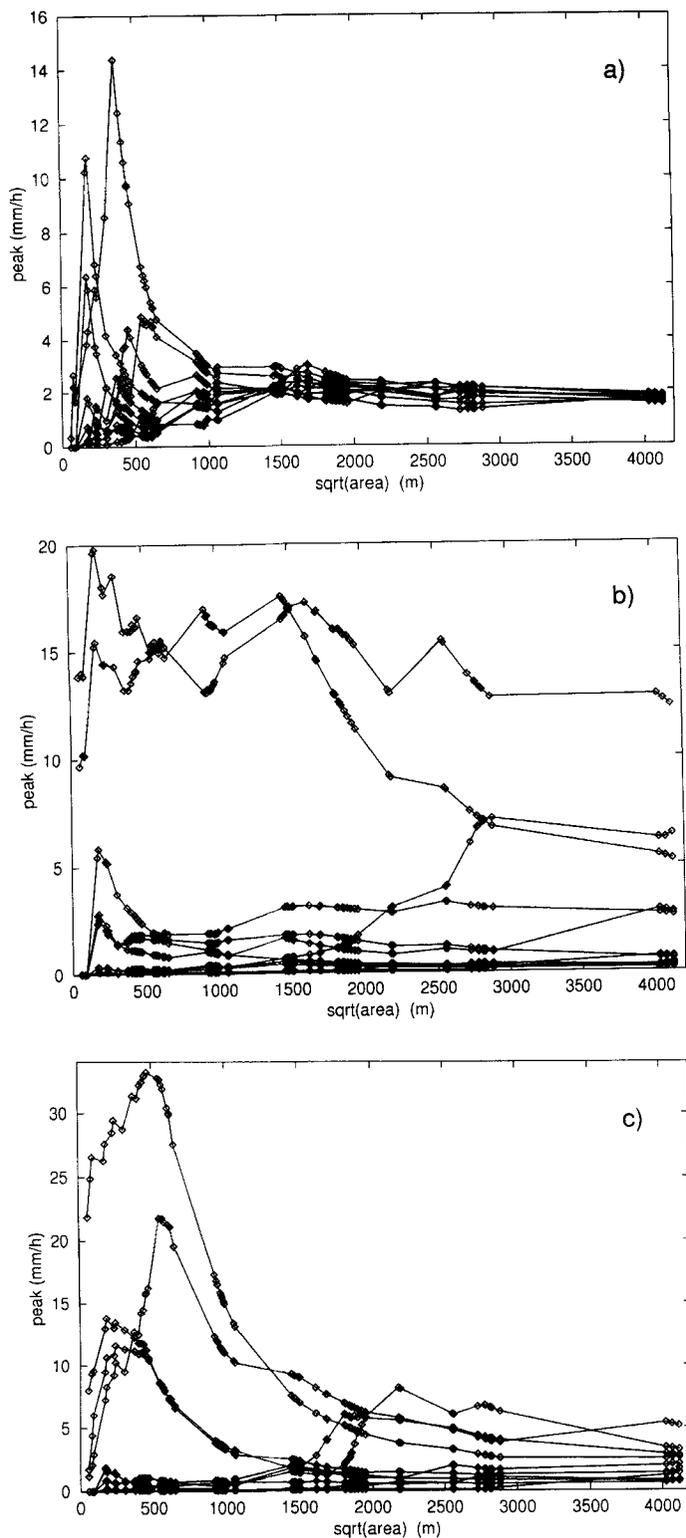
Figure 10. Peak flow versus subcatchment area for the set of nested catchments shown in Figure 3. Infiltration characteristics and channels as in Figure 9. Ten realizations of spatially variable precipitation of one hour duration with correlation lengths of (a) 125 m; (b) 2500 m; and (c) 625 m
