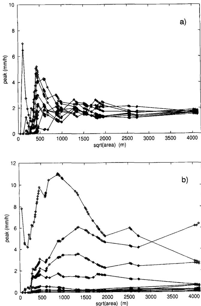
Figure 11. As Figure 10 for another set of nested catchments. Correlation length of precipitation is (a) 125 m; and (b) 2500 m. The highest intensity realization is not shown in (b)
