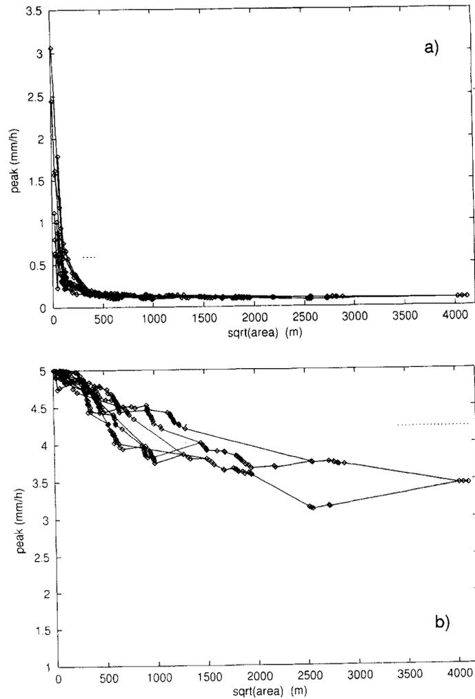
Figure 6. Peak flow versus subcatchment area for 10 sets of nested catchments. Impervious conditions, no channels, Manning's  $n=0.4$ . (a) 12 minute rainblock; and (b) two hour rainblock. Precipitation is spatially invariant
