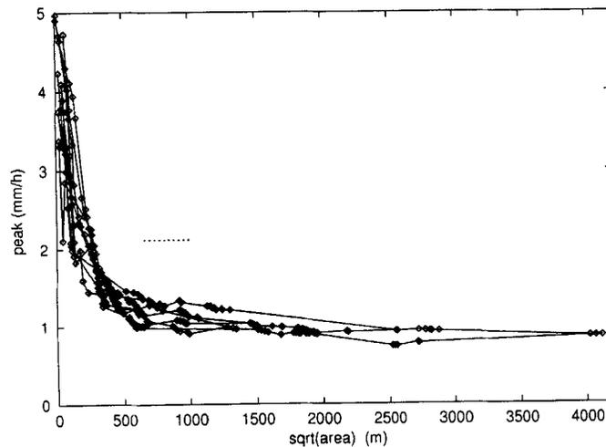
Figure 7. Peak flow versus subcatchment area for 10 sets of nested catchments. Impervious conditions, no channels, 12 minutes rain-block, Manning's  $n=0.04$ . Precipitation is spatially invariant (same as Figure 6a, but lower roughness)
