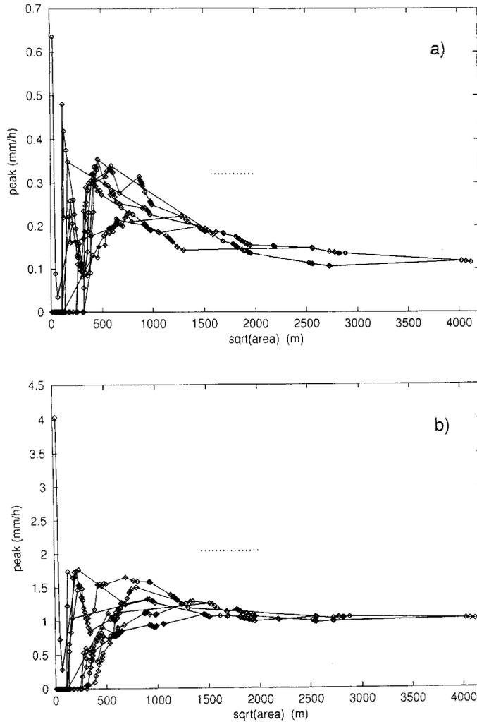
Figure 9. Peak flow versus subcatchment area for 10 sets of nested catchments. Infiltration allowed, 30% initial saturated area, Manning's  $n=0.4$ , channelized flow for upslope contributing areas  $> 10$  ha. (a) 12 minute rainblock; and (b) one hour rainblock. Precipitation is spatially invariant and soils are spatially variable
