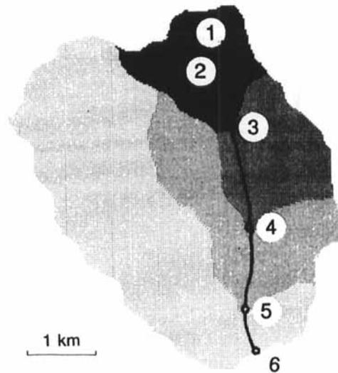
Figure 3. Example of a set of nested catchments. Numbers indicate some of the subcatchment outlets and refer to those in Figure 4.
