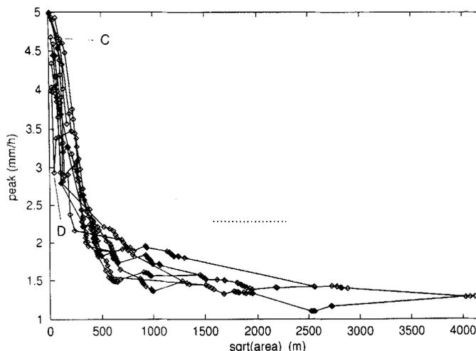
Figure 5. Peak flow versus subcatchment area for 10 sets of nested catchments. Impervious conditions, no channels, Manning's  $n=0.4$ , one hour rainblock. Precipitation is spatially invariant. The dotted line suggests the approximate size of the REA. C refers to a convergent element and D refers to a divergent element
