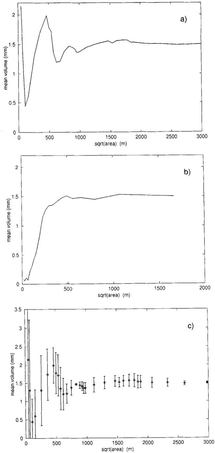
Figure 2. Mean runoff volume versus catchment size for spatially variable soils and constant precipitation. (a) Filtering based on a window of 15 subcatchments moving in steps of five, resulting in 30 classes as in Figure 4a of Wood *et al.* (1988). (b) Filtering based on a window of 135 subcatchments moving in steps of 45, resulting in 30 classes. (c) Standard deviations within windows for (a)
