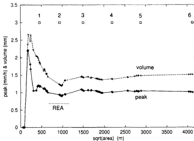
Figure 4. Runoff volume and peak versus subcatchment size for one set of nested catchments as shown in Figure 3. Spatially variable soils and constant precipitation
