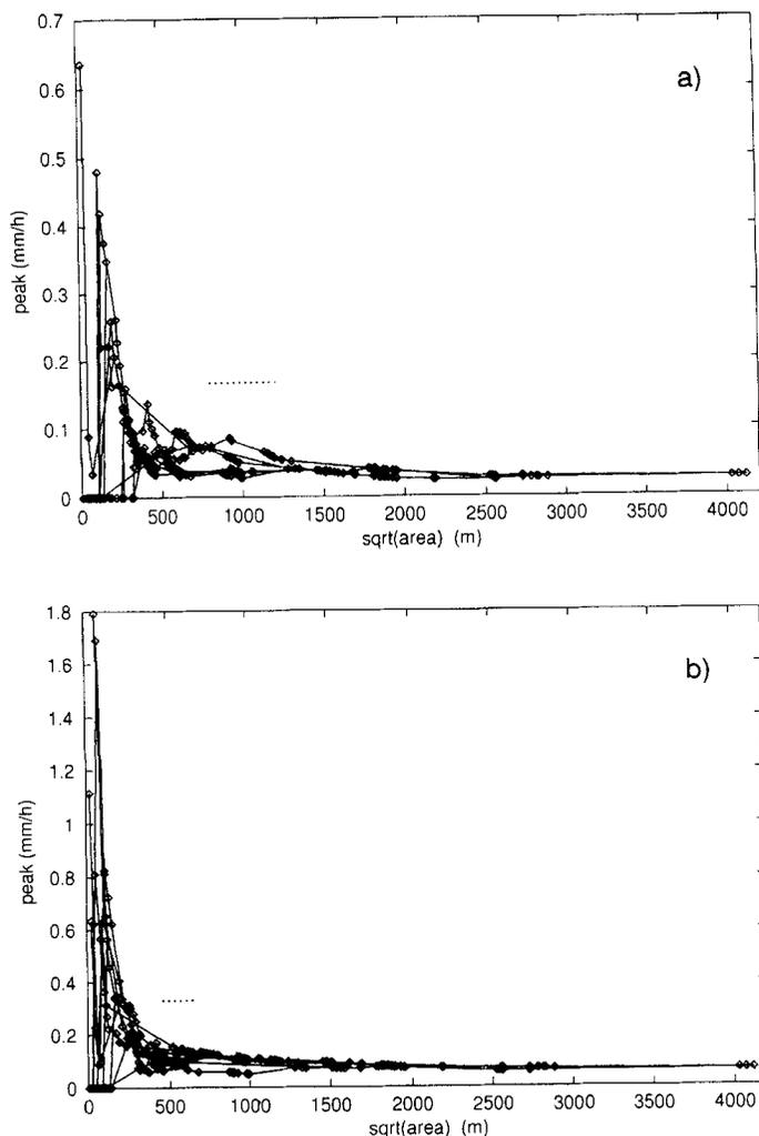
Figure 8. Peak flow versus subcatchment area for 10 sets of nested catchments. Infiltration allowed, no channels, 12 minute rainblock, Manning's  $n = 0.4$ . (a) Initial saturated area is 30%. (b) Initial saturated area is 70%. Precipitation is spatially invariant and soils are spatially variable
