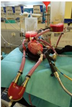
Figure 1 Left: Isolated large animal heart connected to an in-vitro circuit mimicking the human cardiovascular system. Right: A schematic diagram of the proposed HIL system to evaluate the interaction between the VAD and simulated heart failure patients.
