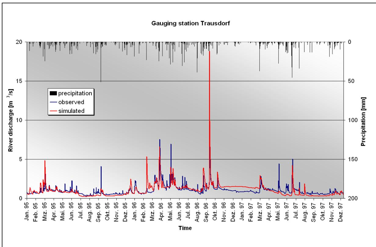
Fig. 5-10: Comparison of the observed and simulated hydrograph of the gauging station Trausdorf (1995-1997)
