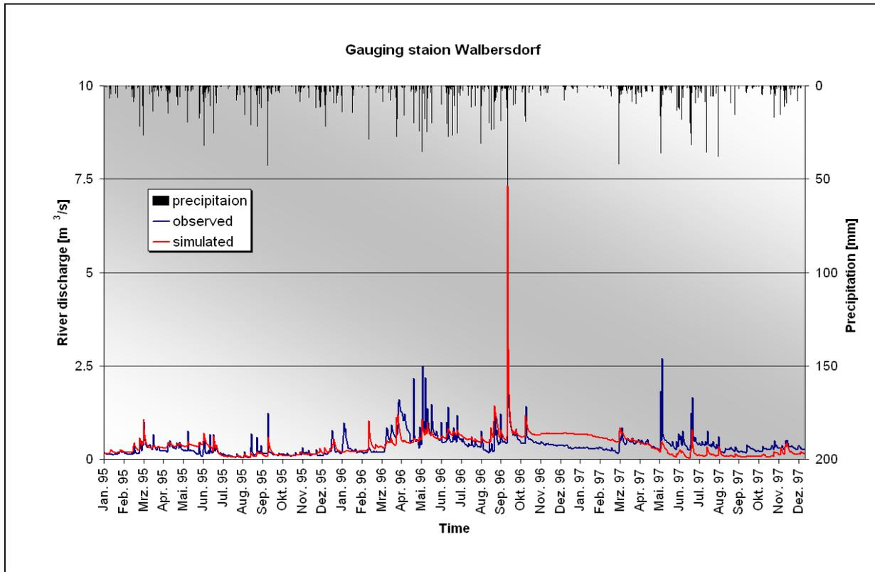
**Fig. 5-8: Comparison of the observed and simulated hydrograph of the gauging station Walbersdorf (1995-1997)**
