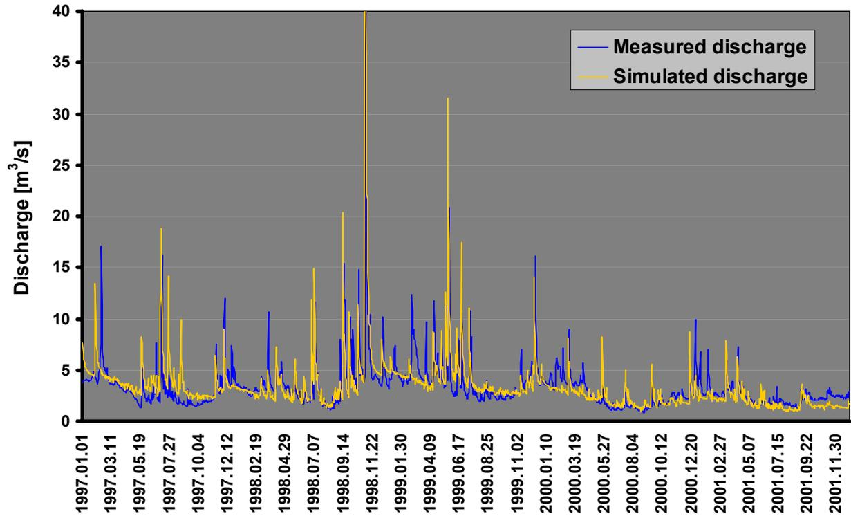
Fig. 6-26: Simulated and measured discharges at Zalabér station
