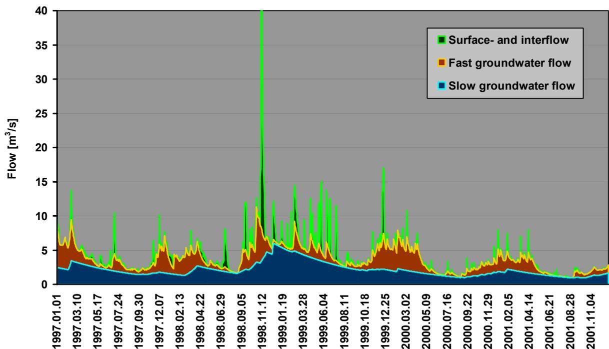
Fig. 6-33: Separated runoff hydrographs at Zalaapáti station
