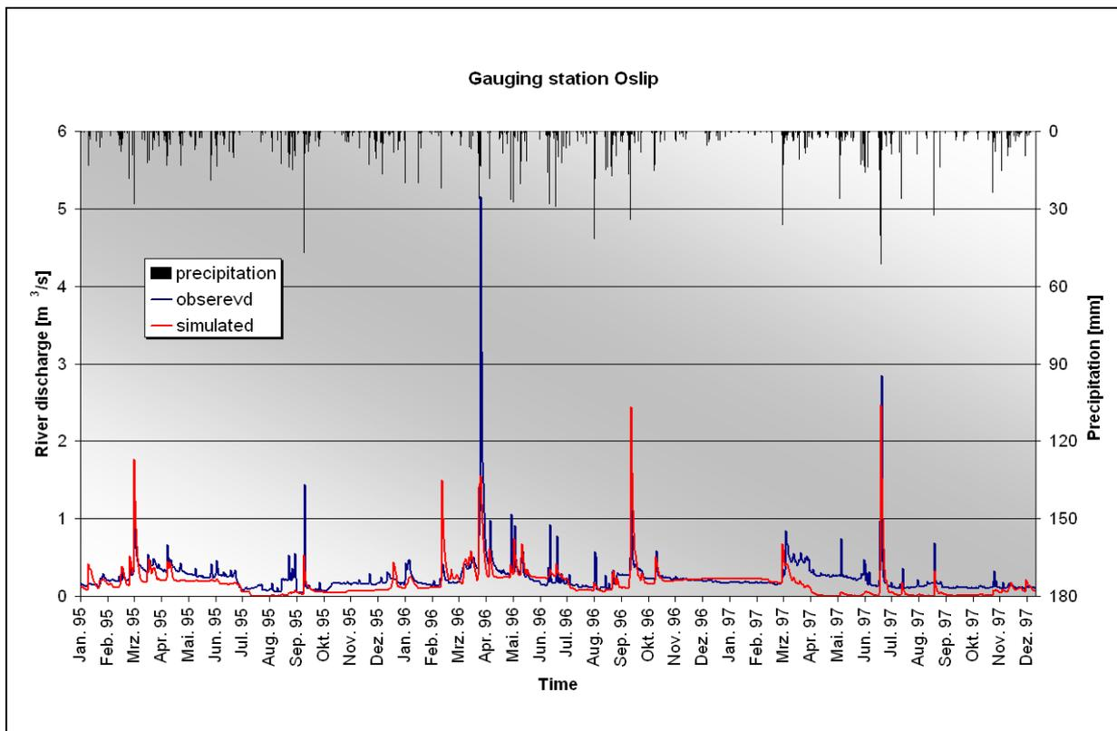
Fig. 5-12: Comparison of the observed and simulated hydrograph of the gauging station Oslip (1995-1997)
