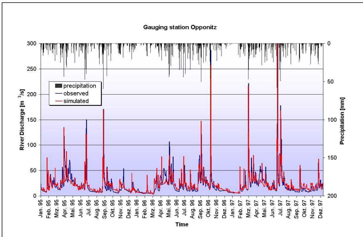
Fig. 5-3: Comparison of the observed and the simulated hydrograph at the gauging station Opponitz (1995-1997)
