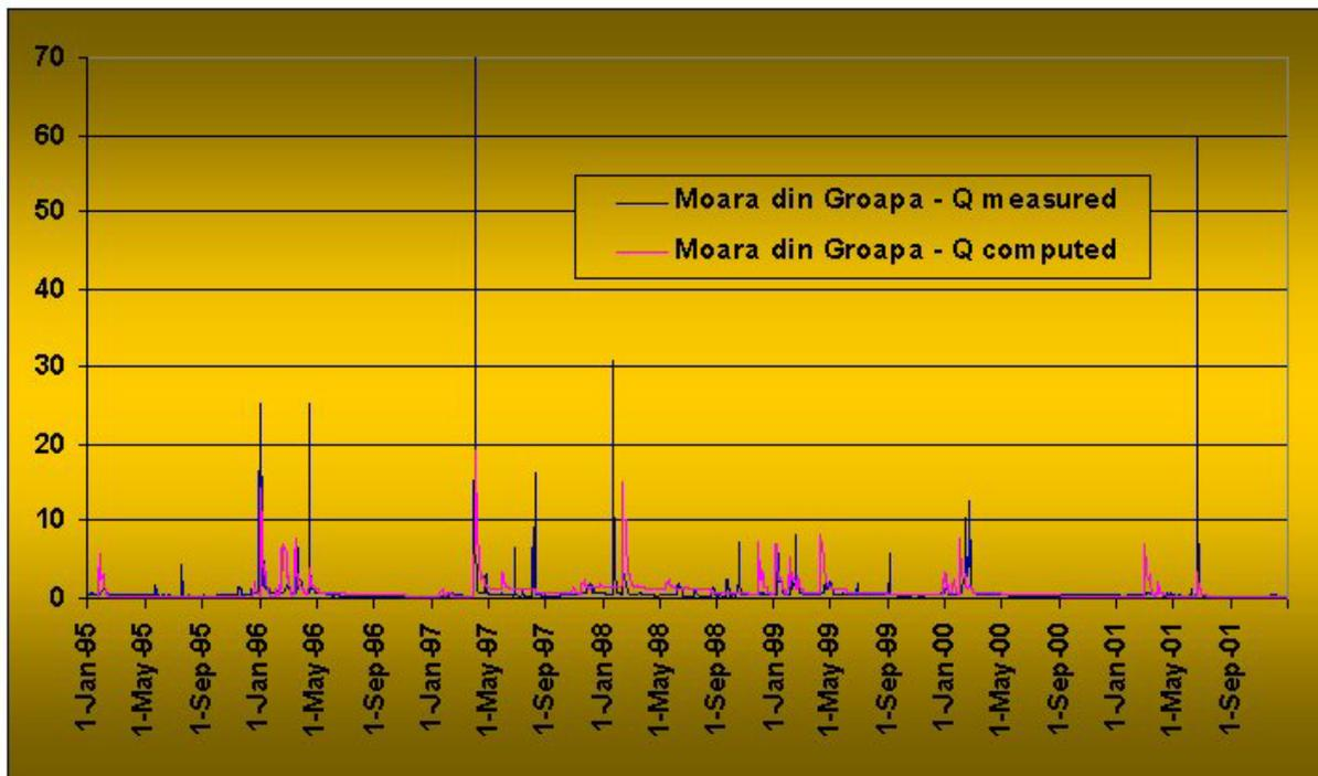
Fig. 5-20: Comparison between measured, uncalibrated and calibrated river discharge values at the Moara din Groapa station
