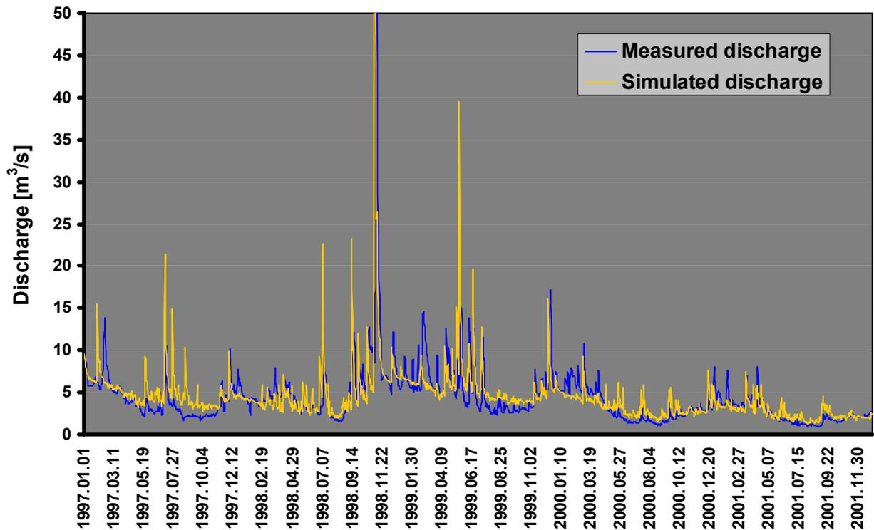
Fig. 6-27: Simulated and measured discharges at Zalaapáti station (watershed outlet)
