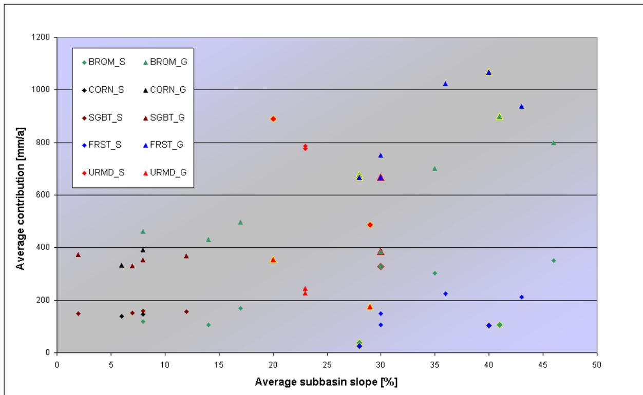
**Fig. 6-1: Average annual contribution of the HRU's in dependence of the subbasin slope and the soil hydrologic group (group B: yellow border, group C: no border, group D: red border)**
