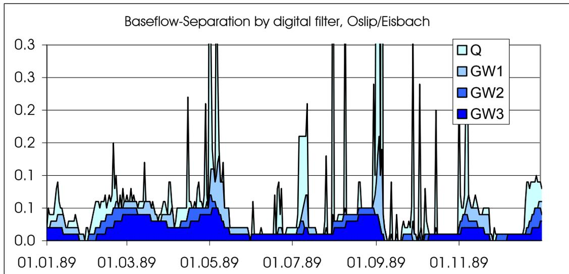
Fig. 6-10: corrected runoff and baseflow-separation in Oslip
