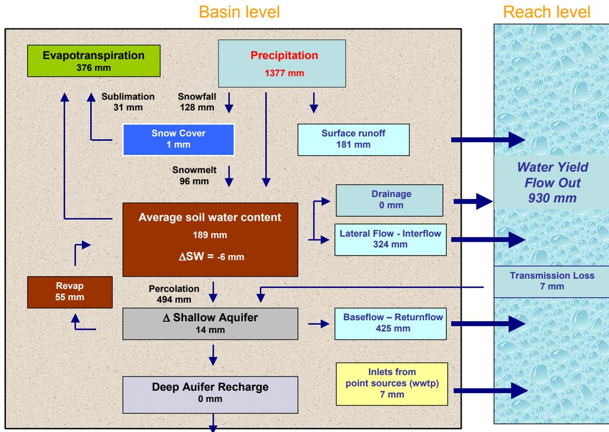
Fig. 6-19: Water cycle scheme for the Ybbs catchment
