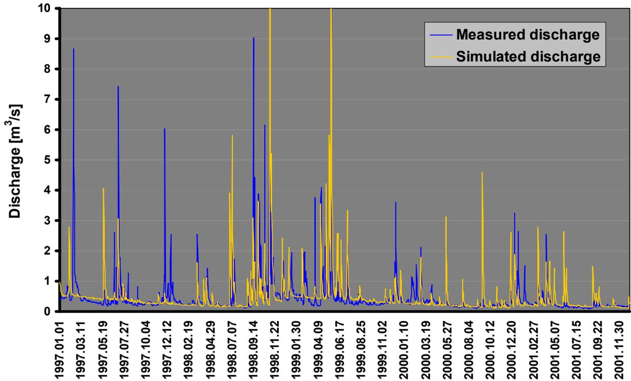
Fig. 6-24: Simulated and measured discharges at Zalalövő station
