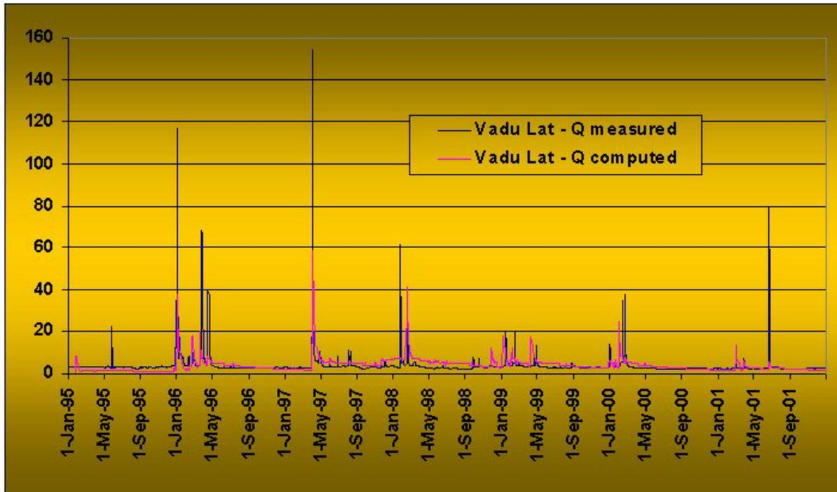
Fig. 5-19: Comparison between measured, uncalibrated and calibrated river discharge values at the Vadu Lat station
