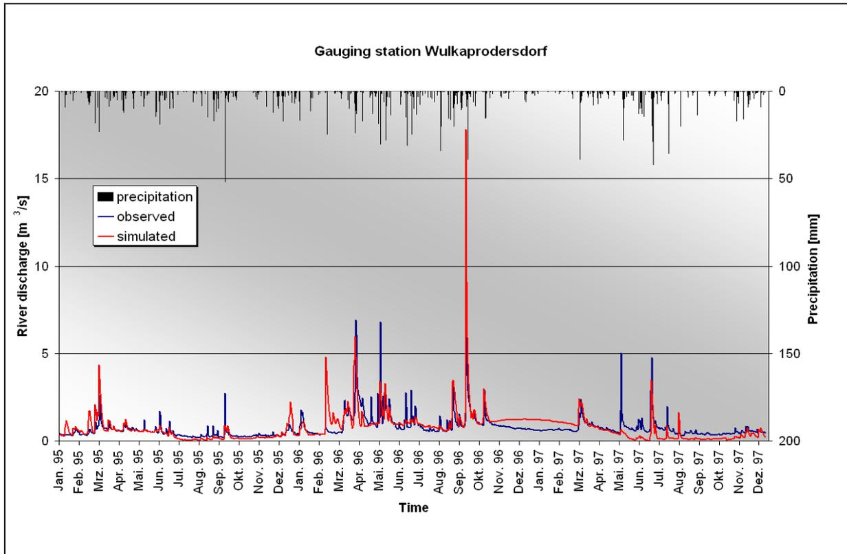
Fig. 5-9: Comparison of the observed and simulated hydrograph of the gauging station Wulkaprodersdorf (1995-1997)
