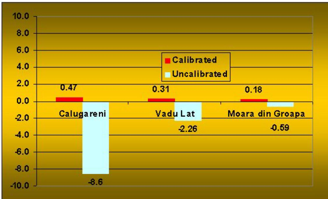
Fig. 5-16: Nash-Sutcliffe coefficient for calibration points (daily basis)
