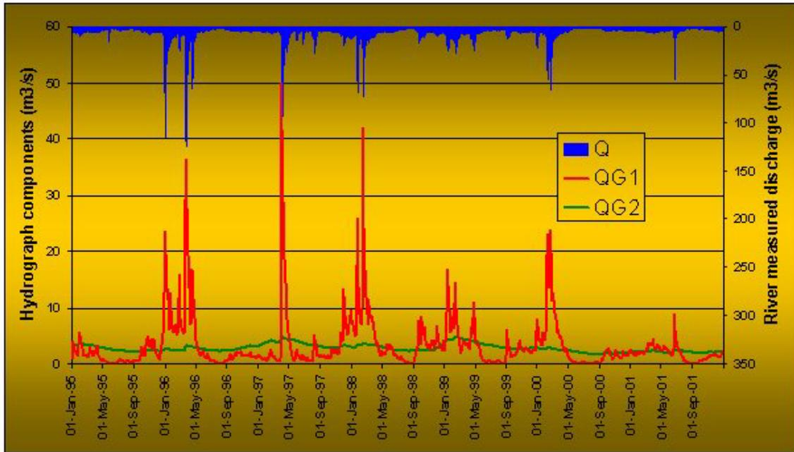
Fig. 6-52: Hydrograph separation for Calugareni station
