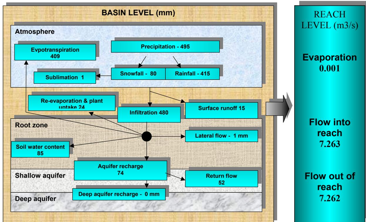
Fig. 6-44: Detailed hydrological cycle for the study case
