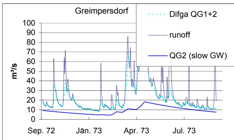
Fig. 6-3: separation of runoff with Difga2000.
