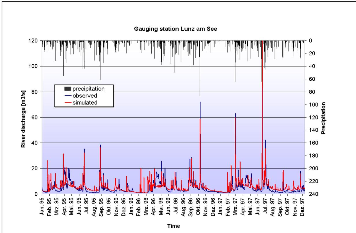
Fig. 5-2: Comparison of the observed and the simulated hydrograph at the gauging station Lunz am See (1995-1997)
