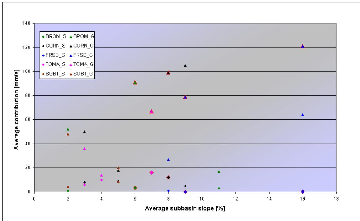
**Fig. 6-2: Average annual contribution of the HRU's in dependence of the subbasin slope and the soil hydrologic group (group A: red border, group B: no border)**
