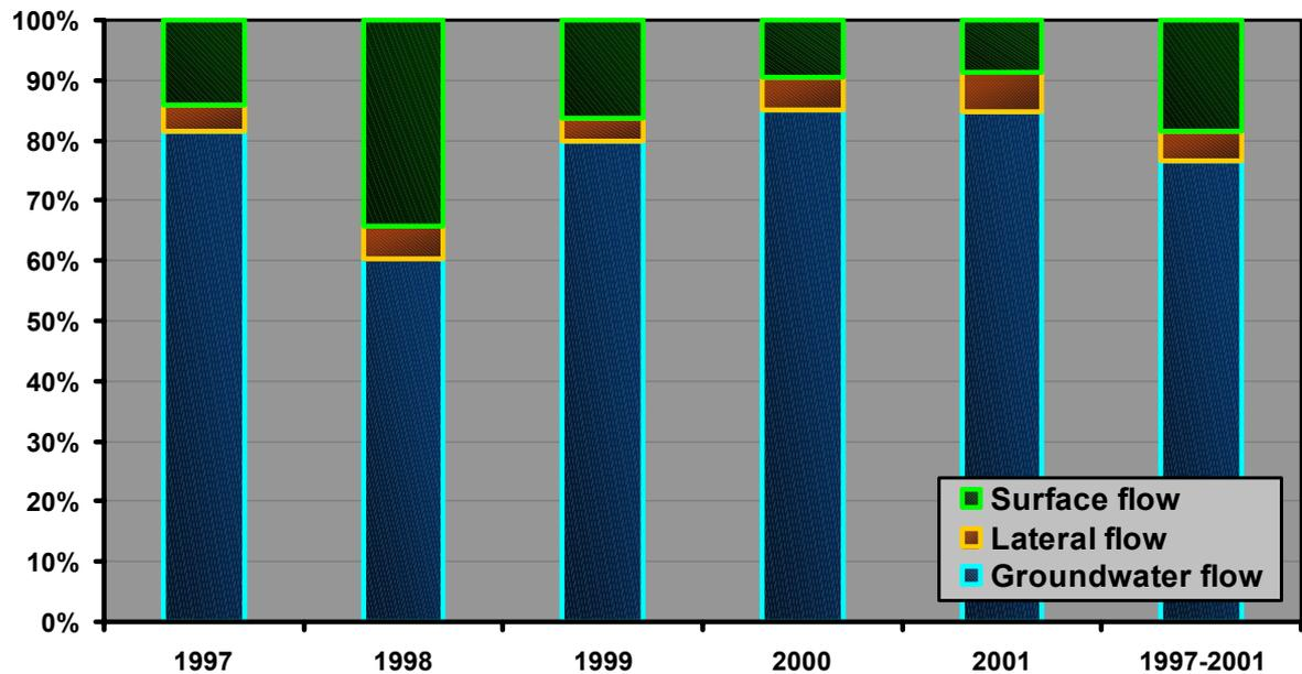
Fig. 6-30: Proportion of the runoff components of the total catchment area
