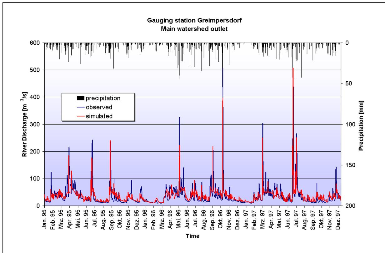
**Fig. 5-6: Comparison of the observed and the simulated hydrograph at the gauging station Greimpersdorf (1995-1997)**
