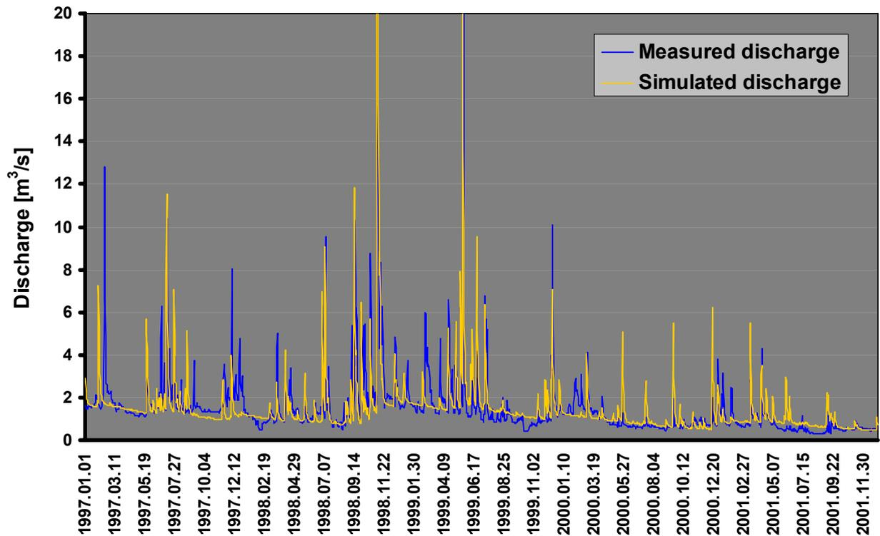
Fig. 6-25: Simulated and measured discharges at Zalaegerszeg station
