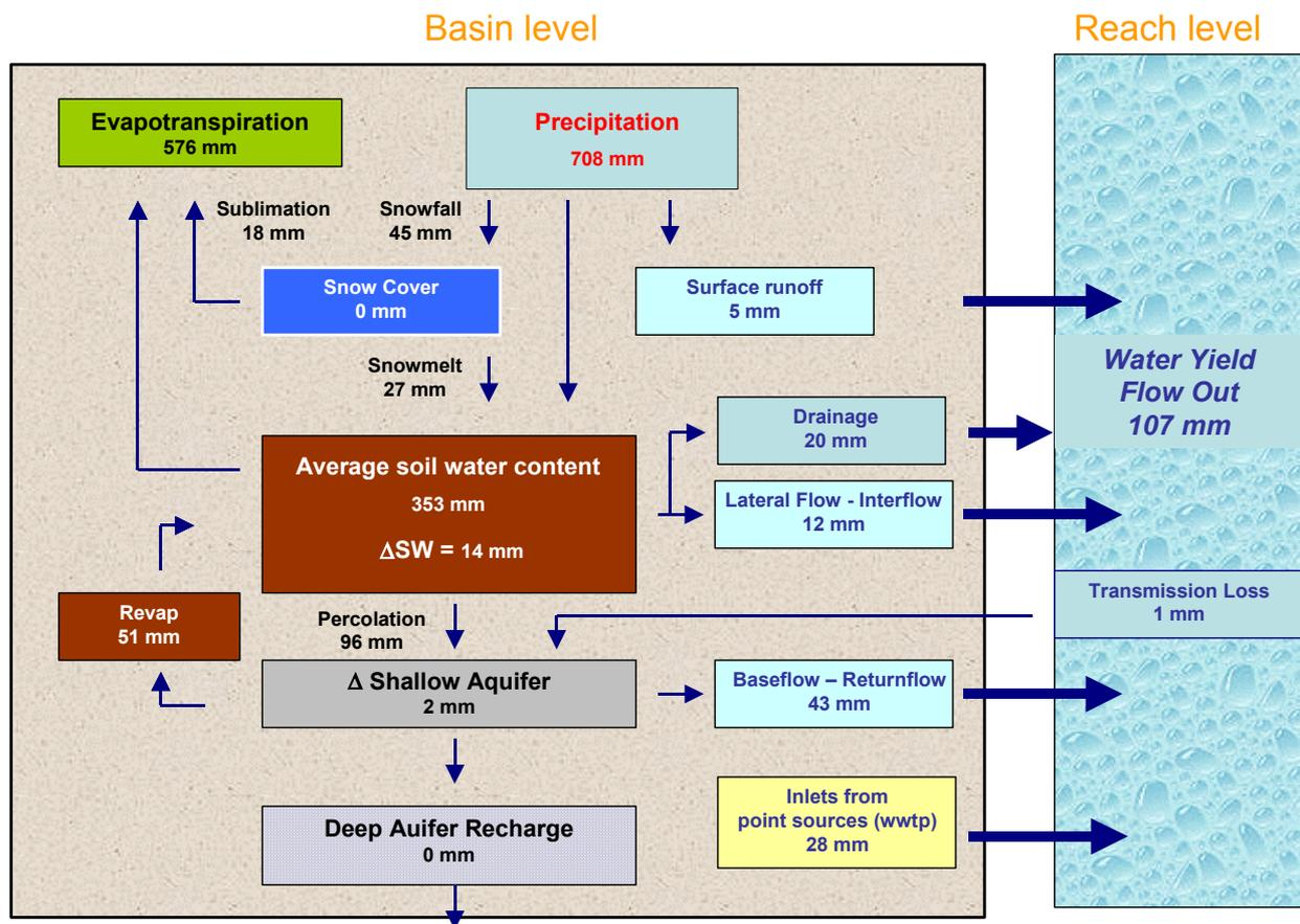
Fig. 6-20: Water cycle scheme of the Wulka catchment
