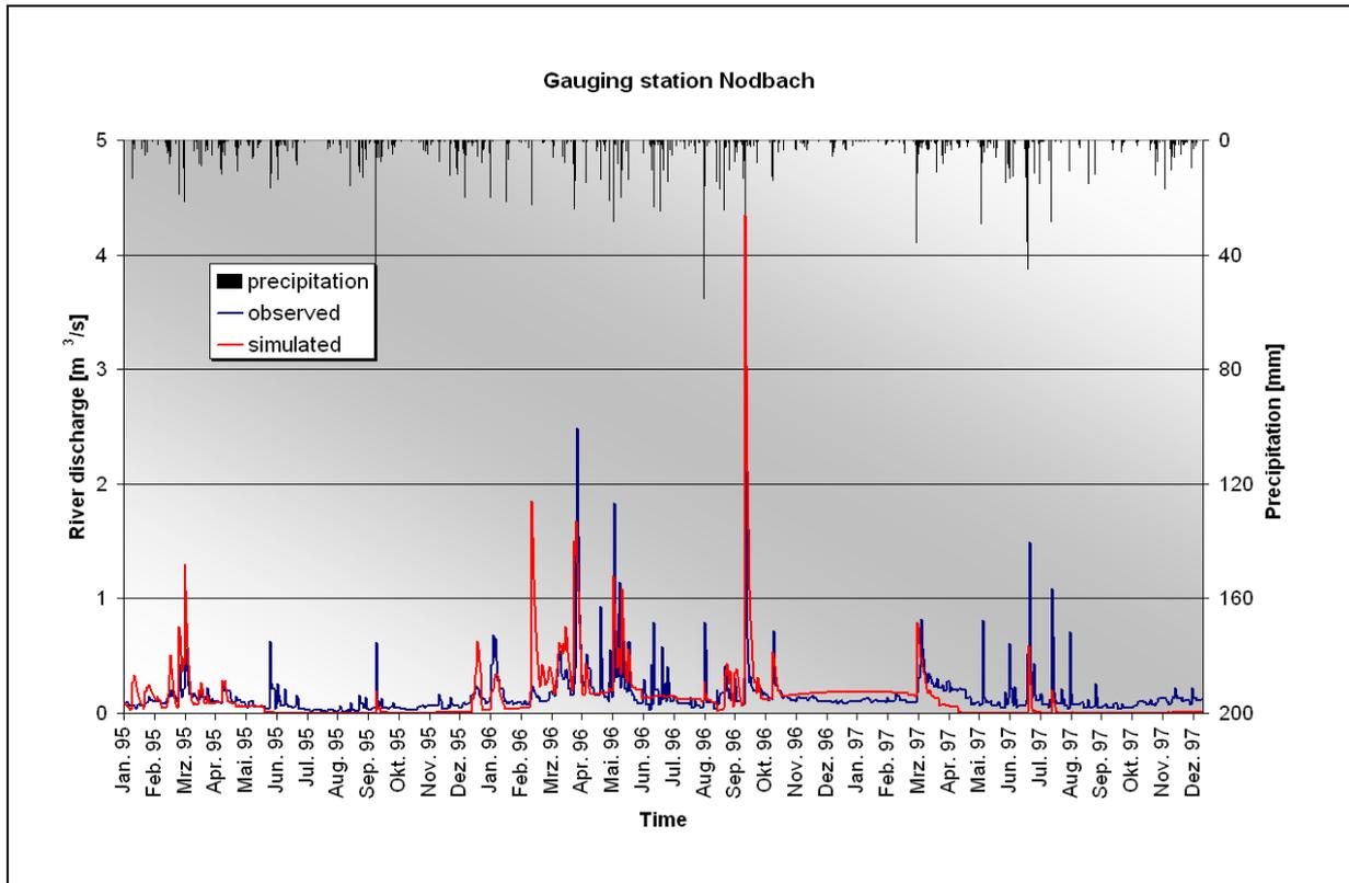
Fig. 5-11: Comparison of the observed and simulated hydrograph of the gauging station Nodbach (1995-1997)
