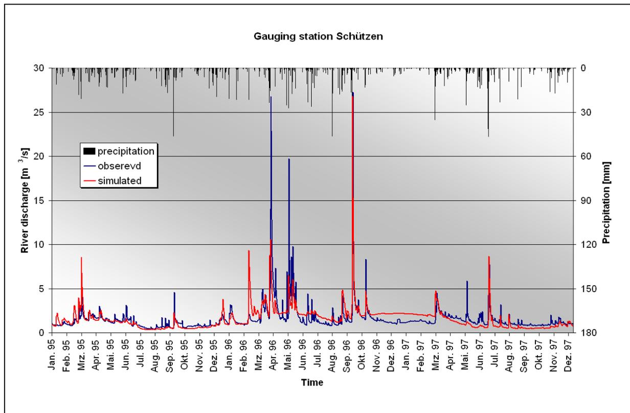
**Fig. 5-13: Comparison of the observed and simulated hydrograph of the gauging station Schützen (1995-1997)**
