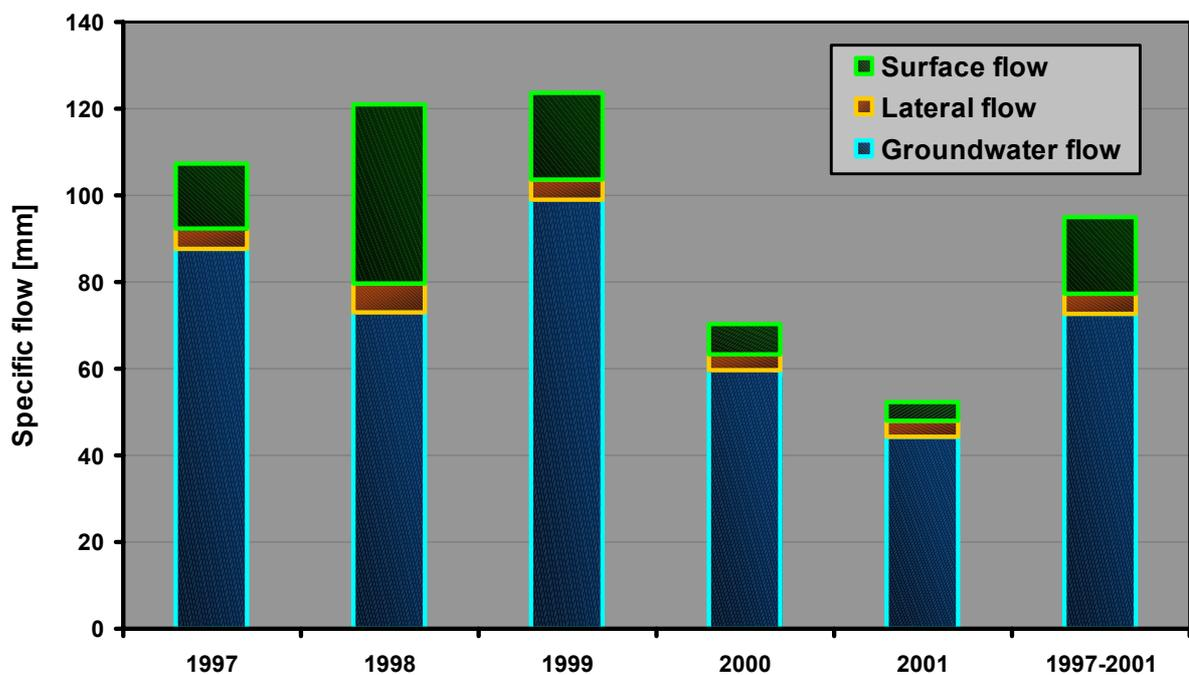
Fig. 6-29: Runoff components of the total catchment area
