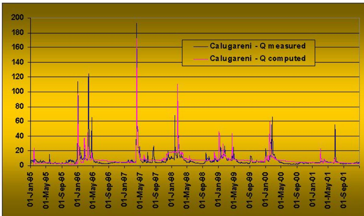
Fig. 5-18: Comparison between measured, uncalibrated and calibrated river discharge values at the Calugareni station
