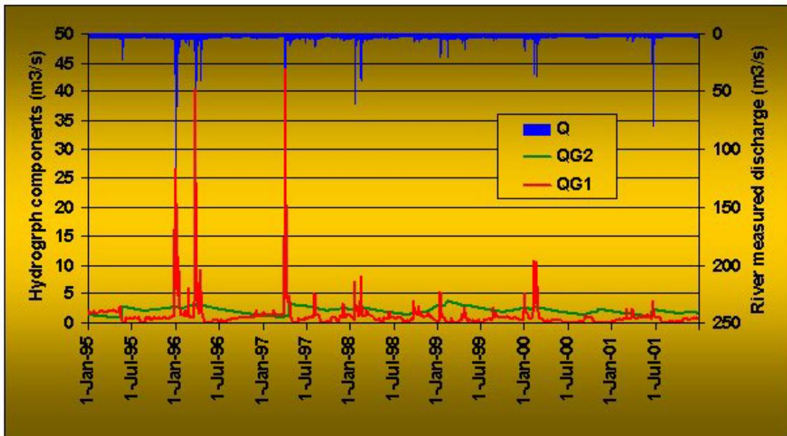
Fig. 6-53: Hydrograph separation for Vadu Lat station
