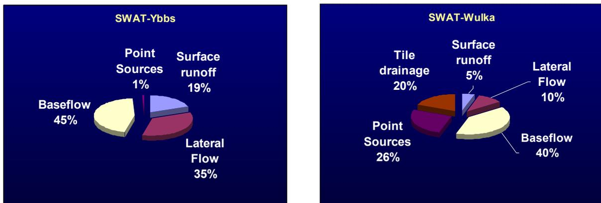
Fig. 6-22: Runoff components calculated by SWAT for the Ybbs catchment (left) and the Wulka catchment (right)
