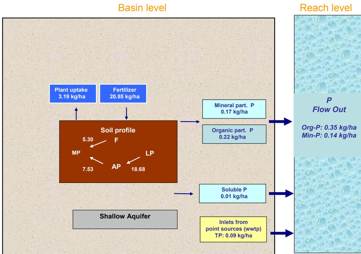
**Figure 7-2:** Phosphorus balance for the Wulka catchment calculated with the SWAT 2000 model (average values for the calculation period 1992 – 1999)
