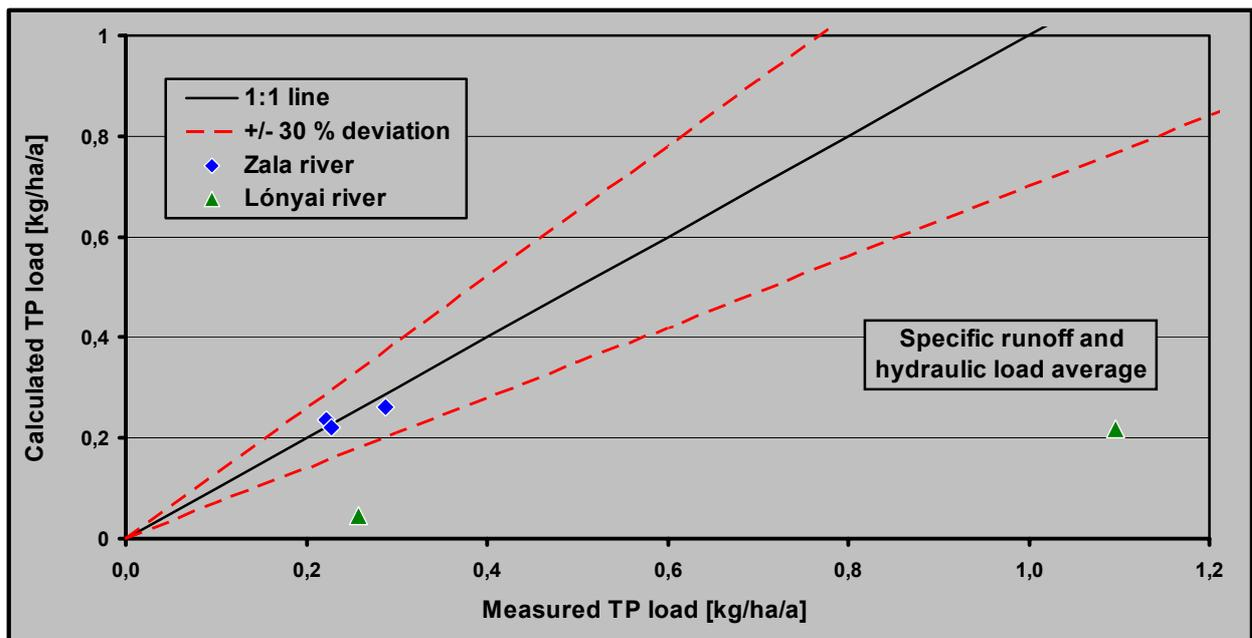
Figure 65: Comparison of measured and modeled TP load calculated based on the modified MONERIS model in dependence on specific runoff and hydraulic load (for the period 1997-2001)
