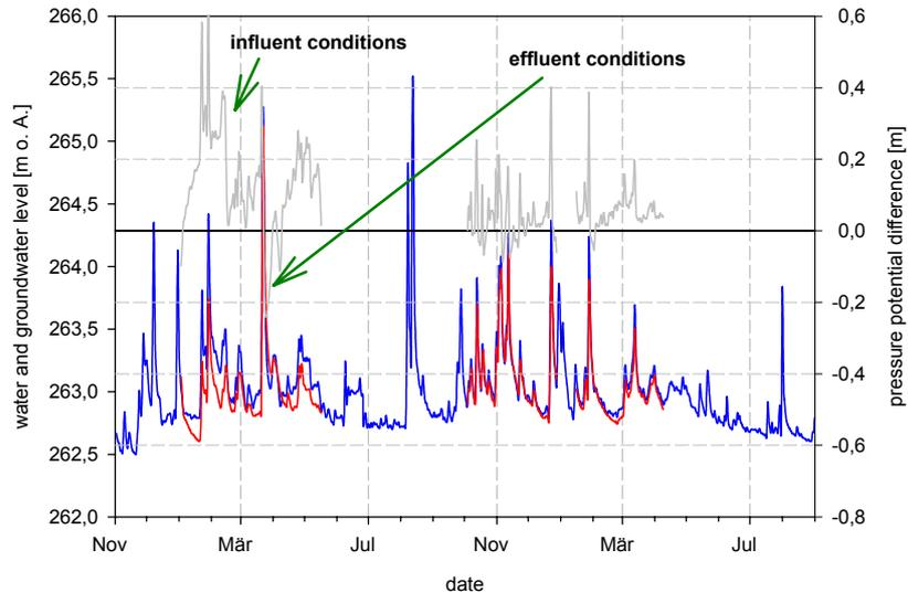
**Figure 5-40:** Surface water and groundwater levels at gauging station “Greimpersdorf” (November 2001 – September 2003). Blue lines = surface water levels; red lines = groundwater levels. Grey line = pressure potential difference between surface water and groundwater.
