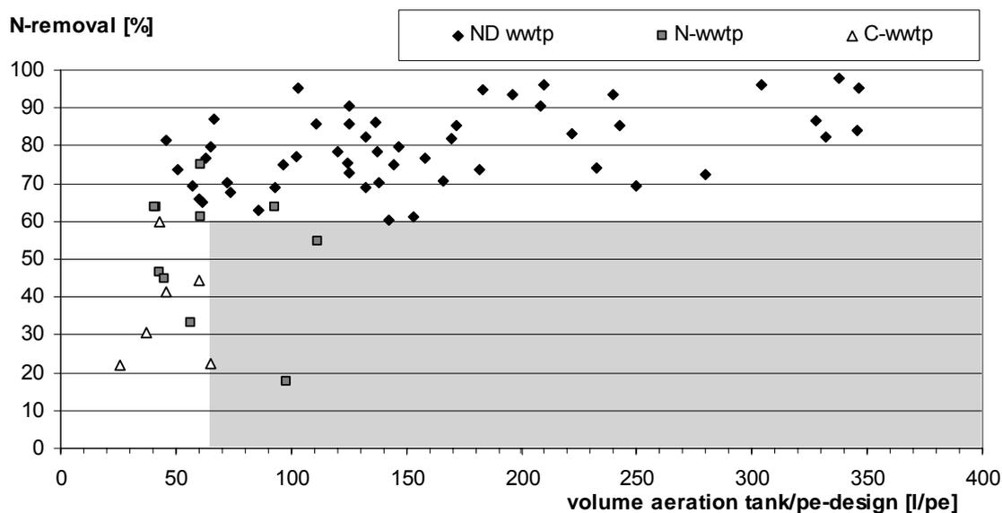
**Figure 29** N-removal rates in dependency of the specific volume of the aeration tank.
