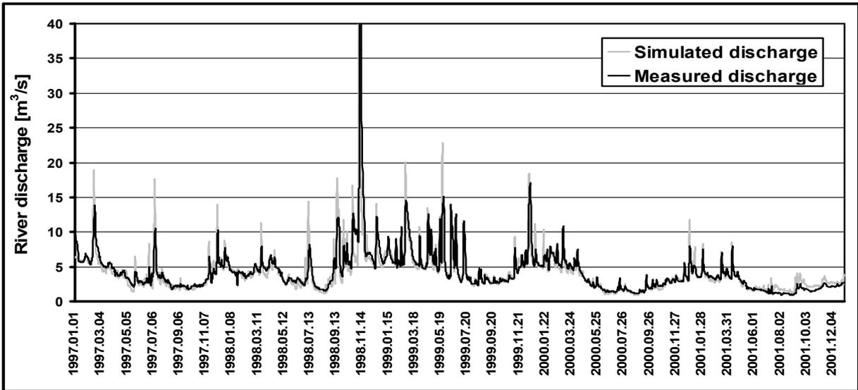
Figure 1: Simulated and measured daily river discharges of SWAT model in Zala catchment
