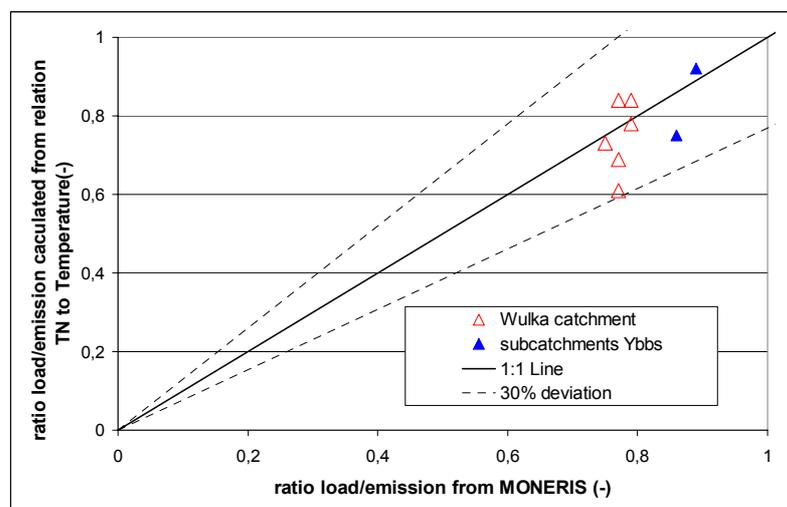
**Figure 9-11:** Comparison of nitrogen retention in surface waters calculated with the MONERIS approach (hydraulic load) and calculated from the correlation between temperature and total nitrogen concentrations
