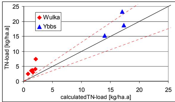
**Figure 9-5:** Comparison of calculated and measured nitrogen loads of different catchments (retention approach based on the specific runoff)
