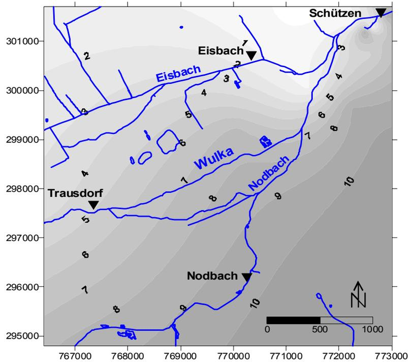
**Figure 5-47:** Average O<sub>2</sub> groundwater concentrations in the area of “Schützen”
