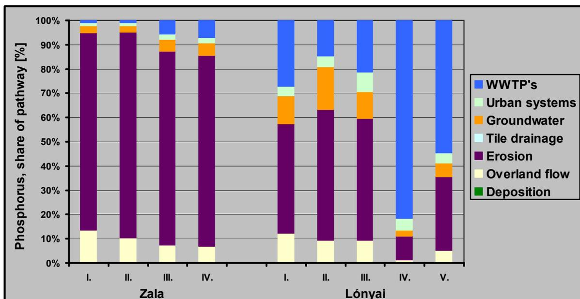
Figure 52: Share of different pathways on total phosphorus emission calculated with the modified MONERIS model (for the period 1997-2001)
