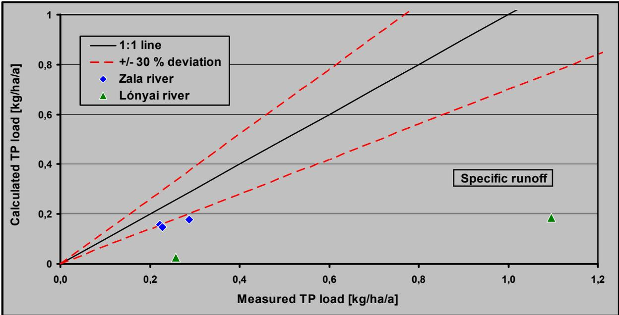
Figure 58: Comparison of measured and modeled TP load calculated based on the modified MONERIS model in dependence on specific runoff (for the period 1997-2001)
