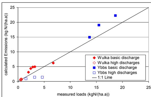
**Figure 9-9:** Comparison of calculated nitrogen emissions and measured loads for basic discharge and high discharges
