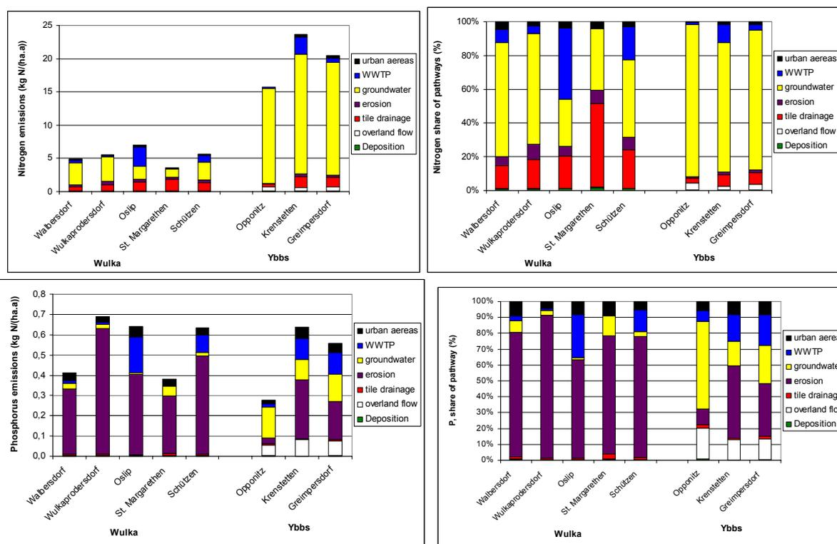
**Figure 6-1:** Graphical presentation of nutrient emissions (N+P) via pathways calculated based on MONERIS approach for the Ybbs and Wulka catchment including total subcatchments
