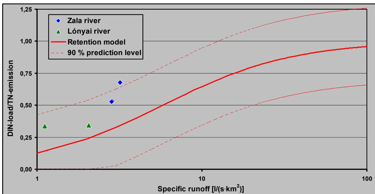
Figure 55: Ratio between measured and modeled DIN load and TN emission calculated with the modified MONERIS model in dependence on specific runoff (for the period 1997-2001)
