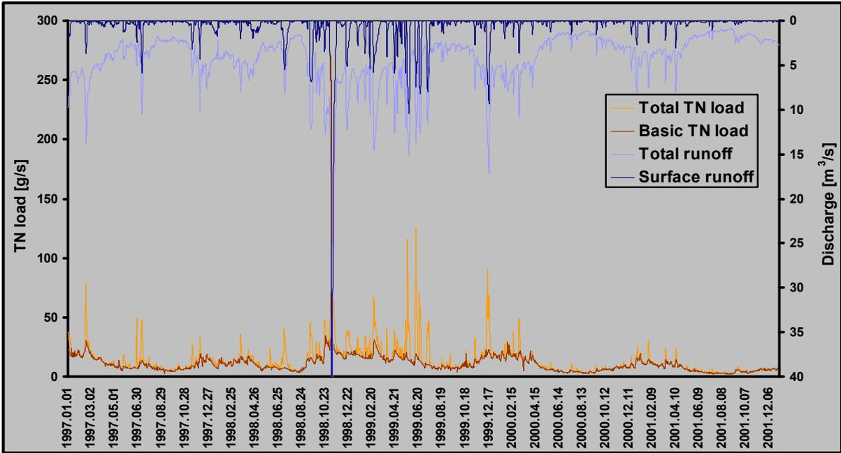
Figure 25: Separated “basic” and total nitrogen load at Zalaapáti station in Zala River (1997-2001)
