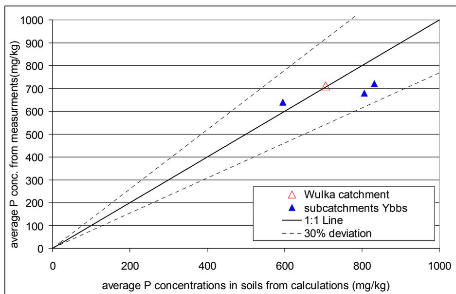
**Figure 9-4:** Comparison of measured and calculated average TP concentrations in soils for different catchments
