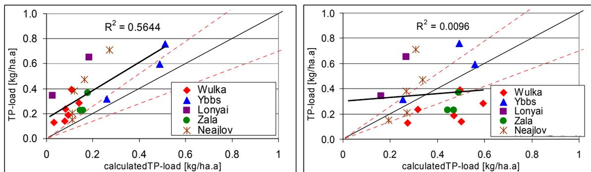
**Figure 39:** Comparison of calculated and measured phosphorus loads of different catchments with retention approach based on the specific runoff (left) and retention approach based on the hydraulic load (right)
