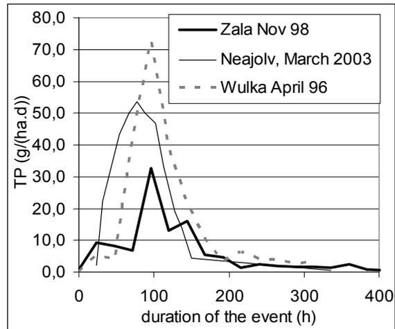
**Figure 23:** Time series of total phosphorus loads during high flow events at Zala, Neajlov and Wulka
