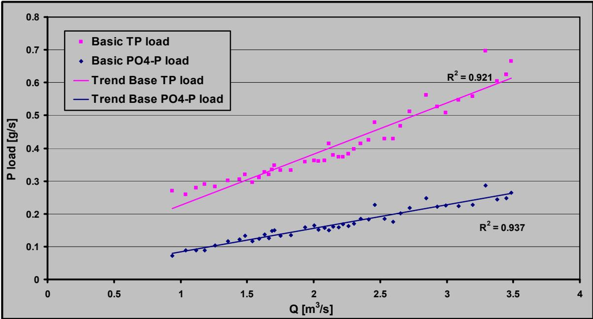
Figure 23: Correlation between base flow discharge and phosphorus loads transported on days without surface runoff contribution at Zalaapáti station in Zala River
