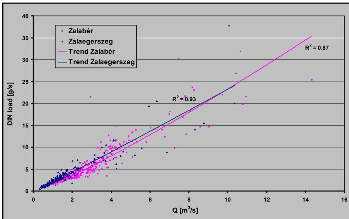
Figure 12: Correlation between river discharge and DIN load at different sampling points of Zala River
