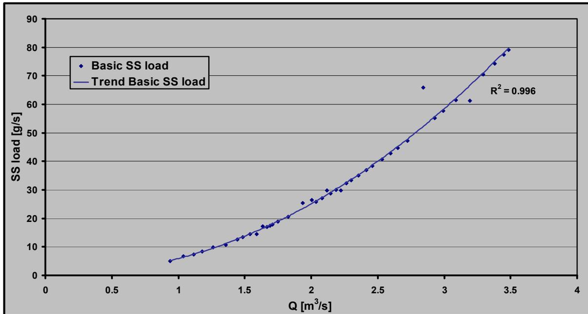
Figure 21: Correlation between base flow discharge and suspended solids load transported on days without surface runoff contribution at Zalaapáti station in Zala River
