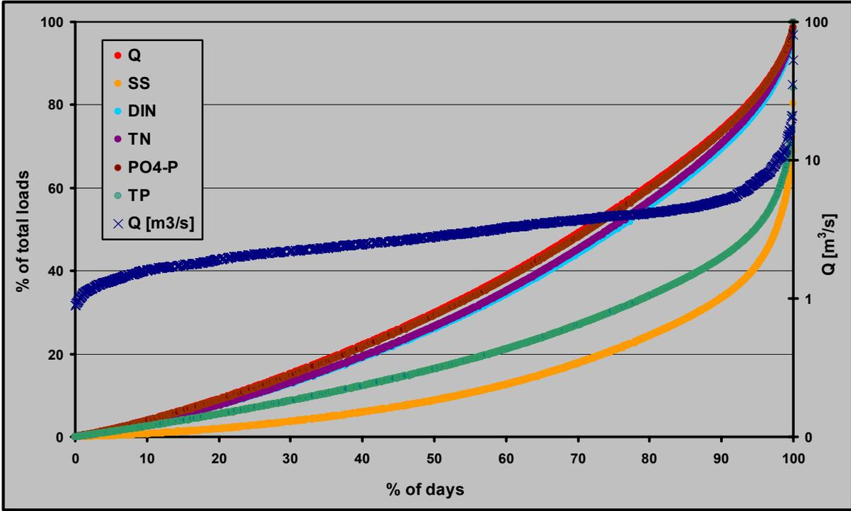
Figure 17: Frequency distribution of river discharge and share of different river loads on the total fluxes at share of days at Zalabér station in Zala River
