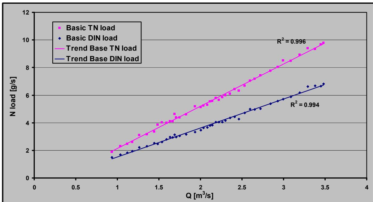
Figure 22: Correlation between base flow discharge and nitrogen loads transported on days without surface runoff contribution at Zalaapáti station in Zala River
