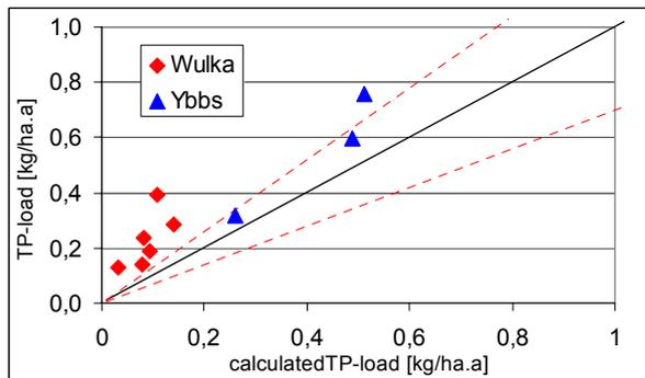
**Figure 9-7:** Comparison of calculated and measured phosphorus loads of different catchments (retention approach based on the specific runoff)
