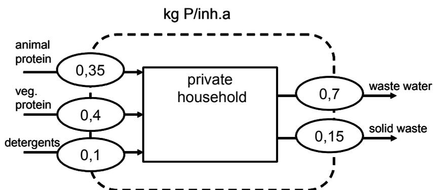
**Figure 8-5:** specific P-flows in kg P/inh.a (total 0,85 kg/inh.y = 1,89 g/inh.d)
