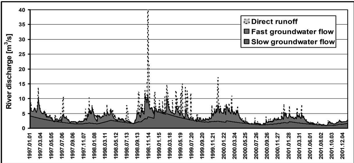
Figure 2: Separated daily river discharge components of DIFGA model in Zala catchment
