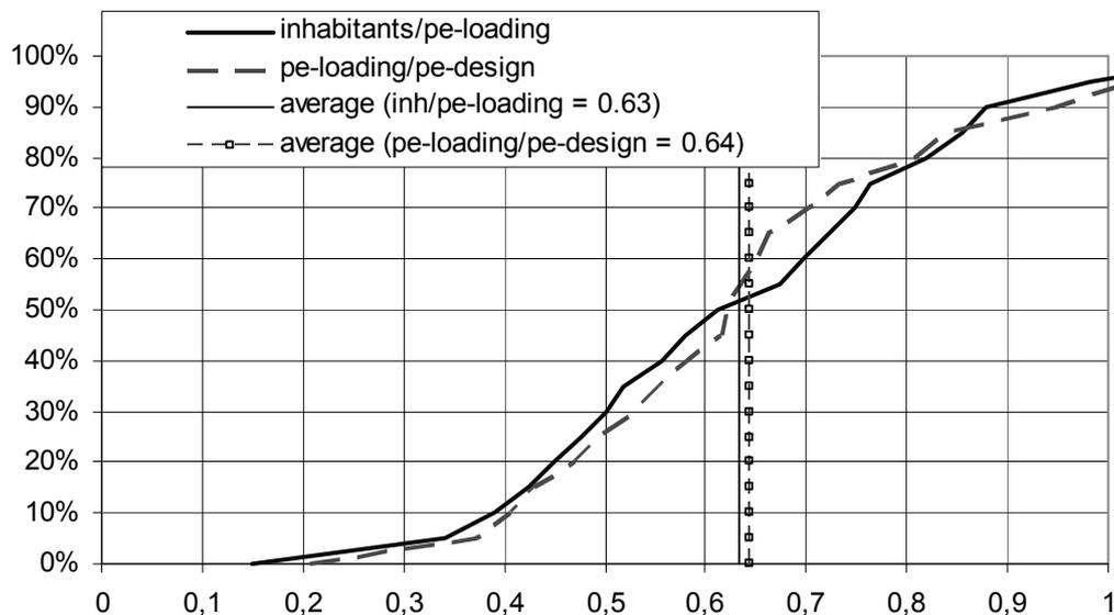
**Figure 28** Probability curves of the relation between connected inhabitants and actual pe-loading and between actual pe-loading and the pe-design capacity.
