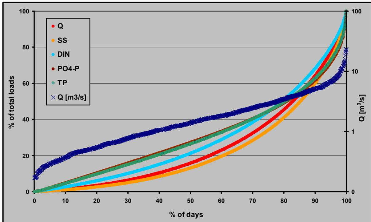
Figure 20: Frequency distribution of river discharge and share of different river loads on the total fluxes at share of days at Buj-Kótaj station in Lónyai River
