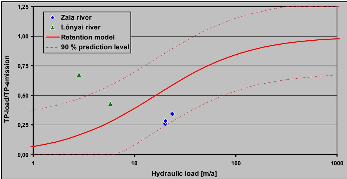
Figure 61: Ratio between measured and modeled TP load and TP emission calculated with the modified MONERIS model in dependence on hydraulic load (for the period 1997-2001)
