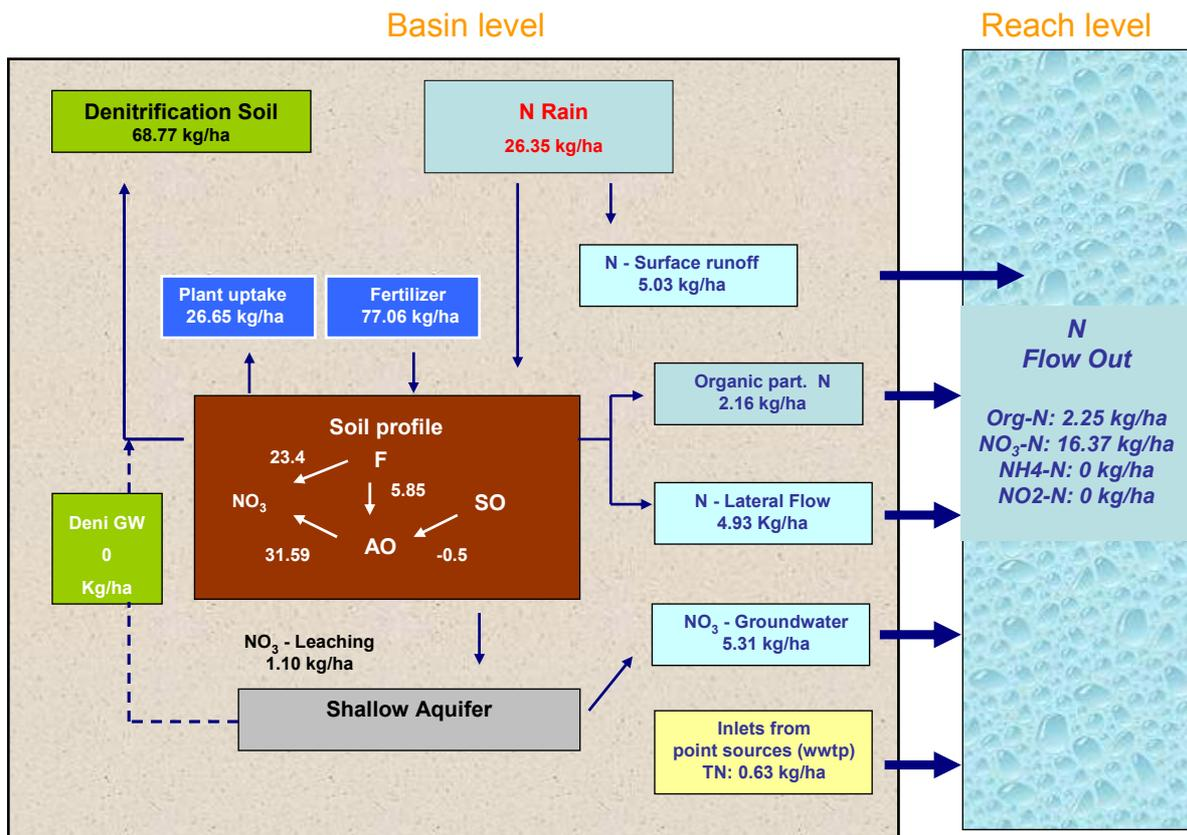
**Figure 7-3:** Nitrogen balance for the Ybbs catchment calculated with the SWAT 2000 model (average values for the calculation period 1991 – 2001)
