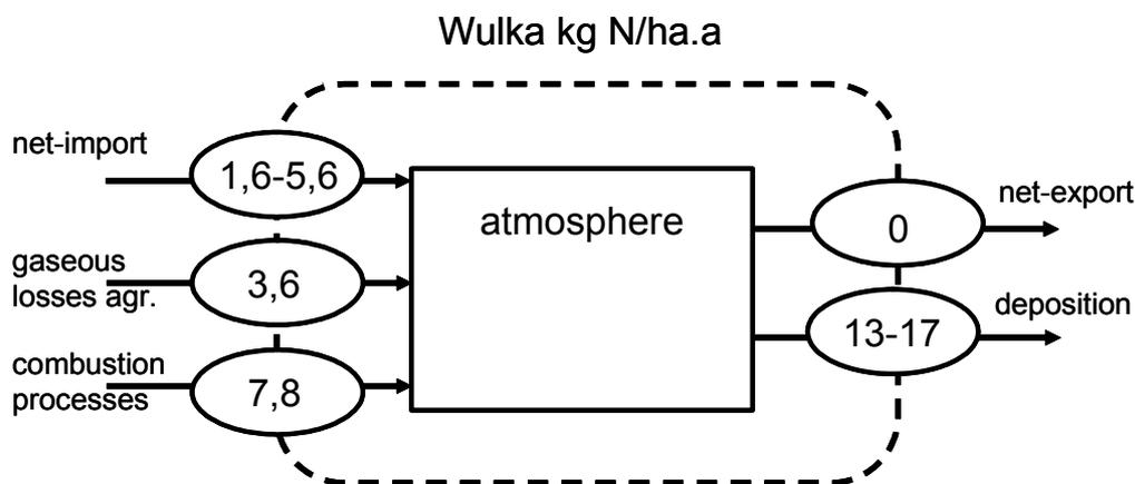
**Figure 8-15:** emissions to the atmosphere in the Wulka area
