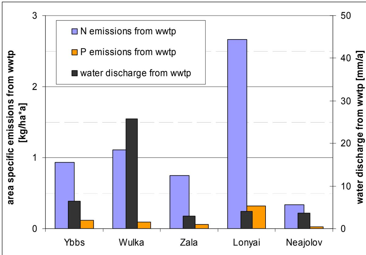
**Figure 4:** Area specific N and P emission from wwtp to the rivers and the water discharge to total river discharge in the 5 CSA
