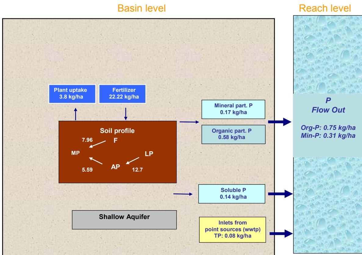
**Figure 7-4:** Phosphorus balance for the Ybbs catchment calculated with the SWAT 2000 model (average values for the calculation period 1991 – 2001)
