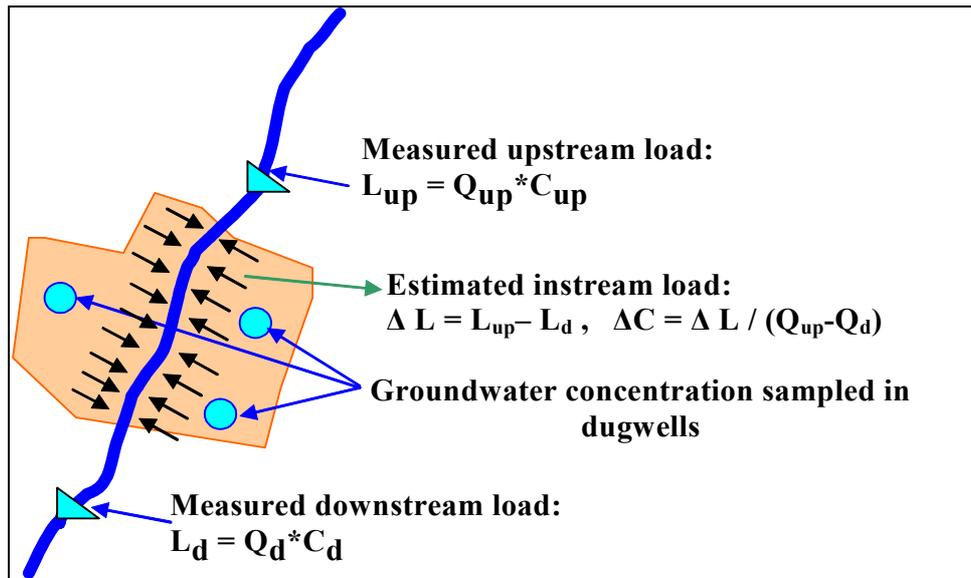
Figure 31: Estimation of nutrient loads via groundwater infiltration
