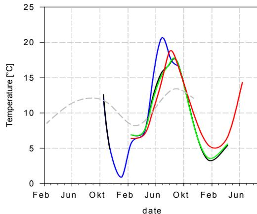
**Figure 5-41:** Temperature in groundwater at different distances from river Ybbs (February 2000 - June 2002). Blue line = surface water; black line = multi level well [0.2m]; green line = multi level well [0.5m]; red line = groundwater well d1 [40m]; grey dotted line = groundwater well 326777 [380m].
