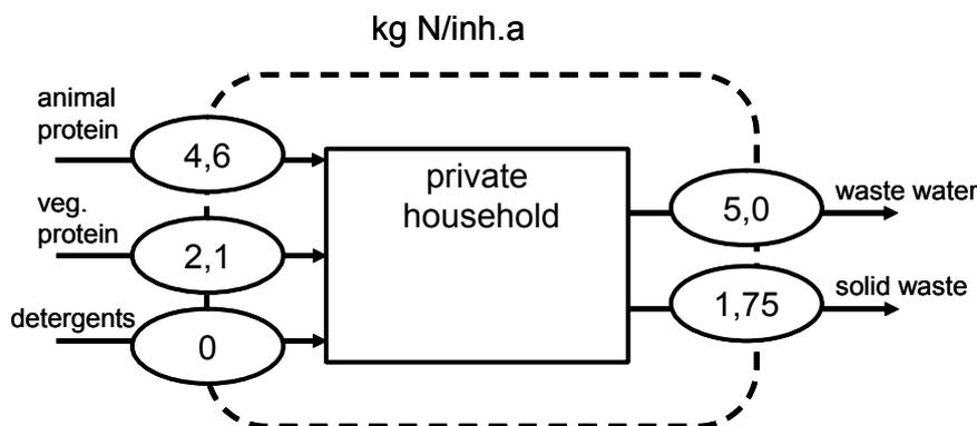
**Figure 8-4:** specific N-flows in kg N/inh.a (total 6,75 kg/inh.y = 13,74 g/inh.d)
