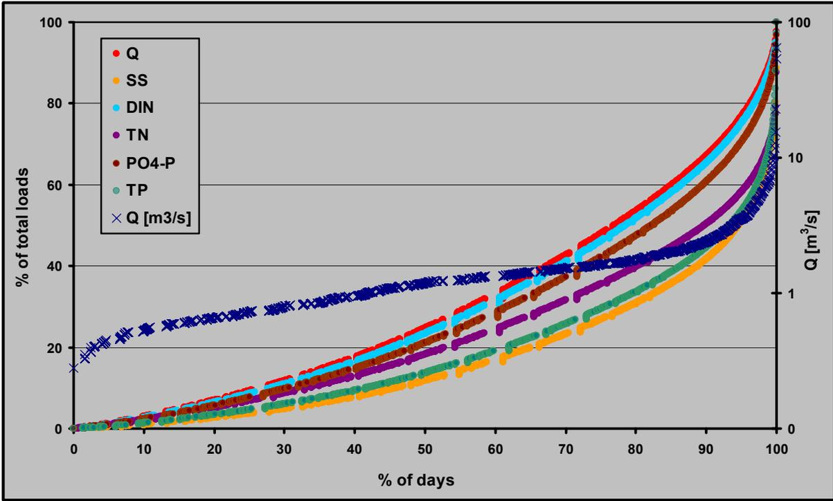
Figure 16: Frequency distribution of river discharge and share of different river loads on the total fluxes at share of days at Zalaegerszeg station in Zala River
