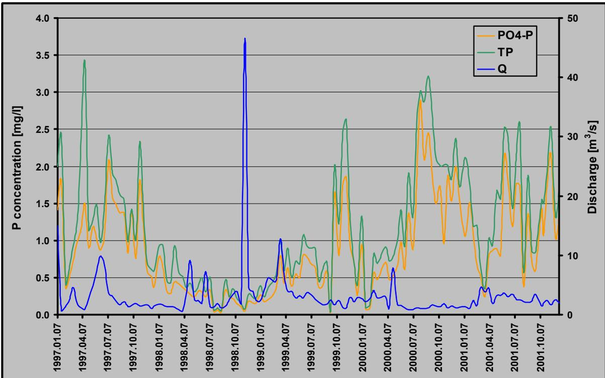
Figure 11: Dynamics of river discharge and phosphorus concentrations of Lónyai River at Buj-Kótaj station (1997-2001)
