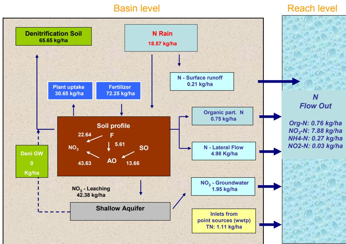
**Figure 7-1:** Nitrogen balance for the Wulka catchment calculated with the SWAT 2000 model (average values for the calculation period 1992 – 1999)
