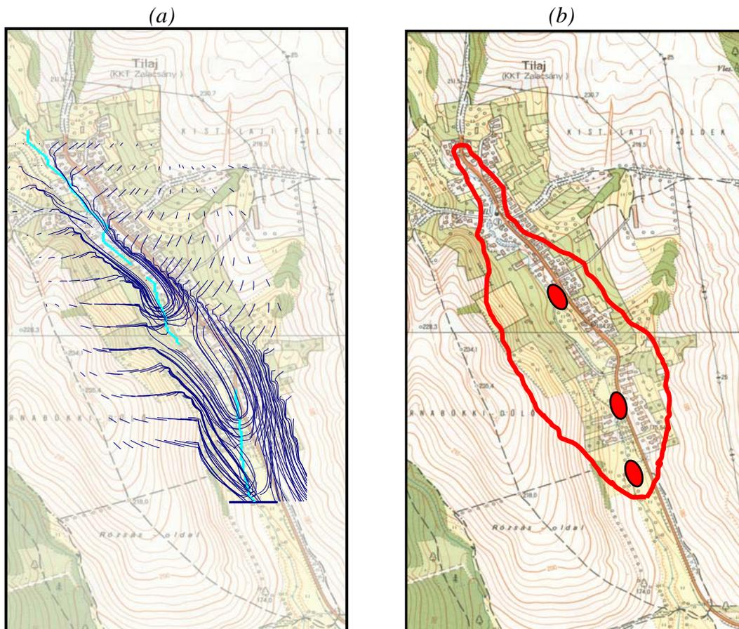
*Figure 35: Groundwater streamlines started from the level of water table (a) and the extension of area drained by the creek (b); (the majority of the drained water enters into the riverbed at the three highlighted small areas in Fig. b.)*
