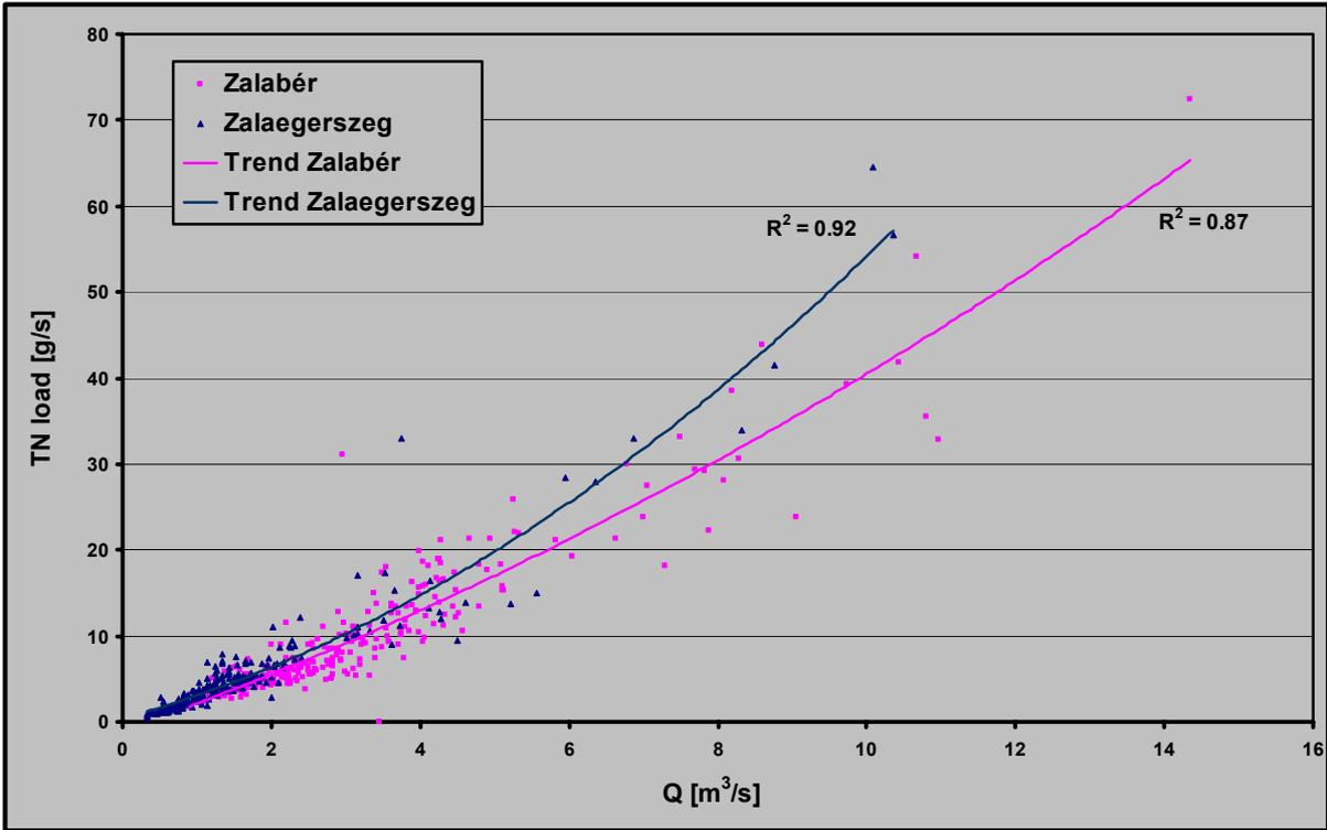
Figure 13: Correlation between river discharge and TN load at different sampling points of Zala River
