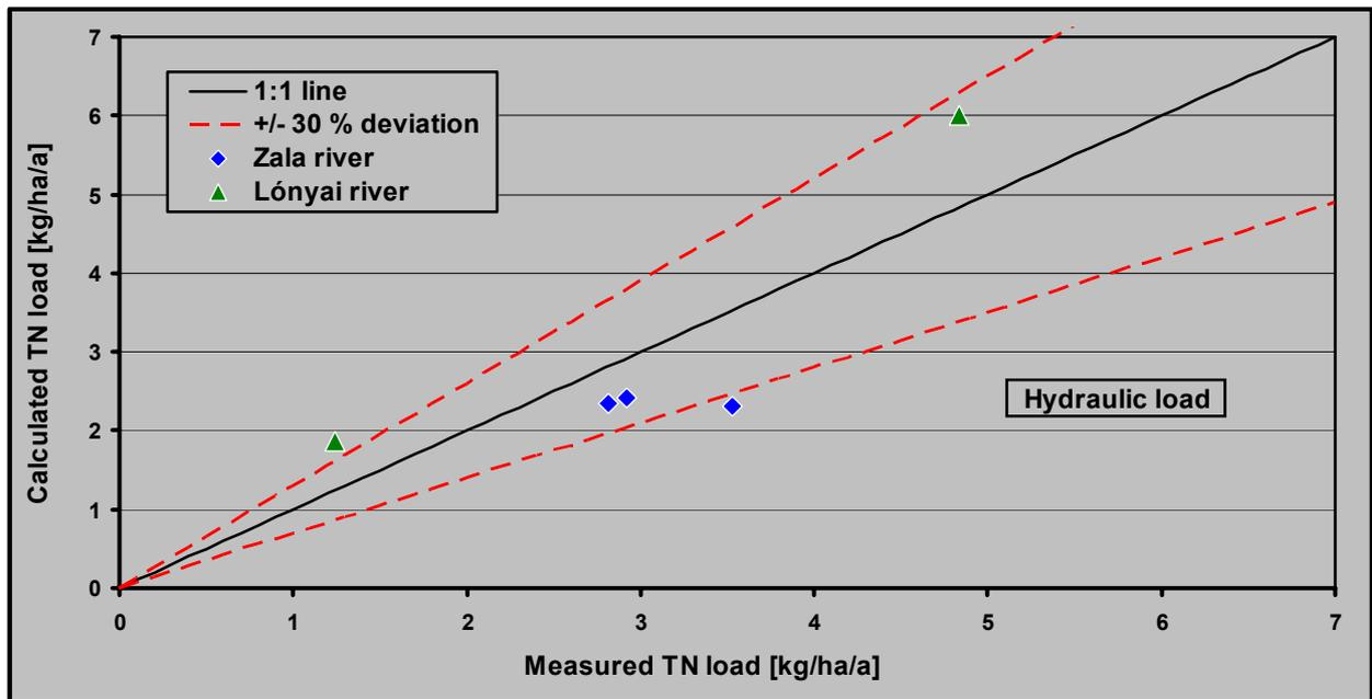
Figure 64: Comparison of measured and modeled TN load calculated based on the modified MONERIS model in dependence on hydraulic load (for the period 1997-2001)
