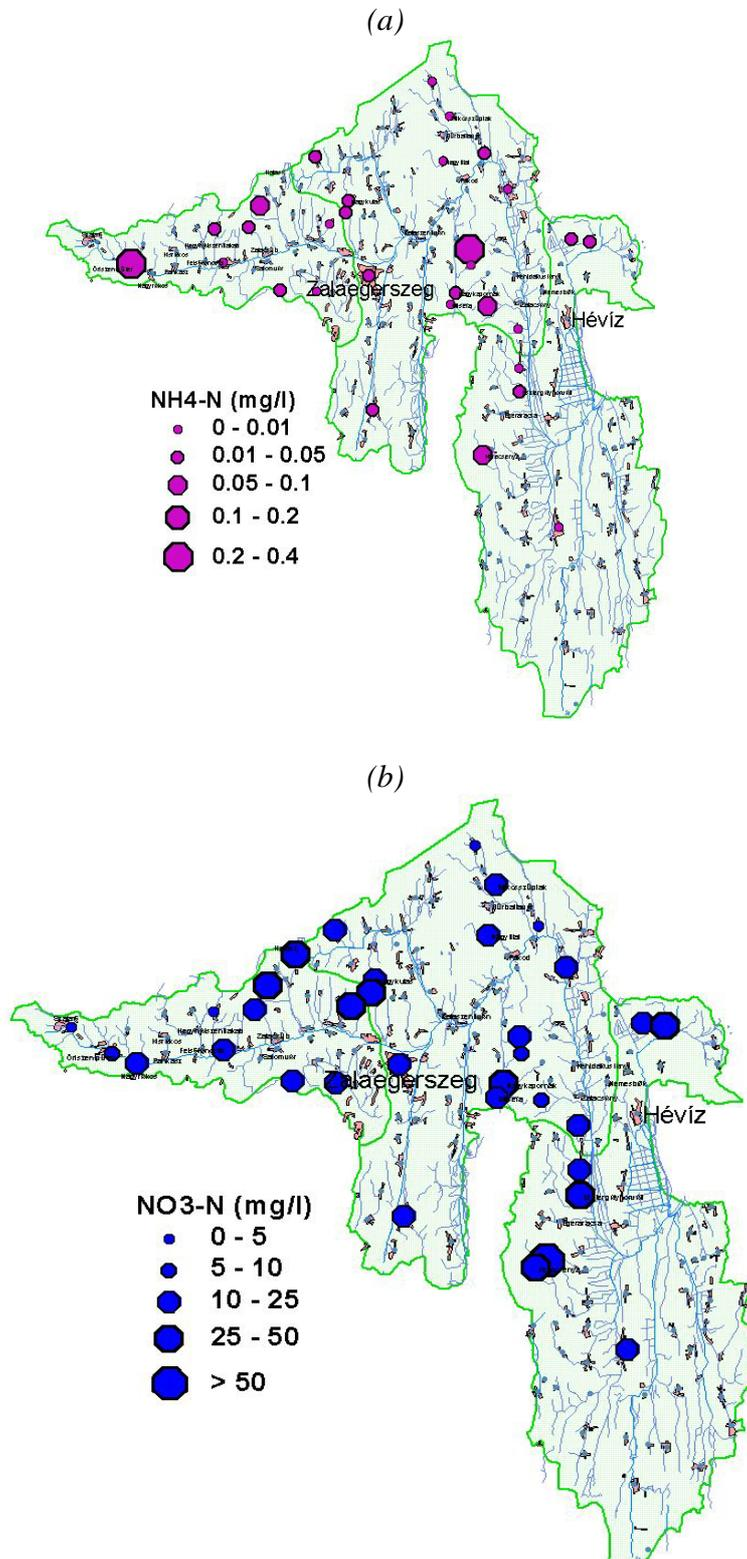
Figure 27: Average ammonium (a) and nitrate (b) concentrations measured in dug wells in the Zala catchment
