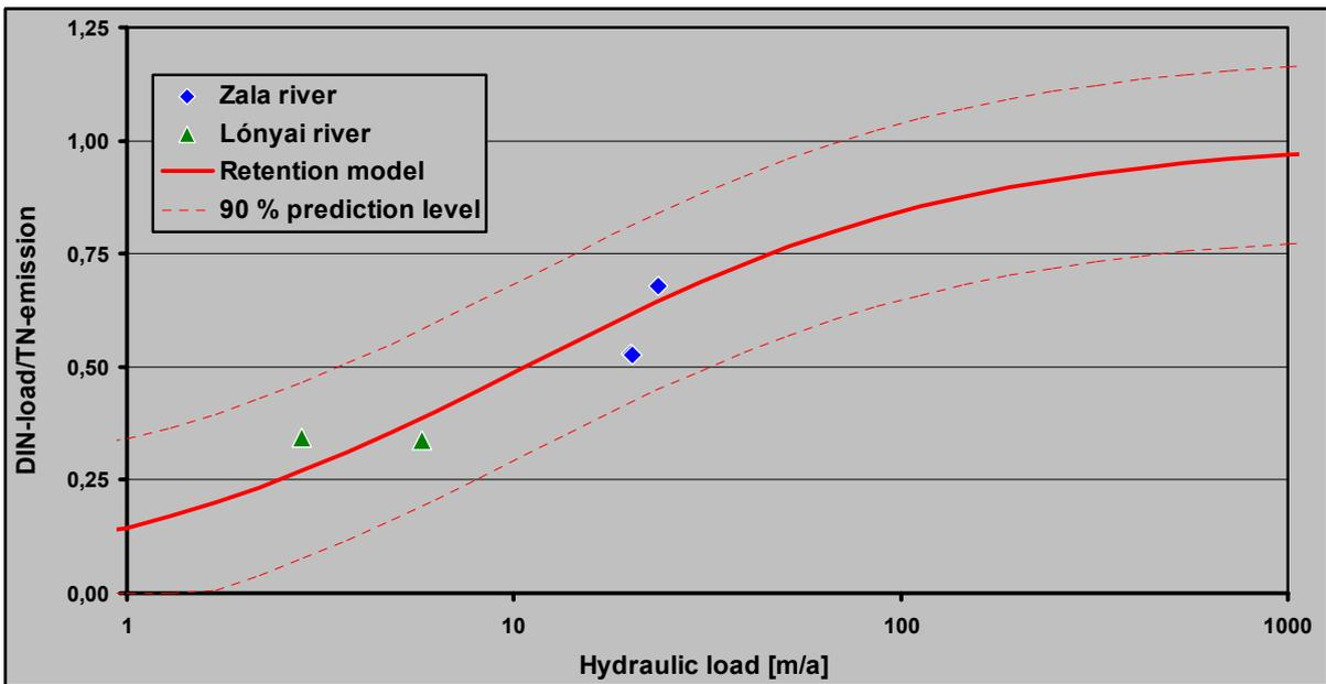
Figure 59: Ratio between measured and modeled DIN load and TN emission calculated with the modified MONERIS model in dependence on hydraulic load (for the period 1997-2001)
