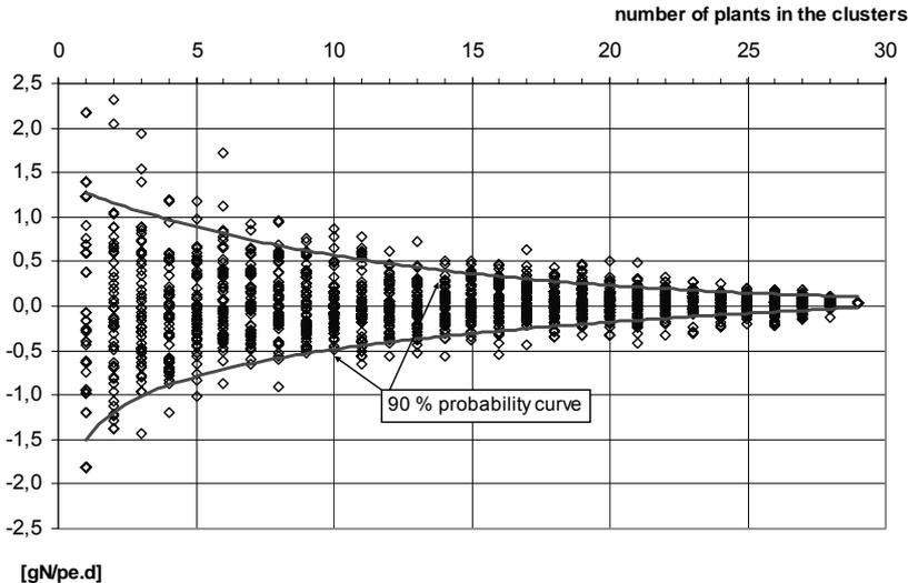
**Figure 30** Deviation of estimated from measured specific nitrogen loads dependent of the number of treatment plants considered together in a cluster (estimations of influent loads were based on BOD-load in the influent and connected inhabitants)
