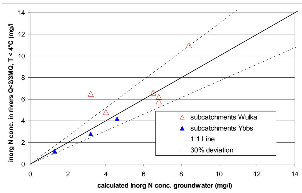
**Figure 9-2:** Comparison of inorganic nitrogen concentrations in surface waters at low temperatures and base flow conditions and calculated nitrogen concentrations in groundwater for different catchment areas
