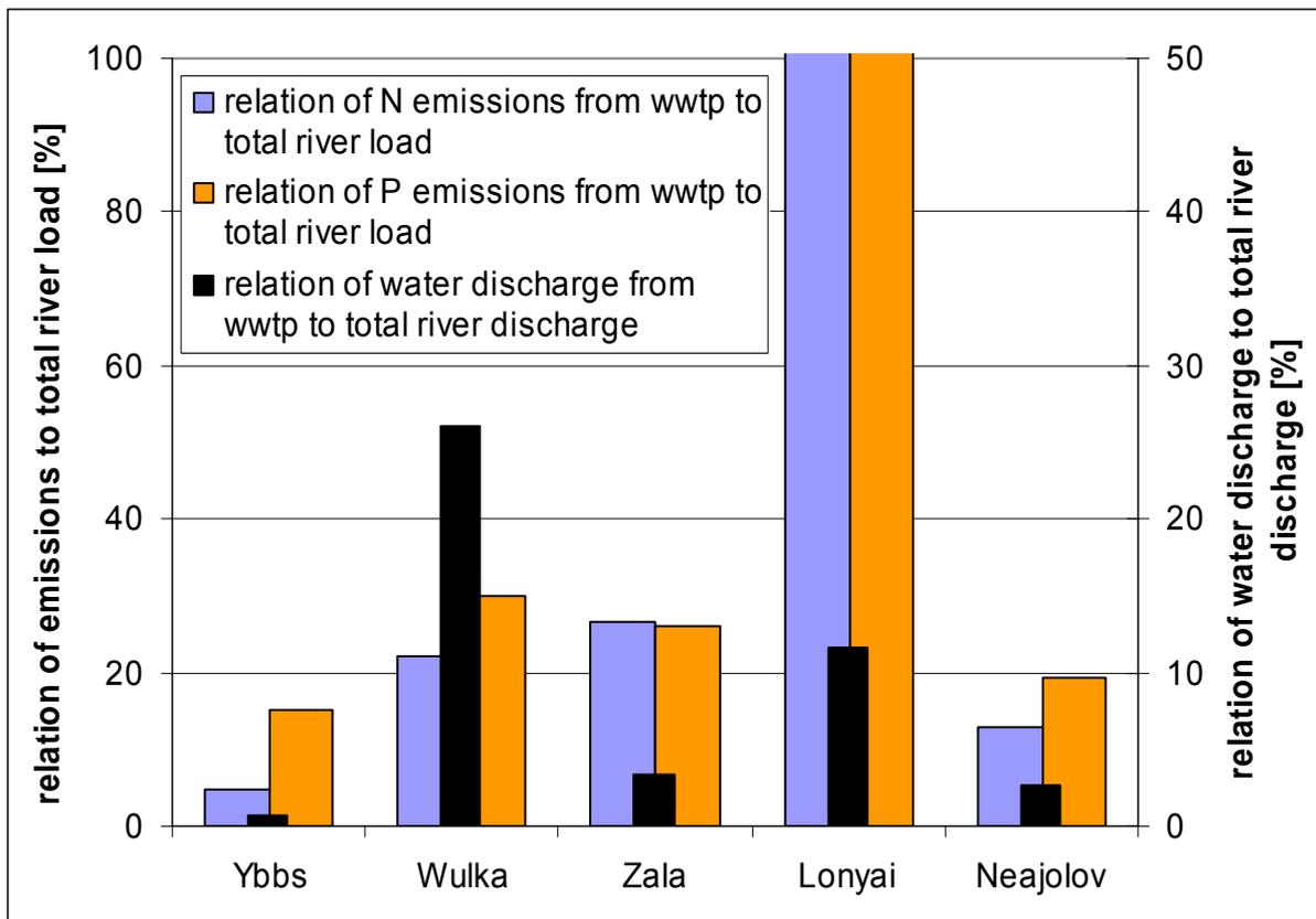
**Figure 5:** Relation of N and P emissions and the water discharge of wwtp to the total N and P river load and the total river discharge of the 5 case study areas
