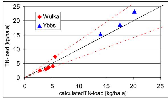
**Figure 9-6:** Comparison of calculated and measured nitrogen loads of different catchments (retention approach based on the hydraulic load)
