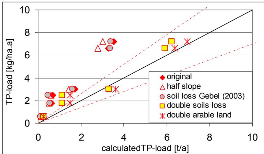
**Figure 9-15:** Sensitivity of MONERIS calculations in the Wulka catchment on slope soil loss values and share of arable land (retention approach based on specific runoff)
