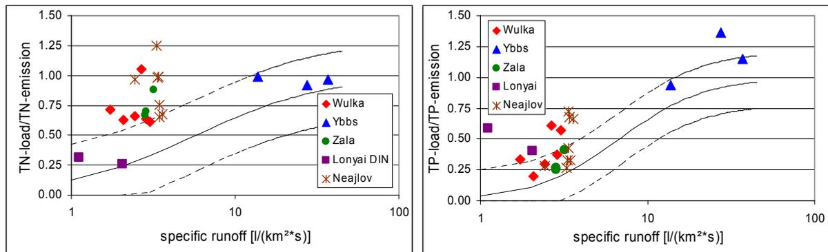
**Figure 36:** Retention of N and P in the river versus the specific runoff of the CSA
