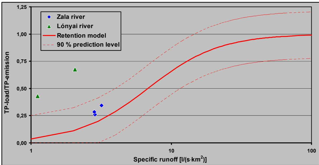
Figure 57: Ratio between measured and modeled TP load and TP emission calculated with the modified MONERIS model in dependence on specific runoff (for the period 1997-2001)
