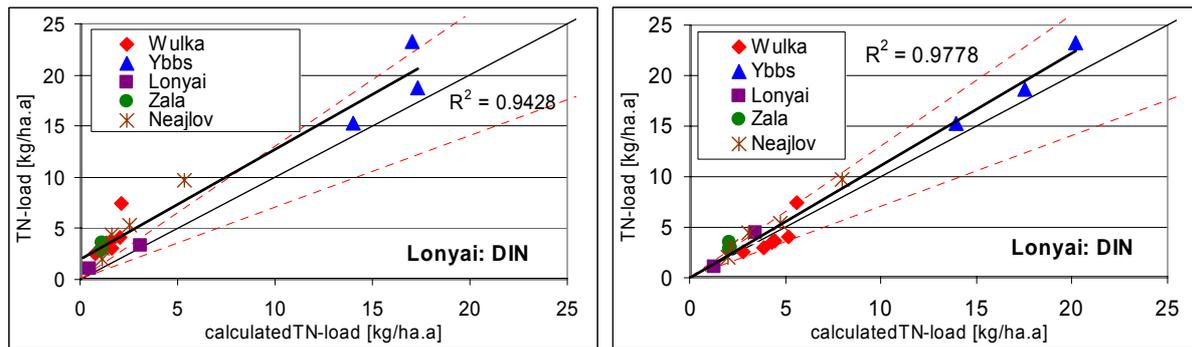
**Figure 38:** Comparison of calculated and measured nitrogen loads of different catchments with retention approach based on the specific runoff (left) and retention approach based on the hydraulic load (right)
