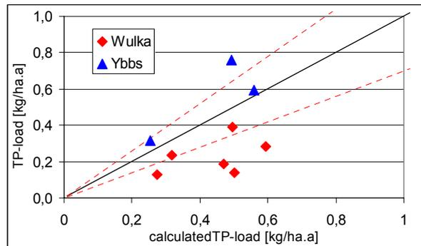
**Figure 9-8:** Comparison of calculated and measured phosphorus loads of different catchments (retention approach based on the hydraulic load)
