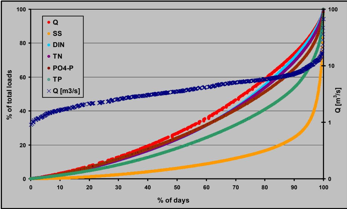
Figure 18: Frequency distribution of river discharge and share of different river loads on the total fluxes at share of days at Zalaapáti station in Zala River
