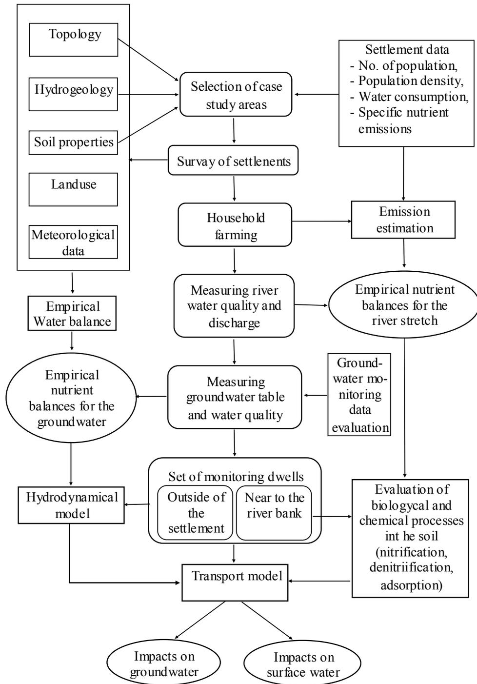
Figure 30: Main steps of the methodology developed for the estimation of the impact of nutrient emissions from non sewered areas
