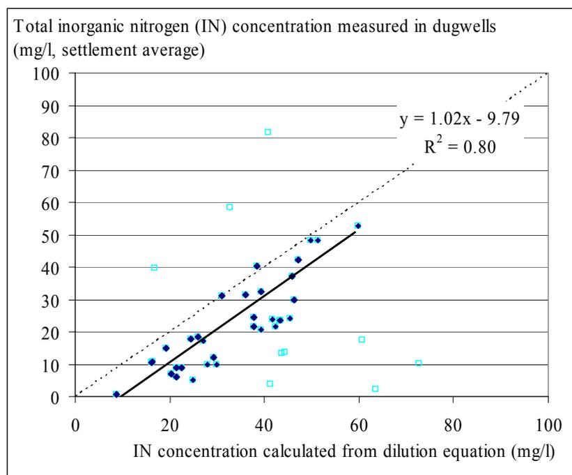
Figure 28: Relationship between the measured and the calculated total dissolved inorganic N concentrations in the groundwater under non sewerred settlements (empty dots were skipped from regression)
