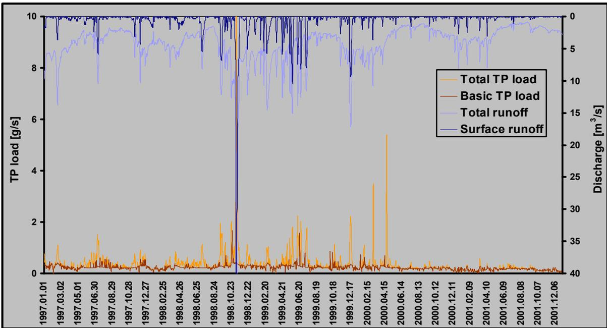
Figure 26: Separated “basic” and total phosphorus load at Zalaapáti station in Zala River (1997-2001)
