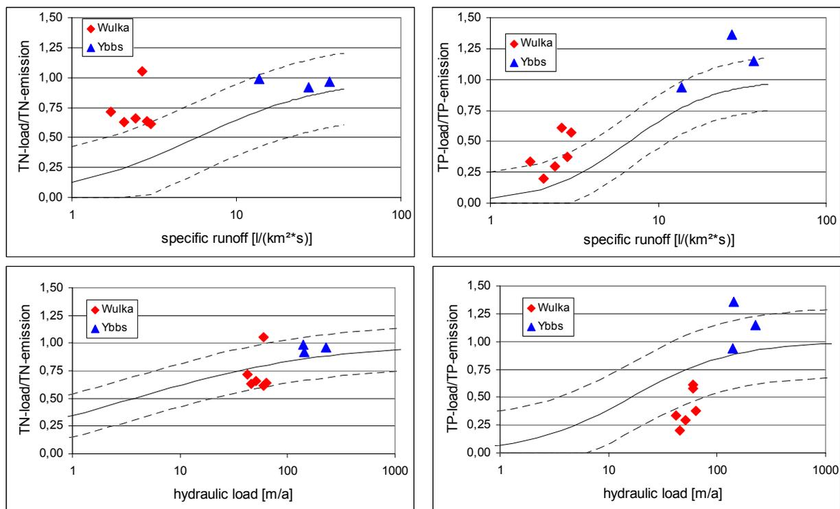
Figure 6-3: Retention versus hydraulic load and area specific runoff for different subcatchments
