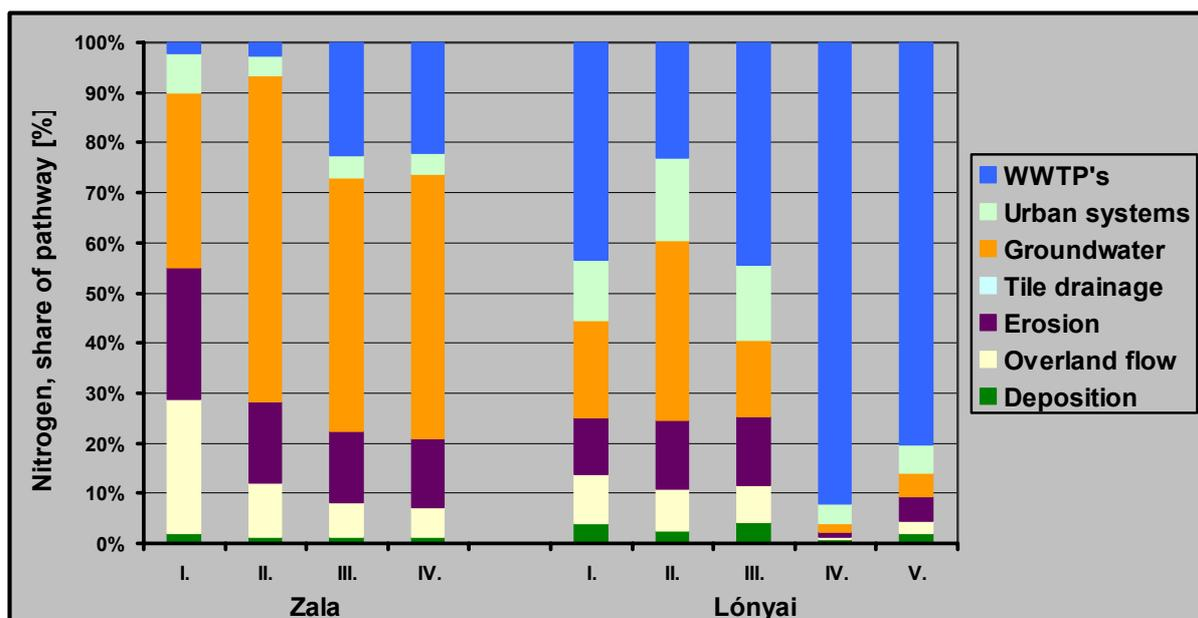
Figure 50: Share of different pathways on total nitrogen emission calculated with the modified MONERIS model (for the period 1997-2001)
