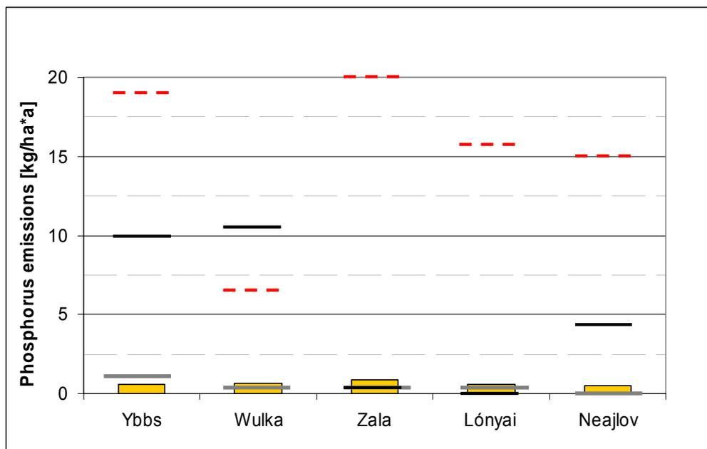
**Figure 32:** Total P emissions with relation to the area specific surplus on the total area of the catchment and the river loads for the 5 CSA
