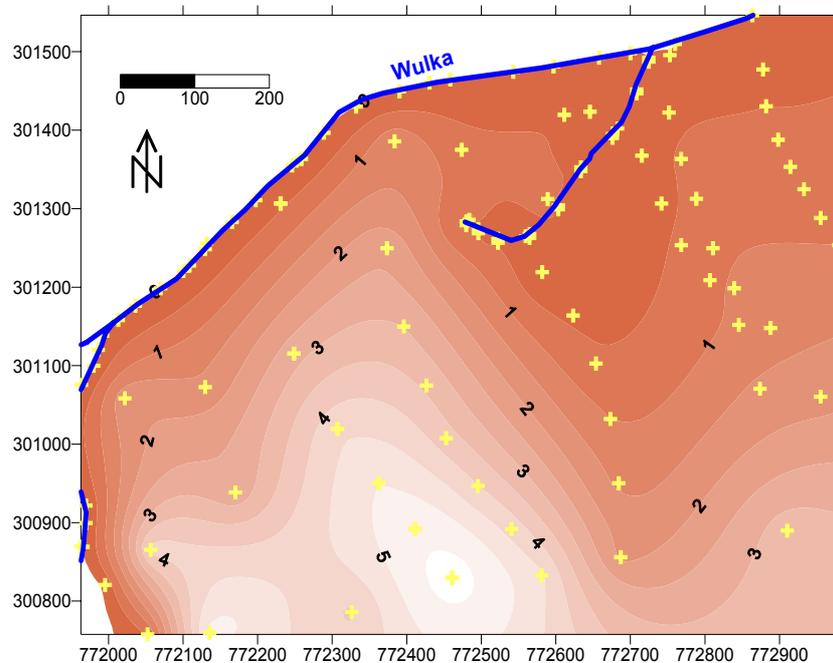
**Figure 5-49:** Mean groundwater residence times (years) interpolated along nine groundwater flow paths south of river Wulka at study site “Schützen”
