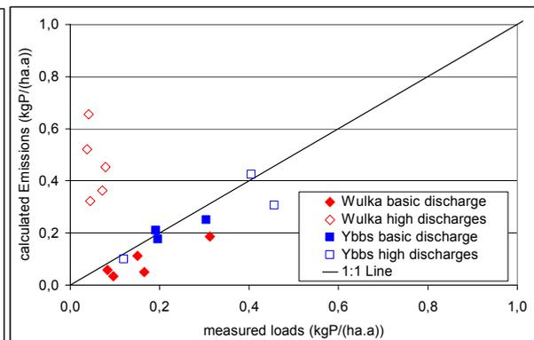
**Figure 9-10:** Comparison of calculated phosphorus emissions and measured loads for basic discharge and high discharges
