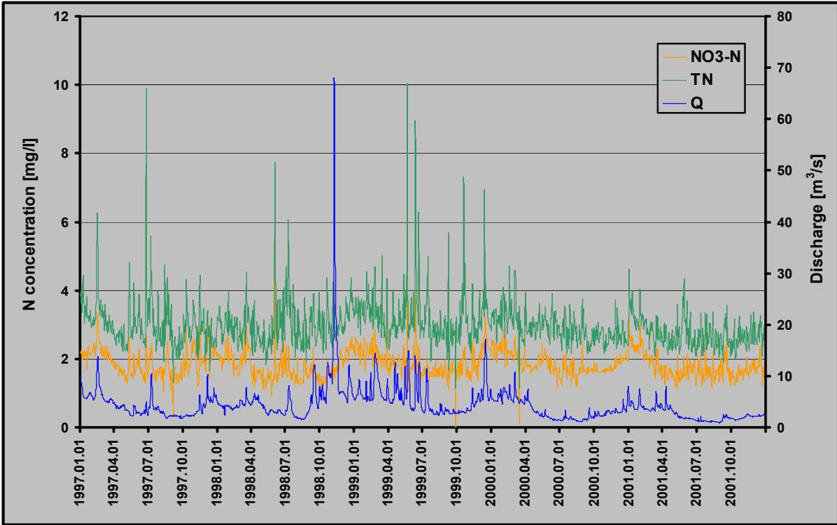
Figure 8: Dynamics of river discharge and nitrogen concentrations of Zala River at Zalaapáti station (1997-2001)
