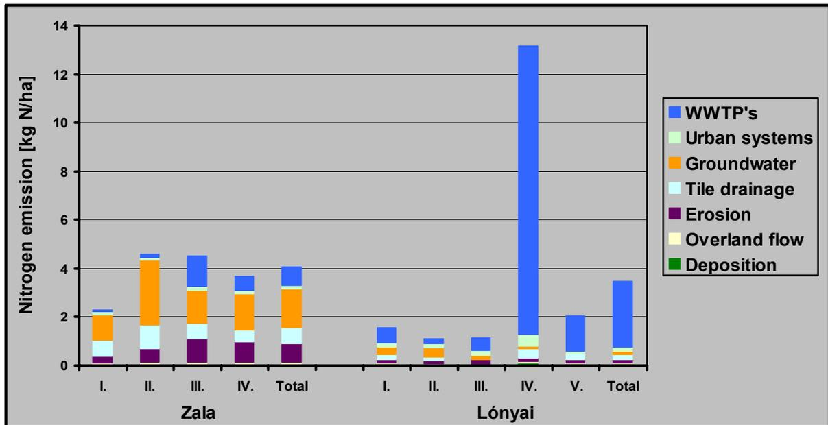
Figure 45: Calculated area-specific nitrogen emissions with the original MONERIS model (for the period 1997-2001)
