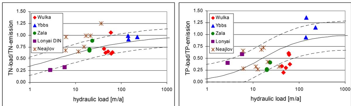
**Figure 37:** Retention of N and P in the river versus the hydraulic load of the CSA
