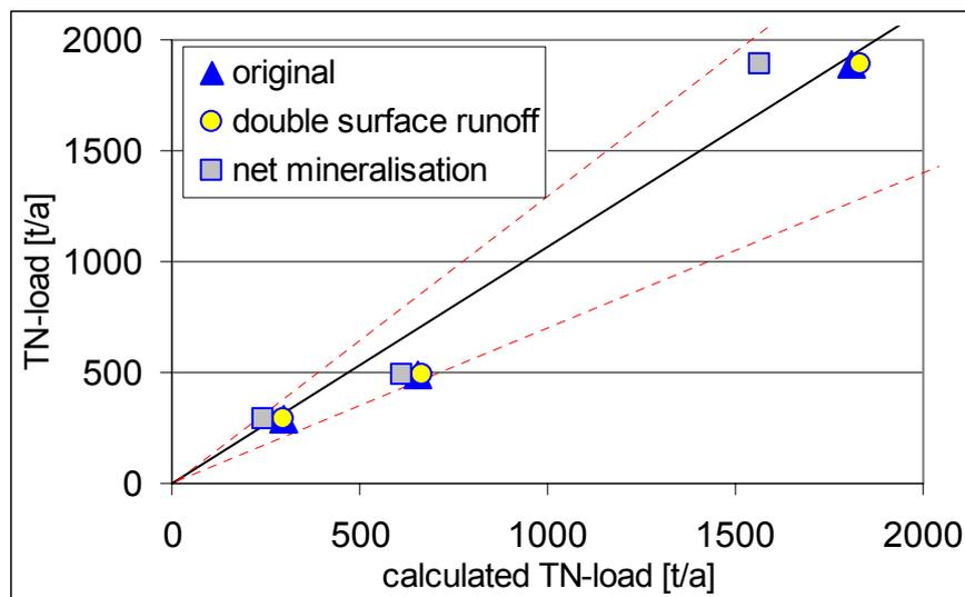
**Figure 9-12:** Sensitivity of MONERIS calculations in the Ybbs catchment on the surface runoff and the consideration of the „net-mineralization“
