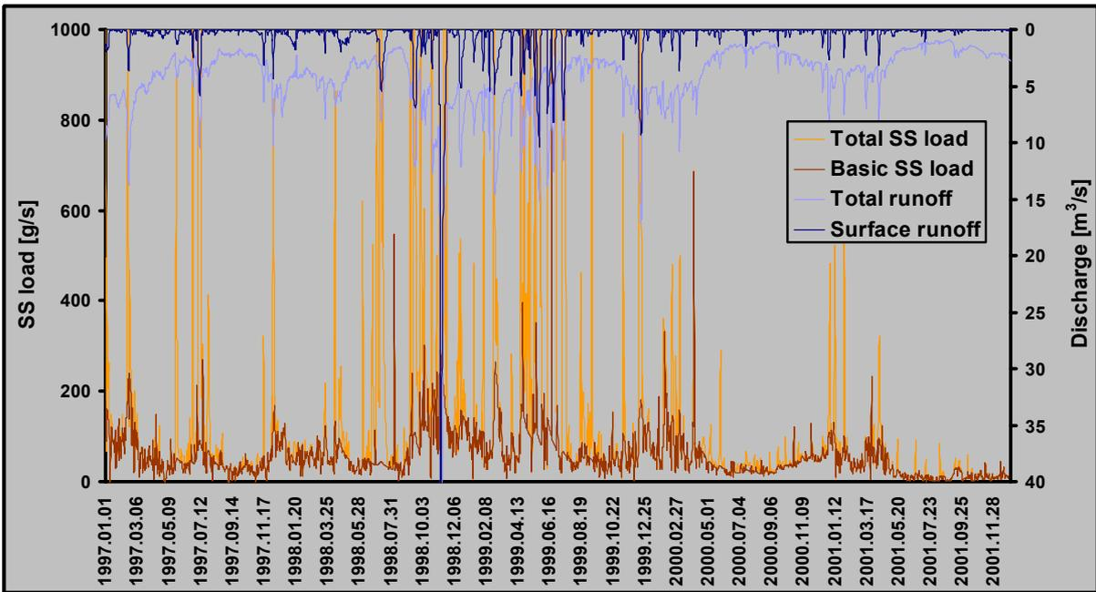
Figure 24: Separated “basic” and total suspended solids load at Zalaapáti station in Zala River (1997-2001)
