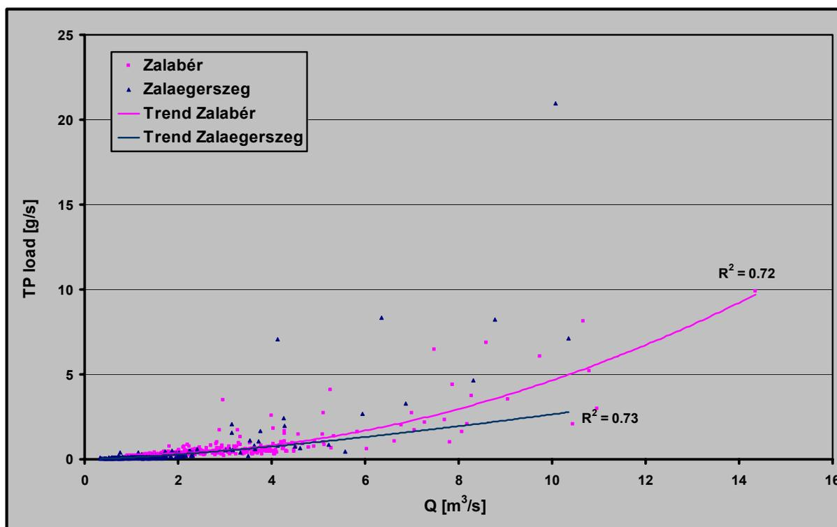
Figure 15: Correlation between river discharge and TP load at different sampling points of Zala River
