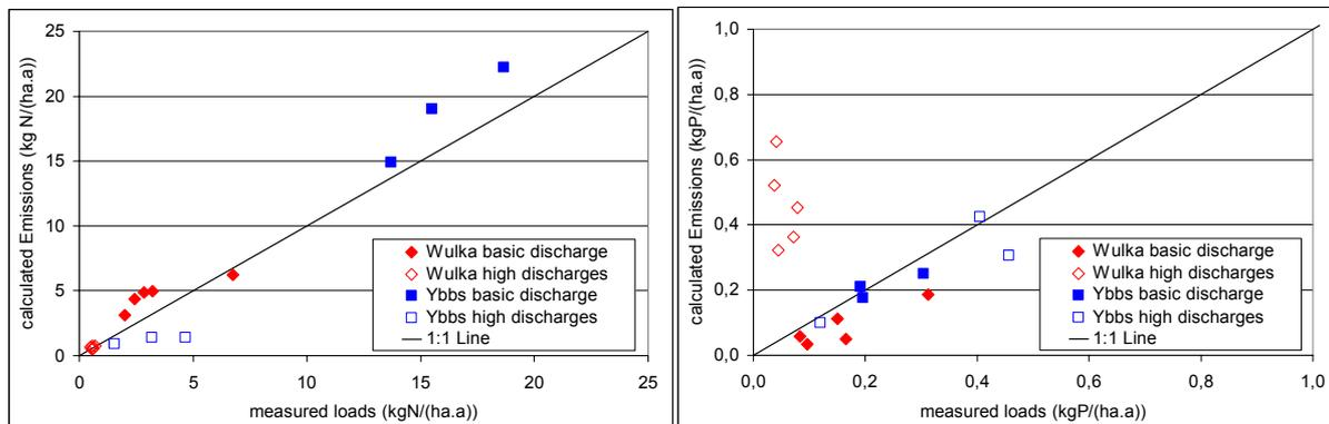
**Figure 40:** Comparison of calculated nitrogen and phosphorus emissions and measured loads for basic discharge and high discharges in the Austrian case study regions
