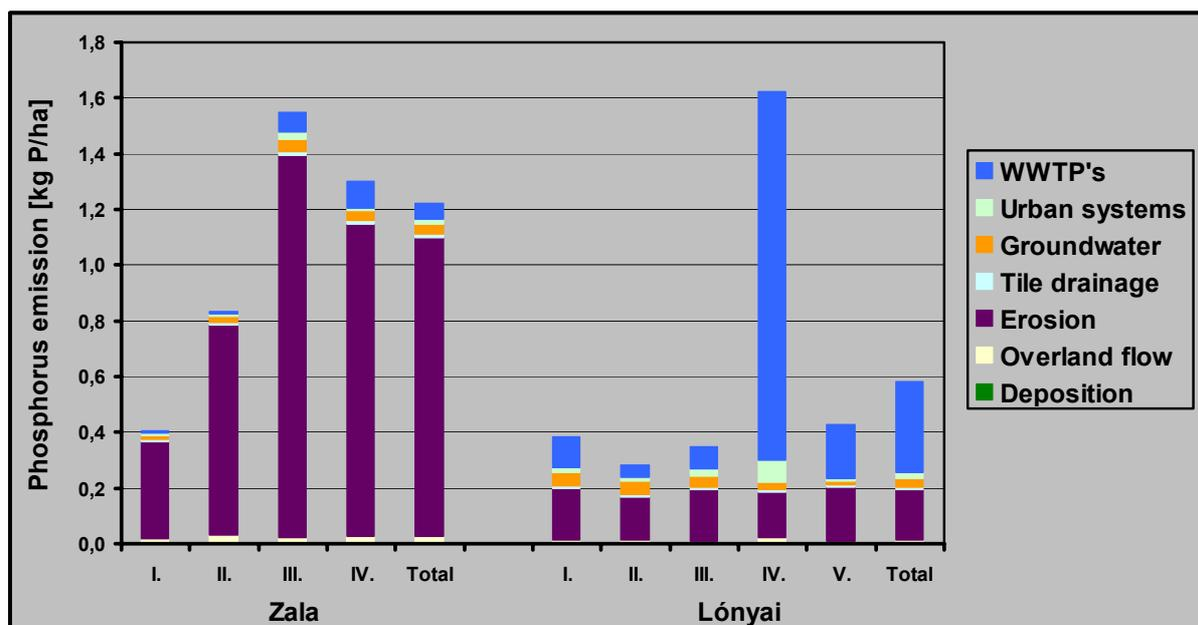
Figure 47: Calculated area-specific phosphorus emissions with the original MONERIS model (for the period 1997-2001)
