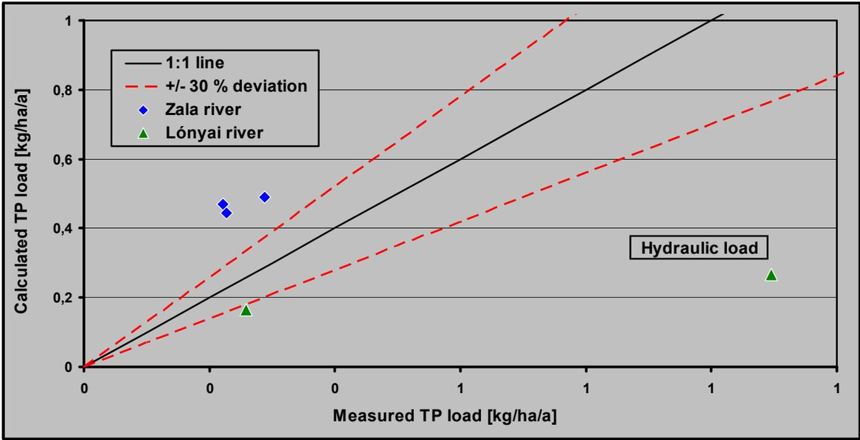
Figure 62: Comparison of measured and modeled TP load calculated based on the modified MONERIS model in dependence on hydraulic load (for the period 1997-2001)
