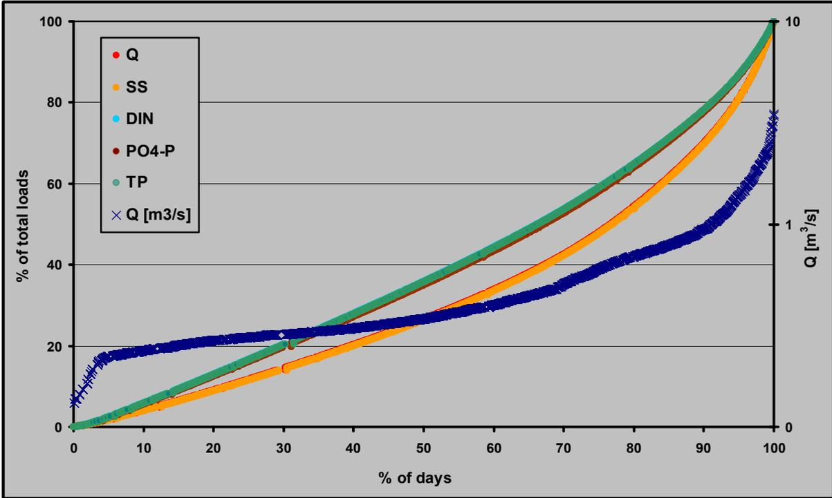
Figure 19: Frequency distribution of river discharge and share of different river loads on the total fluxes at share of days at Szarvassziget station in Lónyai River
