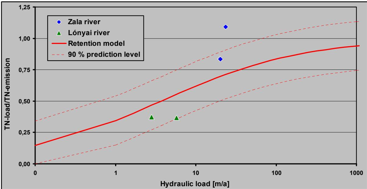
Figure 63: Ratio between measured and modeled TN load and TN emission calculated with the modified MONERIS model in dependence on hydraulic load (for the period 1997-2001)
