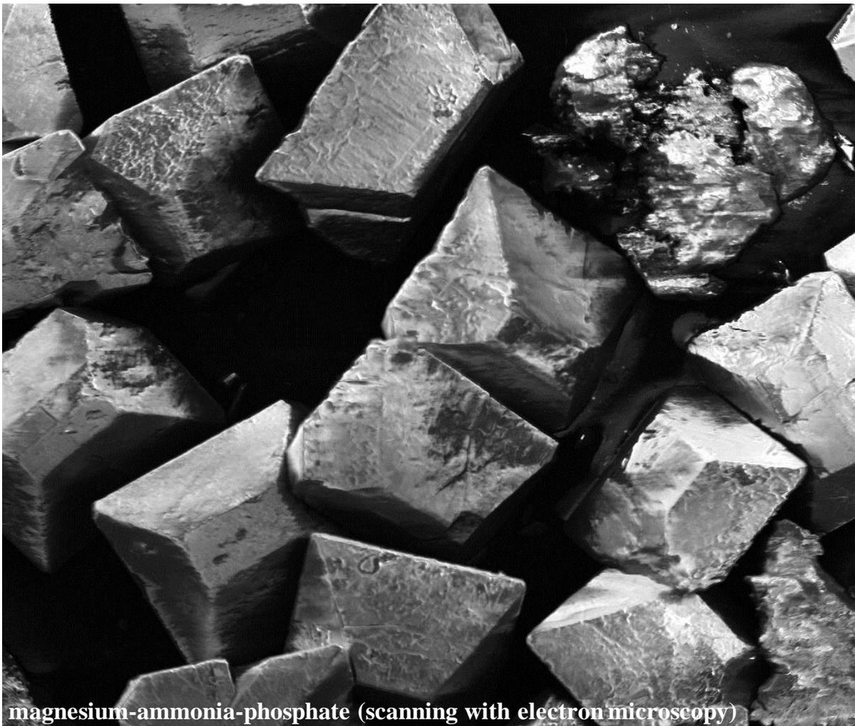
magnesium-ammonia-phosphate (scanning with electron microscopy)
