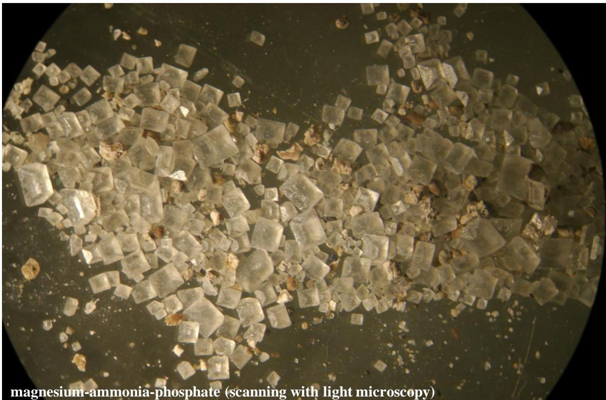
magnesium-ammonia-phosphate (scanning with light microscopy)
