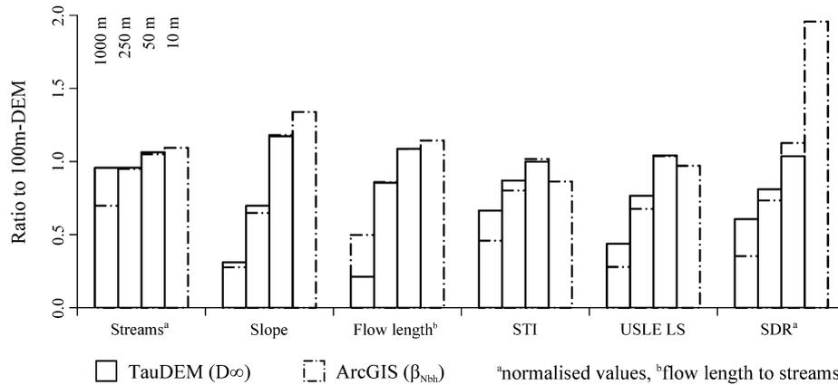
Fig. 4: Effect of DEM resolution on stream delineation and average topographic attributes
