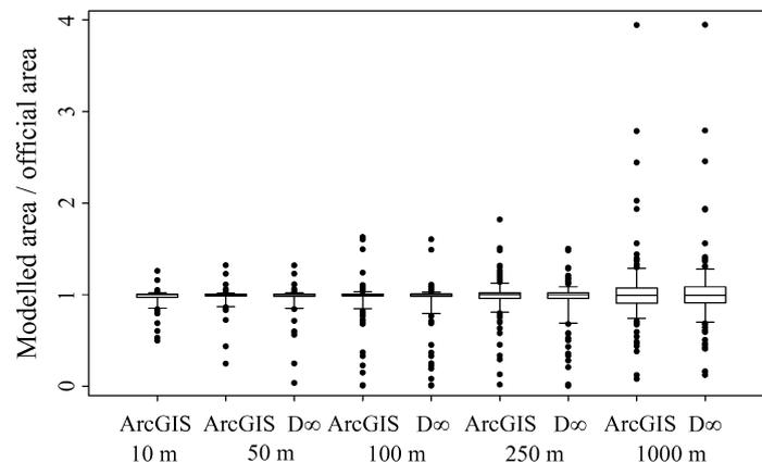
Fig. 2: Modelled area to official area for different DEM resolutions and flow routing algorithms
