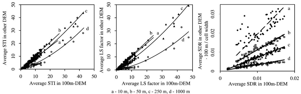
Fig. 6: Average STI, LS, and normalised average SDR for non-stream cells in relation to DEM100, all topographic calculated with neighbourhood-slope method ( $\beta_{\text{Nbh}}$ )
