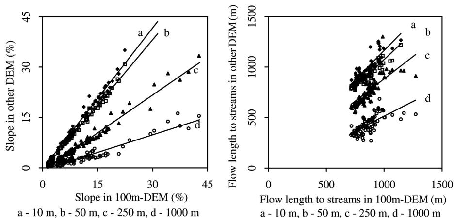
Fig. 3: Average slope and average flow length to streams in relation to DEM100, left: slope ( $\beta_{\text{Nbh}}$ ), right: flow length (ArcGIS)
