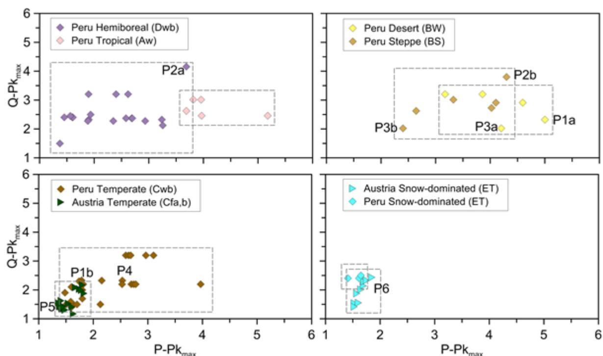
Figure 2.5: Relationship between maximum seasonality index of precipitation  $P-Pk_{max}$  and runoff  $Q-Pk_{max}$  stratified by Köppen climate classes for Peru and Austria: Labels refer to the example stations of Figure 2.2-2.4 top.
