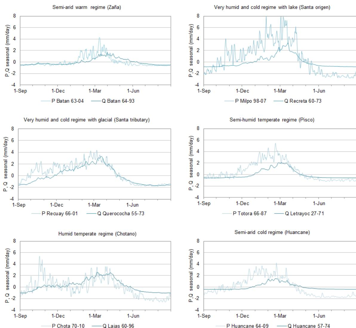
Figure 3.8: Intra-annual signal of precipitation (P) and runoff (Q) for the six hydro-climatic regimes.
