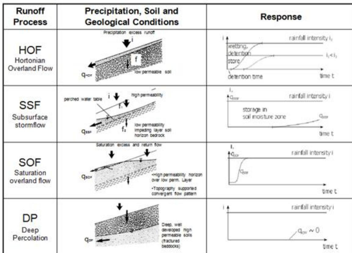
Figure 4.3: Schematic of runoff production mechanisms and runoff process dynamics (Gutknecht, Lecture notes).
