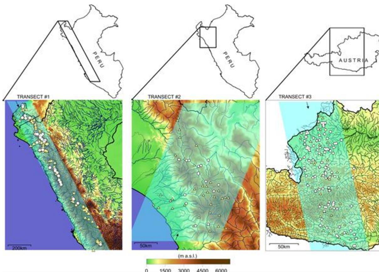
Figure 2.1: Topography and rivers of Peru (left: Transects 1 and 2) and Austria (right: Transect 3), with location of precipitation (triangles) and runoff stations (circles) along the transects.
