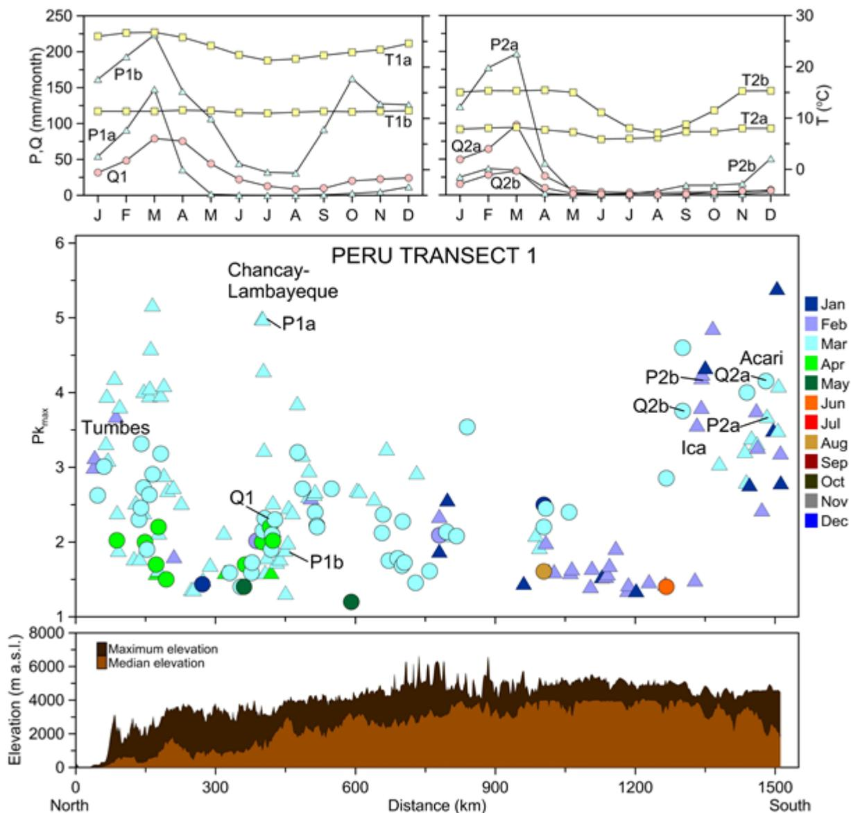
Figure 2.2: Top: Long term water balances for the Chancay-Lambayeque basin (2400 km<sup>2</sup>) (left), and the Ica (2600 km<sup>2</sup>) and Acari basins (250 km<sup>2</sup>) (right). Precipitation (triangles), runoff depths (circles) and air temperatures (squares). Middle: Maximum seasonality strength  $Pk_{max}$  and month of occurrence along Transect 1 for precipitation (triangles) and for runoff (circles). Bottom: median and maximum elevations of the transect.
