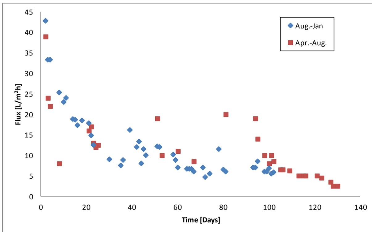
**Figure 3 - 3: Mean flux of pilot plant during 10 month operation in permeating phase**
