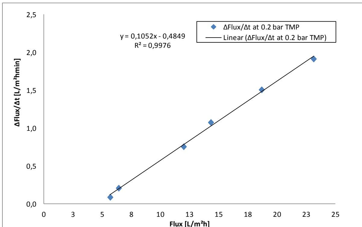
Figure 3 - 4: Flux drop during permeating phase of 6 min with constant pressure at different initial flux
