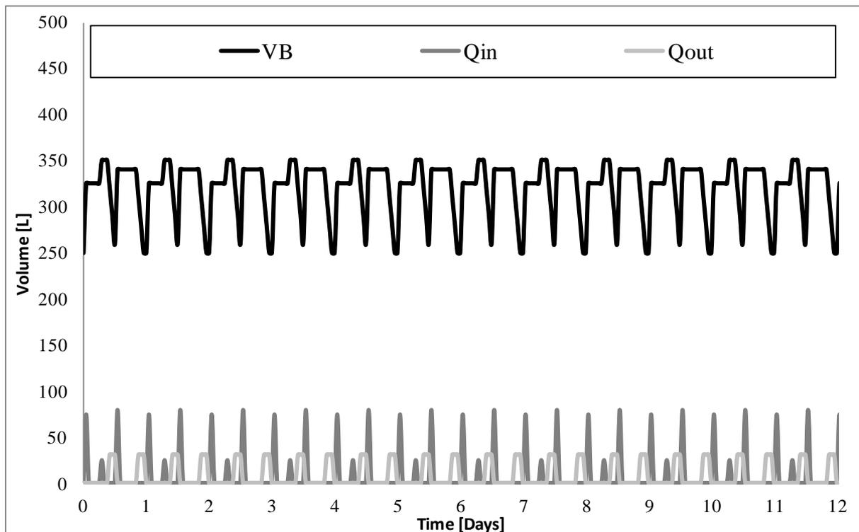
**Figure 5 - 1: Modelled hydraulic characteristics of bioreactor volume ( $V_B$ ), inflow ( $Q_{in}$ ) and effluent ( $Q_{out}$ )**
