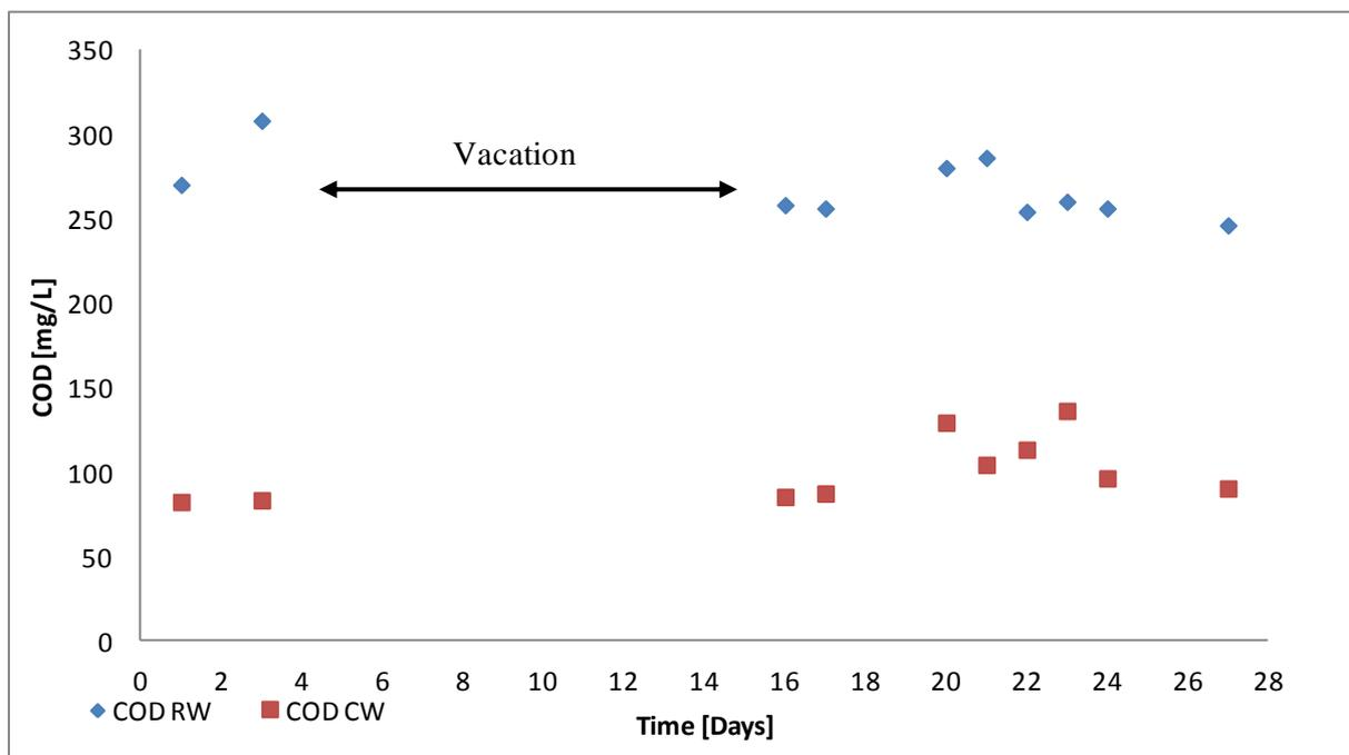
Figure 3 - 5: COD raw grey water (RW) and treated water (CW) before and after vacation
