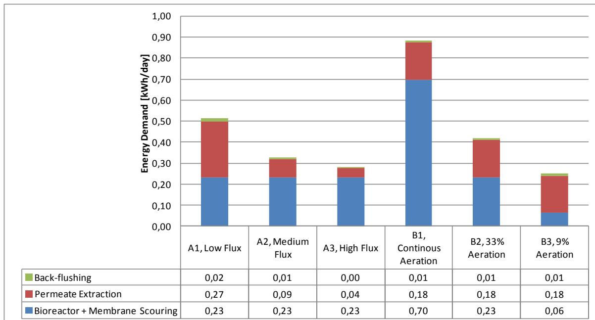
**Figure 3 - 9: Energy consumption of main equipment of MBBMR pilot plant**
