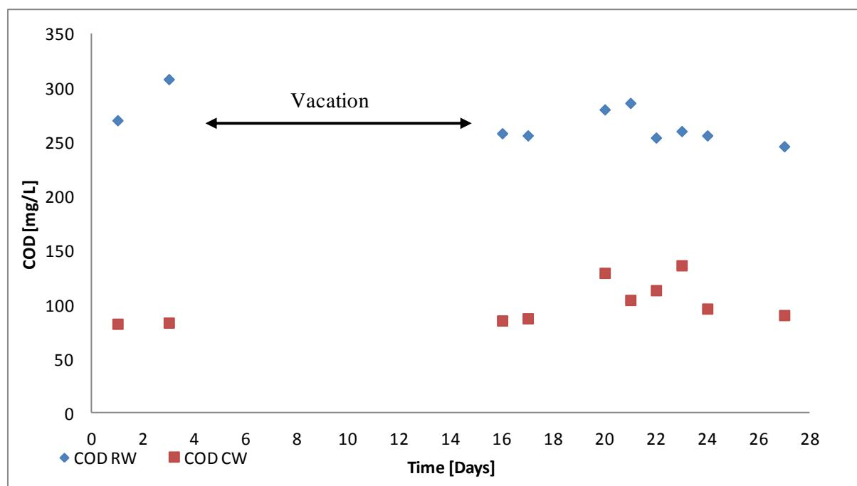
Figure 3 - 5: COD raw grey water (RW) and treated water (CW) before and after vacation
