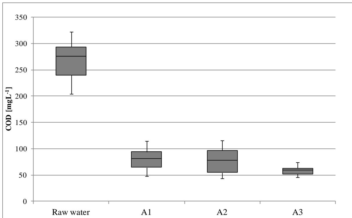
**Figure 4 - 3: COD removal efficiency depending on aeration rates (A1 0.19 Lm<sup>-2</sup>min<sup>-1</sup>, A2 0.38 Lm<sup>-2</sup>min<sup>-1</sup>, A3 0.67 Lm<sup>-2</sup>min<sup>-1</sup>). Bar chart analyses of each set-up including median, 25% and 75% quantile and whisker.**
