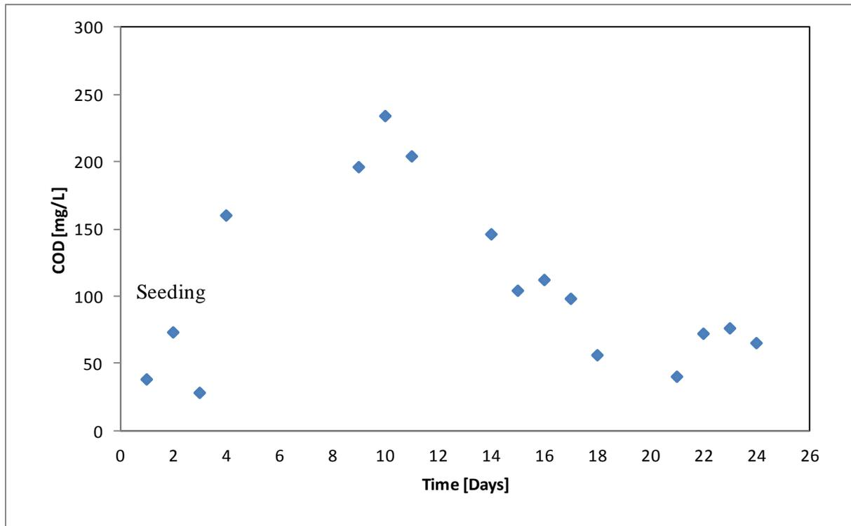
**Figure 3 - 2: COD development in treated water after start up with seed microorganism**
