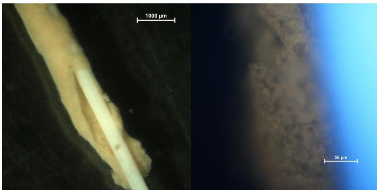
**Figure 4 - 5:** a) Stereo-microscopy of membrane fibre with biofilm-cover; scale bar represents 1000 µM;
