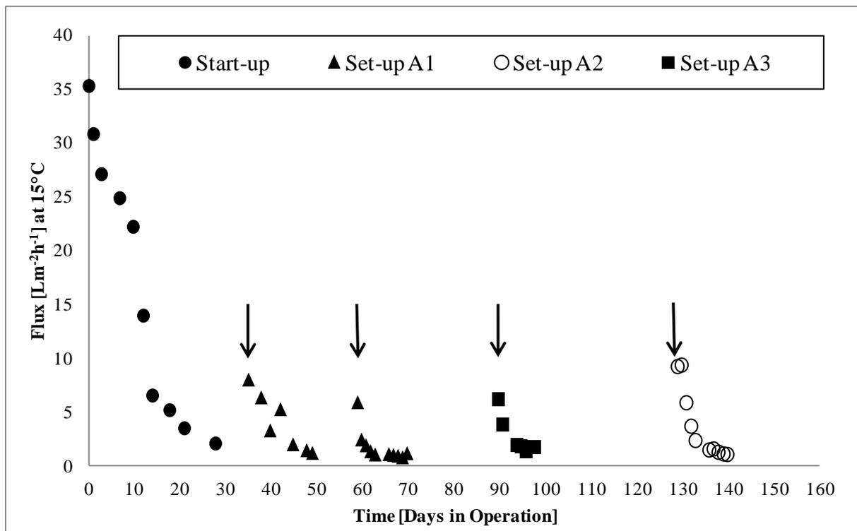
Figure 4 - 4: Flux stabilization after start-up (0.38 Lm<sup>-2</sup>min<sup>-1</sup>) and at different aeration rates (A1 0.19 Lm<sup>-2</sup>min<sup>-1</sup>, A2 0.38 Lm<sup>-2</sup>min<sup>-1</sup>, A3 0.67 Lm<sup>-2</sup>min<sup>-1</sup>), temperature corrected to 15°C, arrows indicate out-of-tank washes of membrane module.
