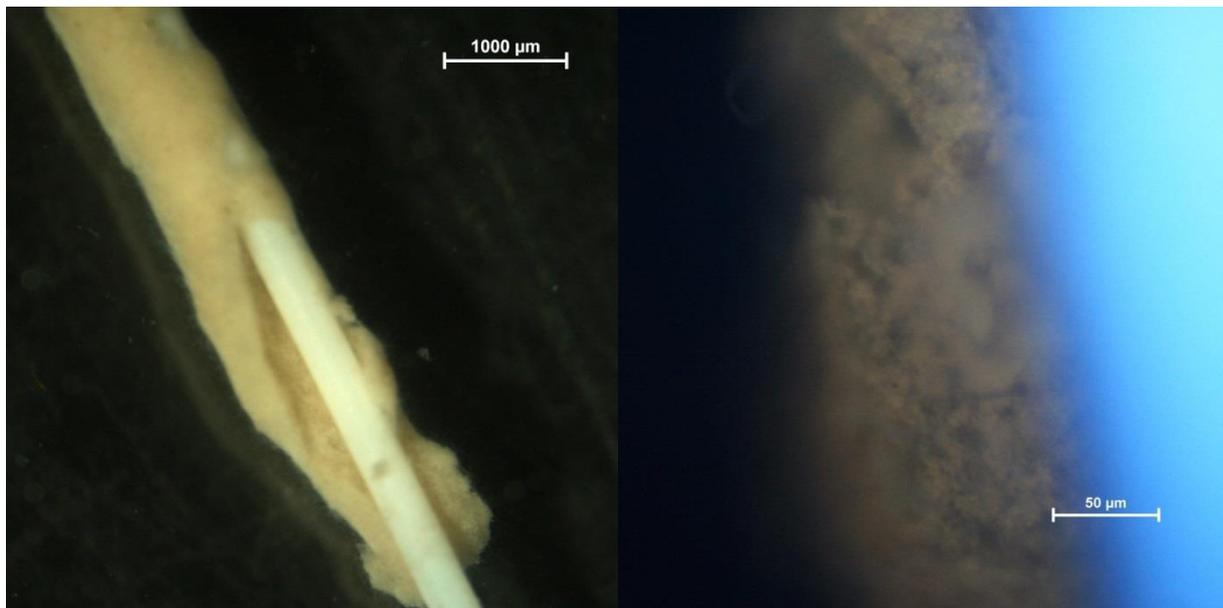
**Figure 4 - 5: a) Stereo-microscopy of membrane fibre with biofilm-cover; scale bar represents 1000 µm; b) Light microscopy picture of biofilm cross section touching UV-fluorescent membrane; scale bar represents 50 µm;**
