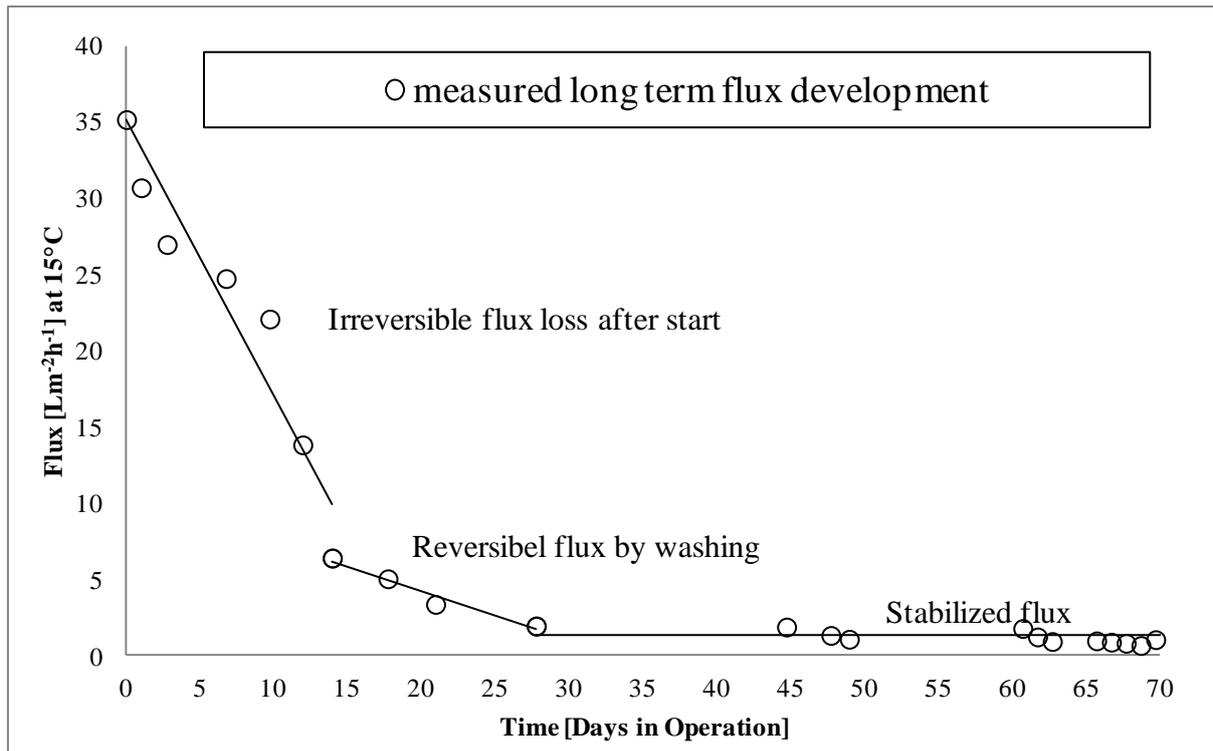
**Figure 4 - 2: Three stages of long-term flux stabilization of the fixed-fibre biofilm membrane reactor adapted from actual measured values by linear regression. First flux decrease describes the irreversible loss by pore blockings after start-up. The second flux decrease during operation is reversible by out-of-tank washings and the third trend represents the final flux bottom line after stabilization.**
