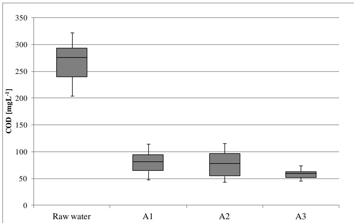
**Figure 4 - 3: COD removal efficiency depending on aeration rates (A1  $0.19 \text{ L m}^{-2} \text{ min}^{-1}$ , A2  $0.38 \text{ L m}^{-2} \text{ min}^{-1}$ , A3  $0.67 \text{ L m}^{-2} \text{ min}^{-1}$ ). Bar chart analyses of each set-up including median, 25% and 75% quantile and whisker.**
