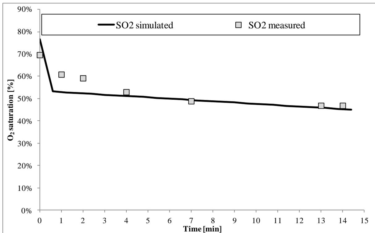
**Figure 5 - 3: Oxygen saturation decay in the bioreactor with switched-off aeration blower shortly after feeding fresh grey water. The straight line shows a comparison between modelled and measured  $\text{O}_2$ -saturation.**
