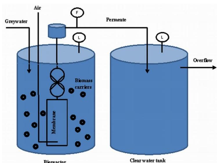
Figure 3 - 1: Flow diagram of Moving Bed Biofilm Membrane Reactor Pilot Plant
