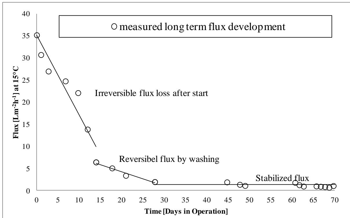
**Figure 4 - 2: Three stages of long-term flux stabilization of the fixed-fibre biofilm membrane reactor adapted from actual measured values by linear regression. First flux decrease describes the irreversible loss by pore blockings after start-up. The second flux decrease during operation is reversible by out-of-tank washings and the third trend represents the final flux bottom line after stabilization.**
