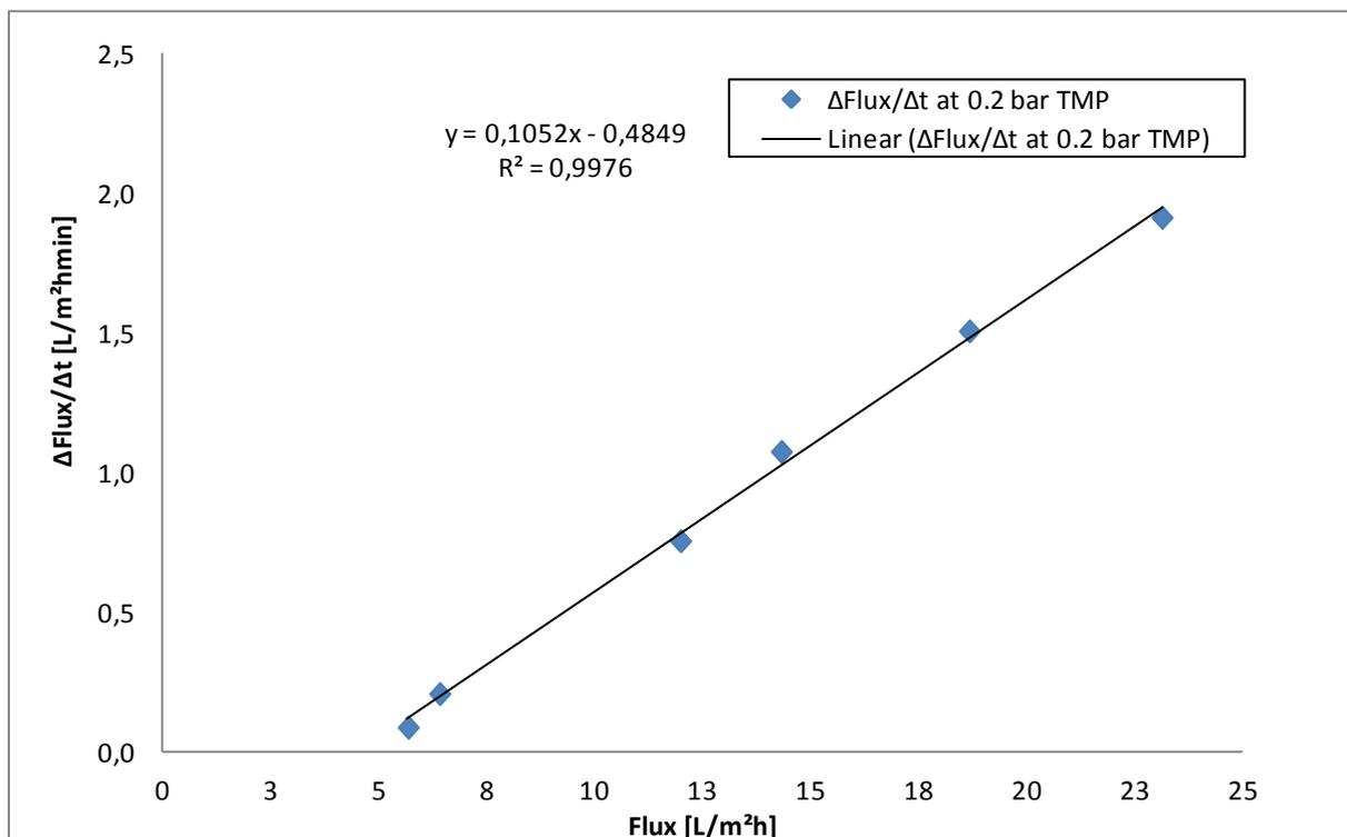
**Figure 3 - 4: Flux drop during permeating phase of 6 min with constant pressure at different initial flux**
