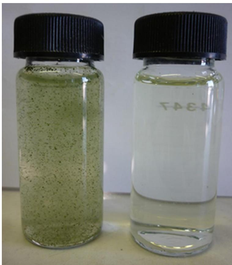
**Figure 3 - 6: Comparison of feed and treated water when Henna colour is used**
