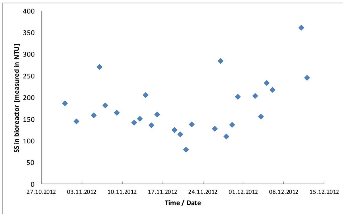
**Figure 3 - 8: Development of suspended solids concentration in the bioreactor during 7 weeks of operation**
