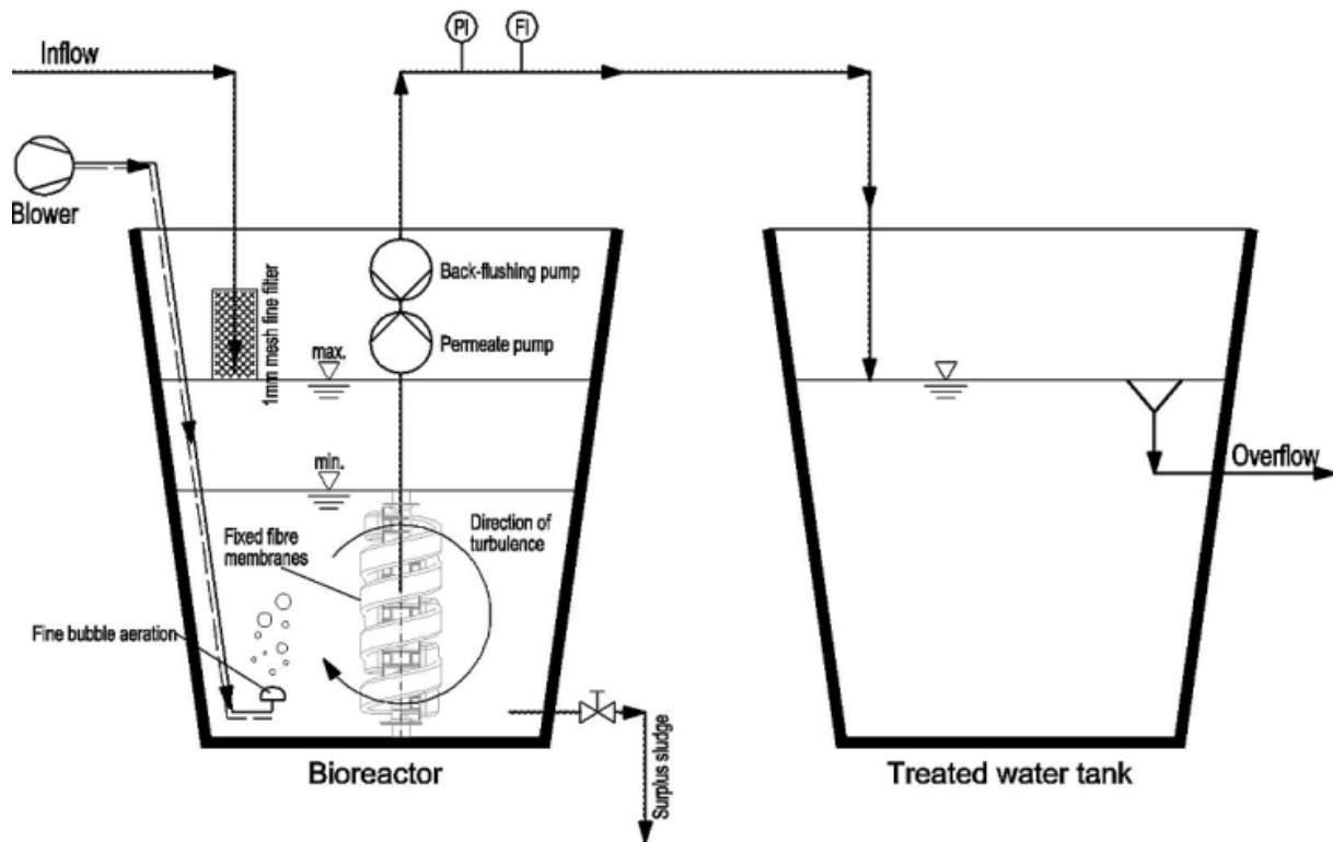
**Figure 4 - 1: Schematic diagram of the fixed-fibre biofilm membrane pilot plant**
