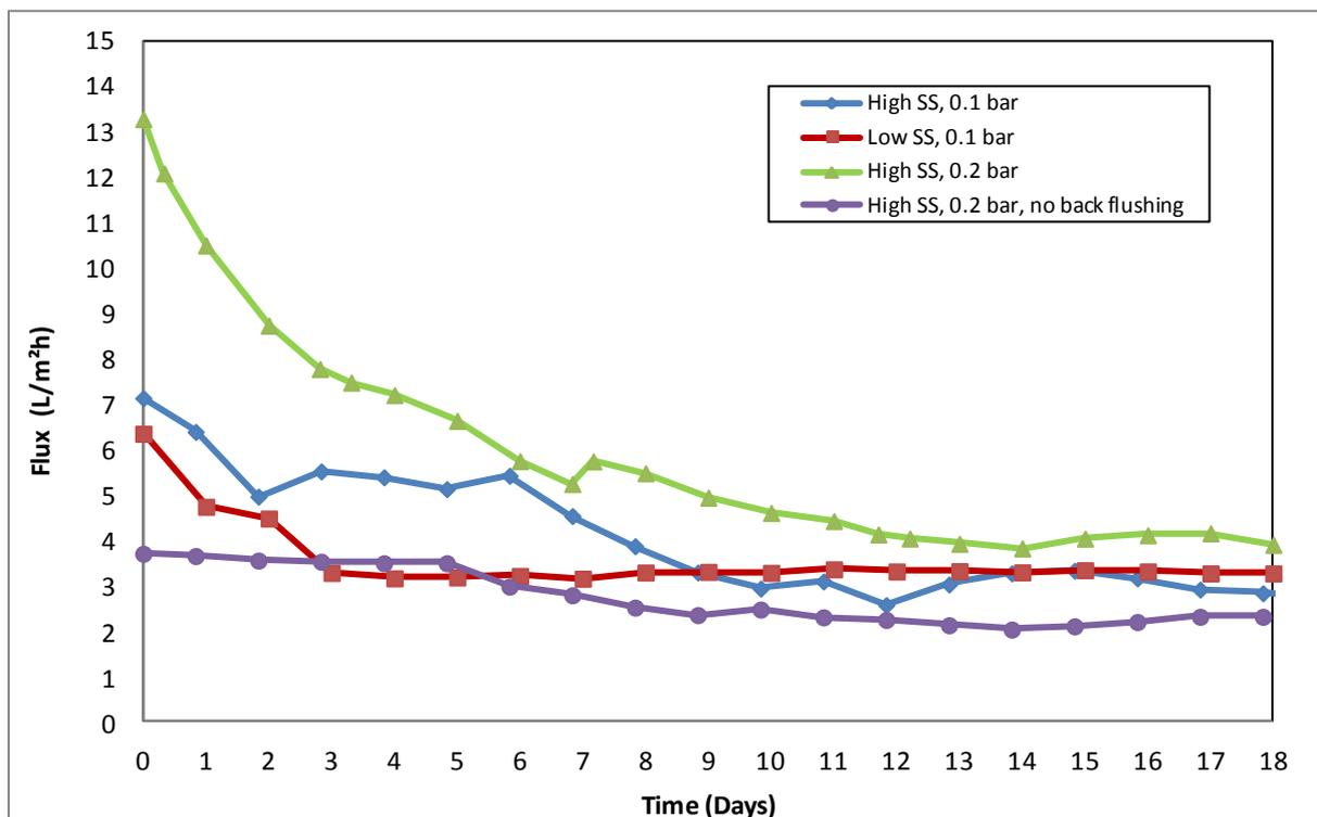
**Figure 2 - 3: Flux development during three weeks operation with different TMP and suspended solid (SS) concentration**
