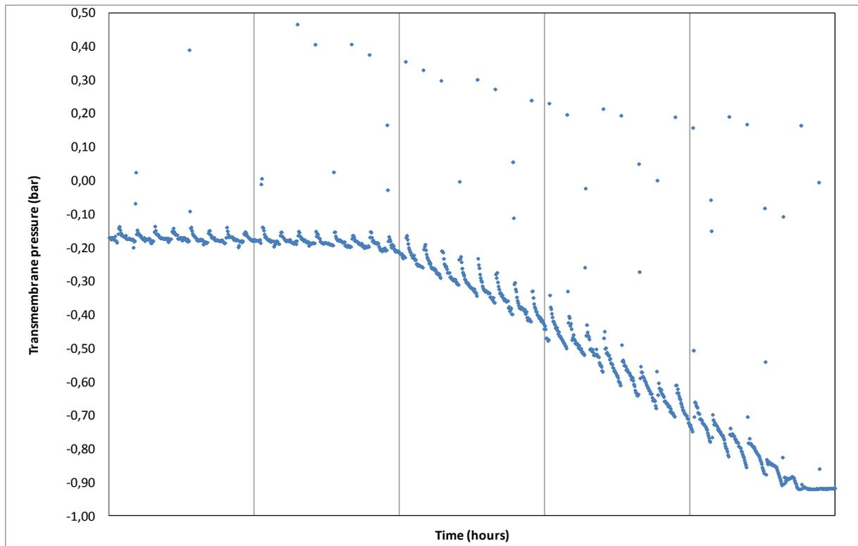
**Figure 2 - 2: Transmembrane pressure (TMP) during constant flow operation without back-flushing**
