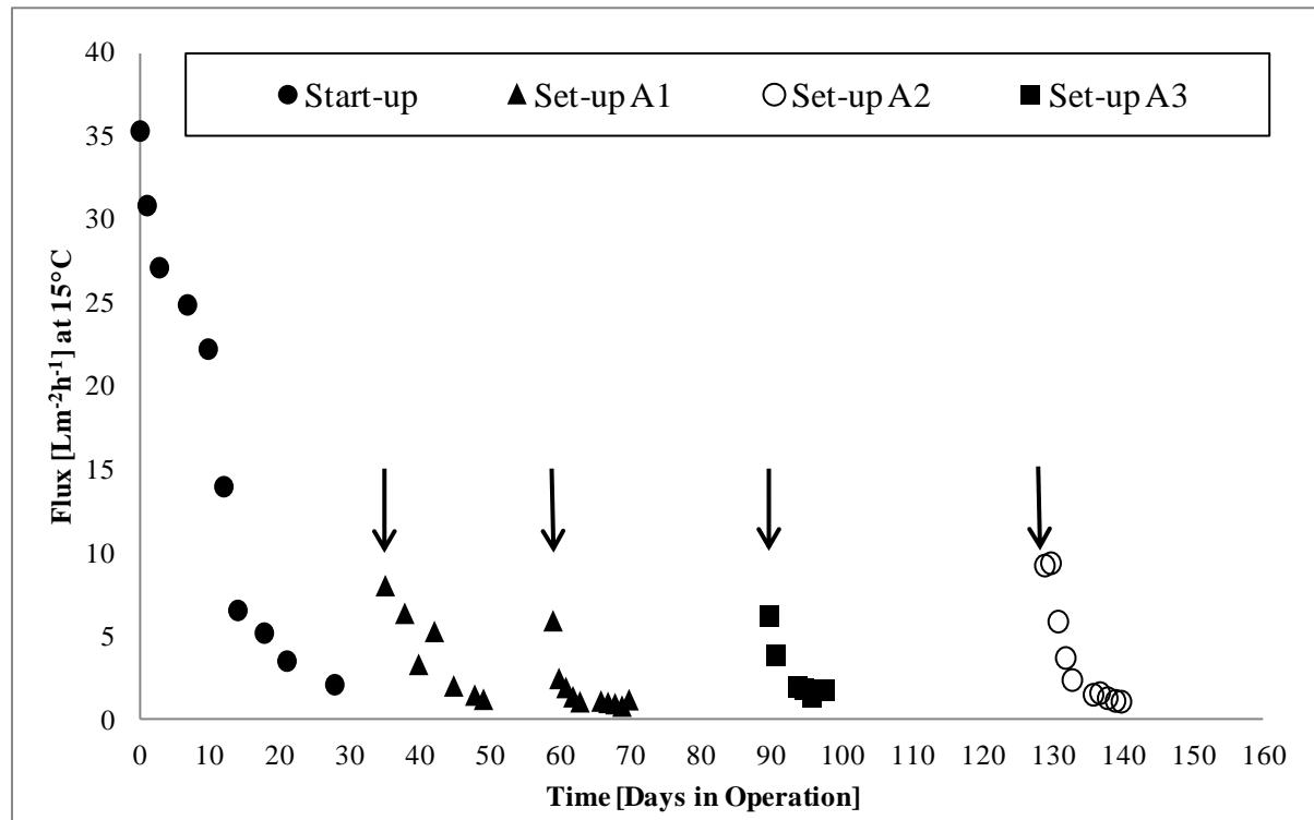
**Figure 4 - 4:** Flux stabilization after start-up ( $0.38 \text{ Lm}^{-2}\text{min}^{-1}$ ) and at different aeration rates (A1  $0.19 \text{ Lm}^{-2}\text{min}^{-1}$ , A2  $0.38 \text{ Lm}^{-2}\text{min}^{-1}$ , A3  $0.67 \text{ Lm}^{-2}\text{min}^{-1}$ ), temperature corrected to  $15^\circ\text{C}$ , arrows indicate out-of-tank washes of membrane module.
