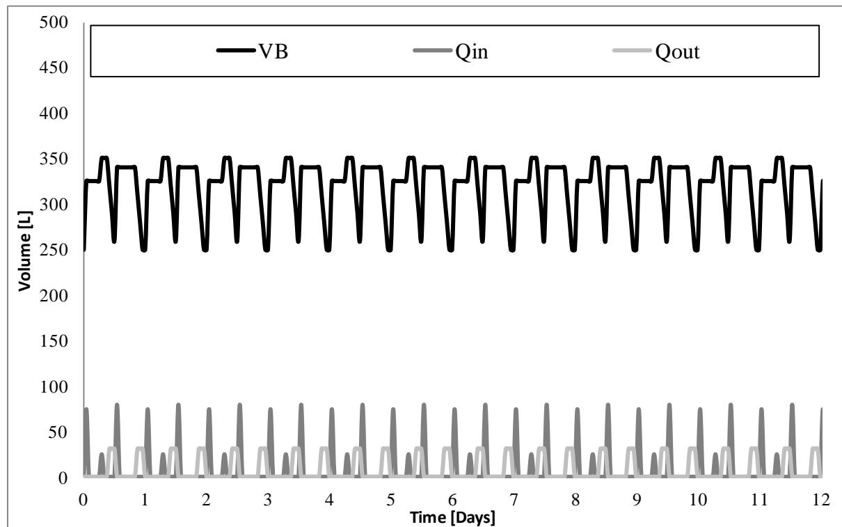
**Figure 5 - 1: Modelled hydraulic characteristics of bioreactor volume ( $V_B$ ), inflow ( $Q_{in}$ ) and effluent ( $Q_{out}$ )**
