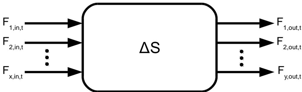
**Figure 1:** Simple balancing layout. Several fluxes may enter or leave a system, accumulation ( $\Delta S$ ) is possible.
