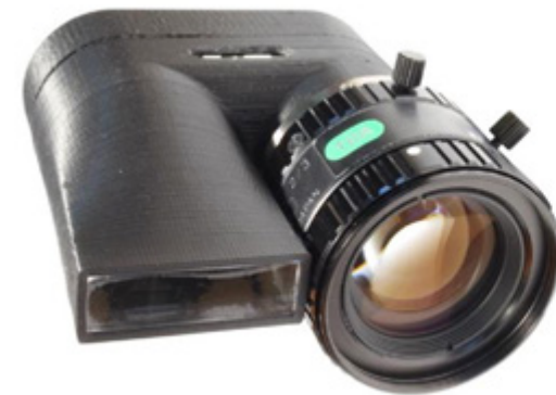
Fig.1 a) Solid-state LiDAR demonstrator b) Image data 3D representation
