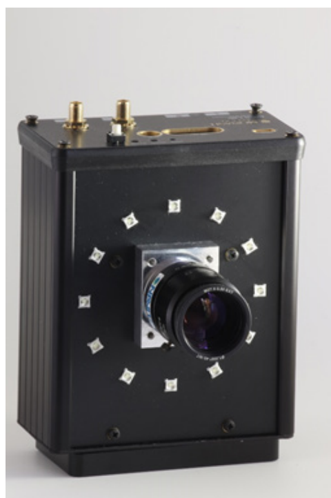
Fig. 1: VisionSens SPAD and Photodiode camera system developed by Monash University
