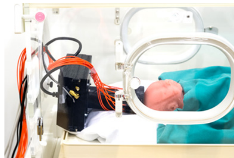
Fig. 1: NIROT measuring a realistic phantom of a preterm head in an incubator.
