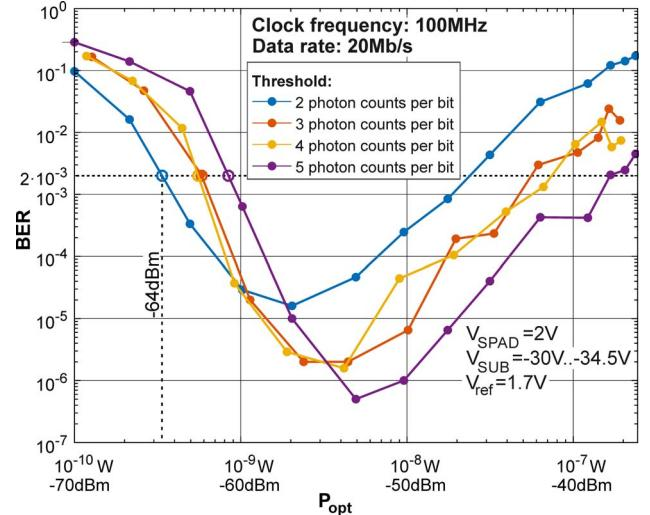
Fig. 6. BER measurements with an NRZ pseudo-random binary sequence (PRBS7) versus the mean optical power applied to the SPAD for different thresholds at 20 Mb/s.
