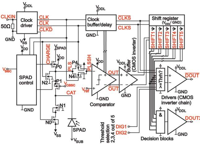
Fig. 1. Block diagram of the SPAD data receiver. N1 and P1 are cascode transistors to apply up to 6.6 V excess bias to the SPAD in this 3.3 V/0.35- $\mu$ m CMOS technology.
