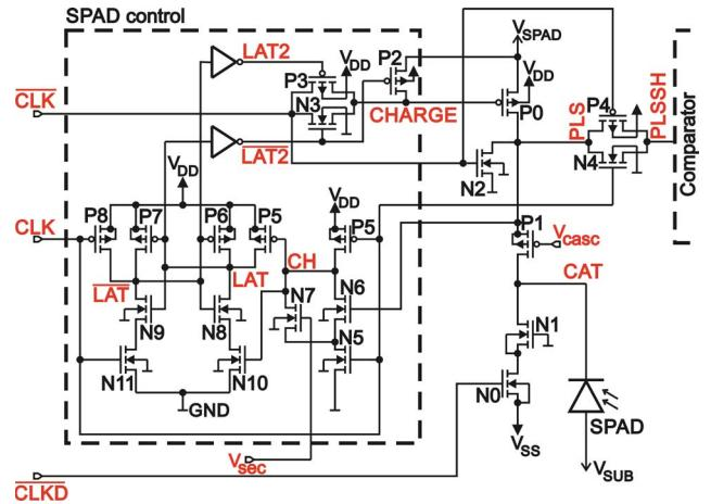
Fig. 3. SPAD control unit. The CMOS design avoids static power consumption (leakage currents neglected).
