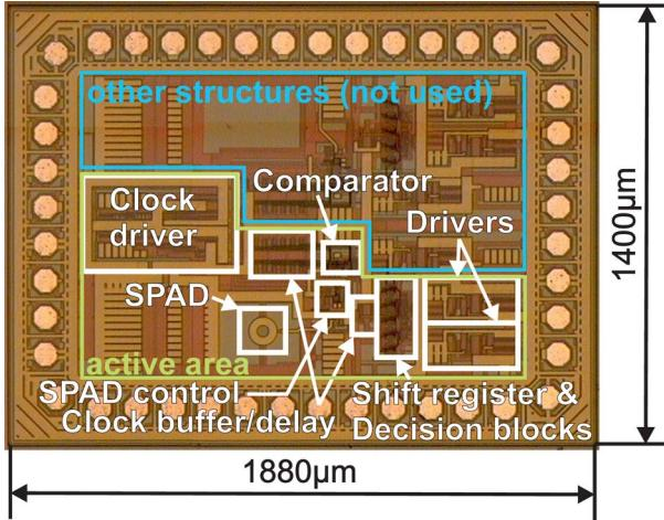
Fig. 5. Microphotograph of the fully integrated SPAD data receiver test chip. The active area of the receiver is  $0.66 \text{ mm}^2$ .
