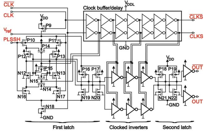
Fig. 4. Schematic of the clocked comparator with a second latch to store the decision during reset (SPAD quenched).
