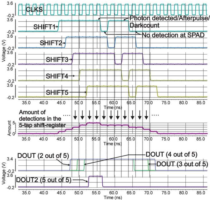
Fig. 2. Principle of operation of evaluating the pulse sequence from the SPAD to get DOUT and DOUT2. For a better understanding, DOUT instead of the inverted output  $\overline{\text{DOUT}}$  is shown.
