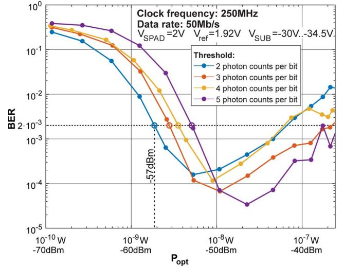
Fig. 7. BER measurements with an NRZ PRBS7 versus the mean optical power  $P_{\text{opt}}$  applied to the SPAD for different thresholds at 50 Mb/s.
