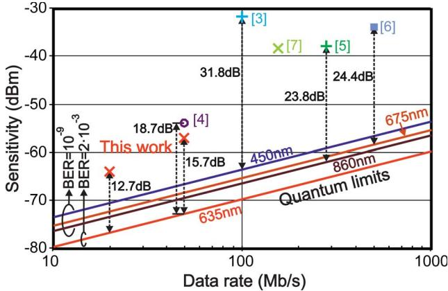
Fig. 8. Distance to the quantum limit of state-of-the-art results.
