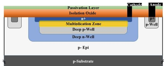
Fig. 1. Cross section of the  $n^+$ /DPW SPAD (not to scale).
