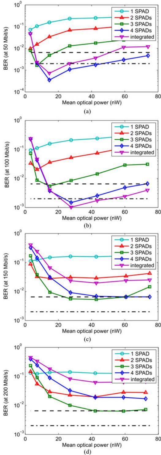
Fig. 7. BER at different optical power of the incident light; (a) 50 Mbit/s (b) 100 Mbit/s (c) 150 Mbit/s (d) 200 Mbit/s.
