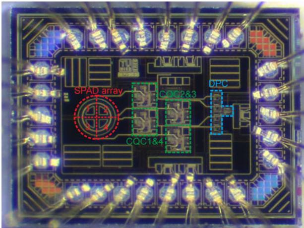
Fig. 5. Microphotograph of the receiver chip.
