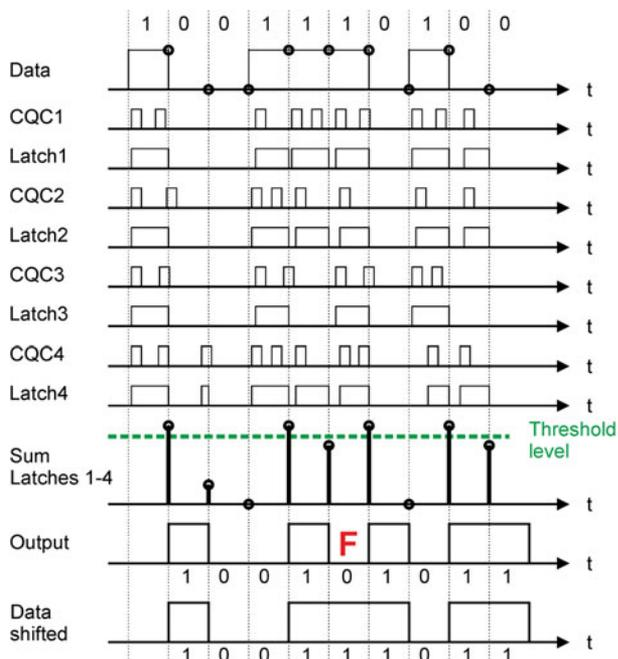
Fig. 6. Principle of digital latch-type processing of the 4 active quenching circuits (AQC) output data. The final output data are shifted by one bit period to the right compared to the input data.
