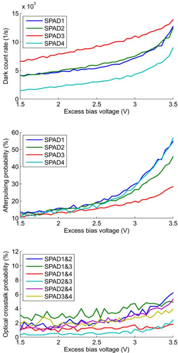
Fig. 2. DRC, AQC and OCTP (between 2 SPADs) at 25 °C.
