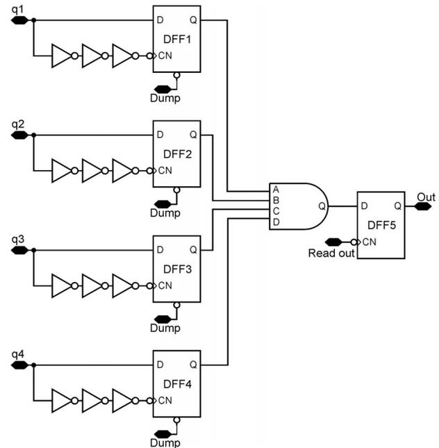
Fig. 4. Schematic diagram digital latch-type processing circuit.
