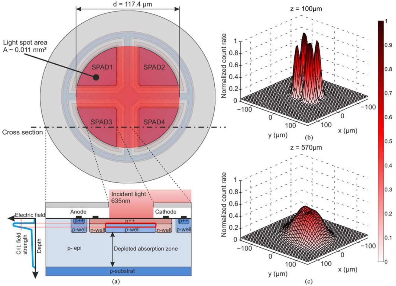
Fig. 1. Structure of the SPAD array. (a) Upper part: top view (not to scale), lower part: cross section and schematic electric field distribution (not to scale). (b) Surface scan with fiber tip  $\sim 120 \mu\text{m}$  above chip surface (c) Surface-scan with fiber tip  $\sim 1 \text{ mm}$  above chip surface.
