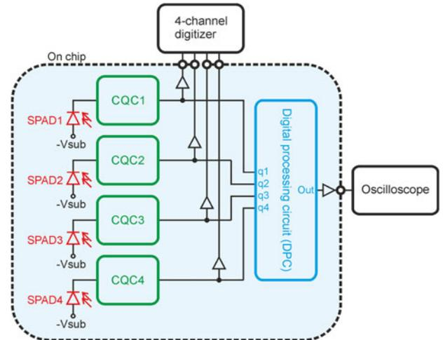
Fig. 3. Block diagram of the receiver chip and the connections of the outputs of the cascaded quenching circuits to the 4-channel digitizer and of the output of the digital processing circuit to the oscilloscope.
