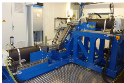
Universal test stand in power feedback configuration at TU Wien
