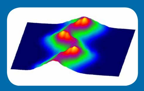
This picture illustrates the streaking of ejected electrons from Helium with attosecond half-cycle laser pulses.
