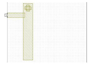
To subtract (de-embed) an amount of electrical length from the simulation results, the reference plane for the port must be moved away from the edge of the box.
