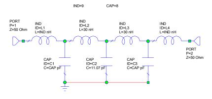
4 Click the "lpf3" schematic window to make it active. Change the C parameter value of CAP ID=C2 to the following value.
