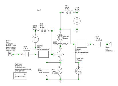
5 Specify the SWPVAR parameter settings shown in the following figure to define Vcc as a variable swept between 4 and 8 in steps of 0.5, then click **OK**.
