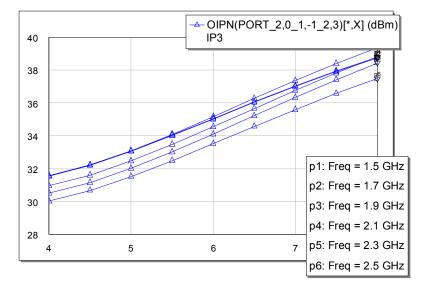
3 Choose **Simulate > Analyze** to obtain the output-referred IP3 intercept, swept over the bias voltage, as shown in the following graph.
