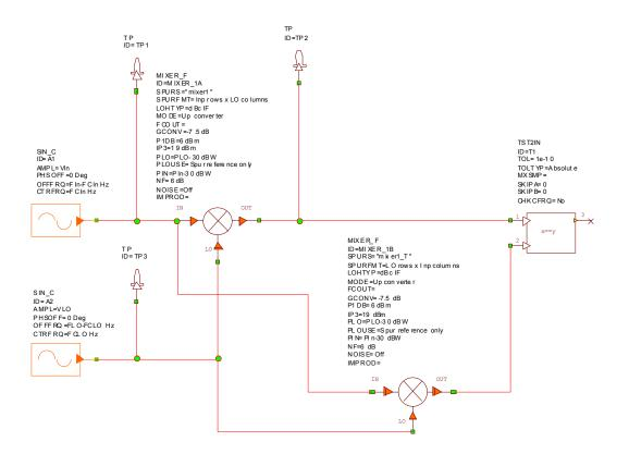
5 Import the "mixer1.txt" and "mixer1\_T.txt" data files located in the ProgramFiles\AWR\AWR2003\Examples\Getting Started\VSS\MIXER directory. In the "mixer1" data file, each row represents the input harmonic and each column represents the LO harmonic, with the top row and left column representing the first harmonic. The "mixer1\_T" data file is the transpose of the "mixer1" data file with rows representing LO harmonics and columns representing the input harmonic.
