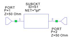
9 Create an index variable X=Xvector[1] in the same schematic, and change the NET parameter to "X" as shown in the following figure. (For details, see "Editing Element Parameters" on page 4-6.)
