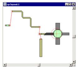
The red lines indicate that the faces of the layout cells are not snapped together.
