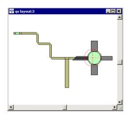
The "snap to fit" function finishes the routing of an MTRACE2 layout cell to a specified adjacent layout cell. In this example, the chip cap layout cell is moved and MTRACE2 re-routes to snap to the chip cap face.
