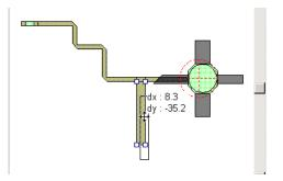
4 Repeat step 3 with the MTRACE2 element and the chip cap cell. Position the layout cells as shown in the following figure.
