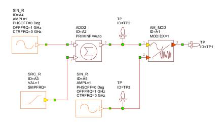
**TIP**: You can also connect blocks by moving them to snap their nodes together. When they are properly connected a small green square displays and the connection wire extends if you move either block. If you do not see the green square, try to drag one of the block into place again.
