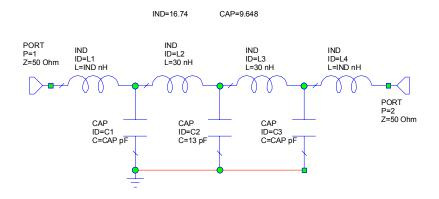
To create a schematic which contains a subcircuit that references the three schematics:
