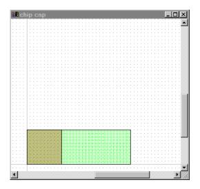
18 Click the copper square in the "chip cap" window, and press Ctrl+C then Ctrl+V to copy and paste it. Slide the mouse to position the copied square along the right edge of the rectangle as shown in the following figure, and click to place it.
