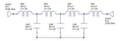
3 Repeat Step 1 to add a port to the right-most inductor, but right-click two times to rotate the port 180-degrees before you place it.
