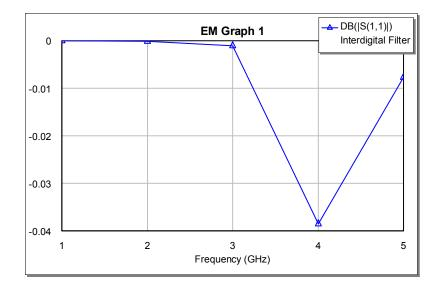
To determine a more precise measurement of the resonant frequency, you must change the frequency range and step size of the simulation.
