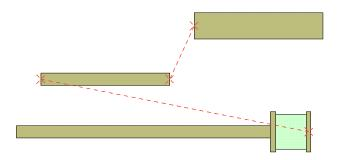
The resulting layout contains layout cells representing electrical components floating in the layout window. Choose **Edit > Snap Together** to snap the faces of the layout cells together. The following figure shows the layout view from the previous figure after a snap together operation.
