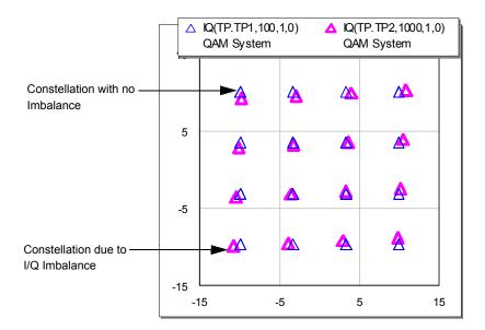
The INP\_IMBAL block has an amplitude imbalance of 0.6, a phase imbalance of 6 degrees and a DC offset value of 20e-3 (or 0.02). If the DC offset value is zero, ideally it should produce an image rejection ratio (IRR) of 24 dBW. Here, you display the IRR for tones.
