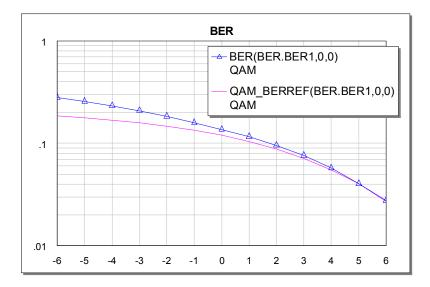
The simulation stops when 25 errors are counted at  $Eb_NO = 6dB$ . The simulation response in the following graph should display.
