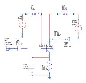
4 In the Element Browser, click the **Subcircuits** category then select the "input match" subcircuit and place it on the schematic between CAP C1 and node 1 of the GBJT transistor as shown in the following figure.
