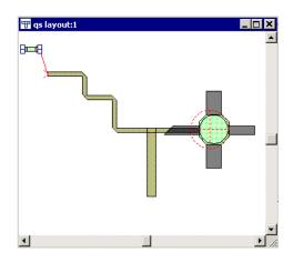
10 Select the MTRACE2 layout cell, hold down the **Shift** key and select the chip cap artwork cell.
