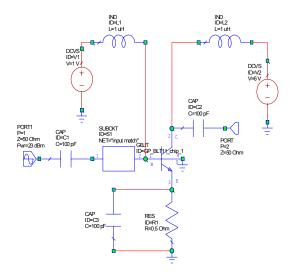
5 If the subcircuit nodes do not properly connect with the capacitor and transistor you may need to slightly move the elements until the proper connections are made.
