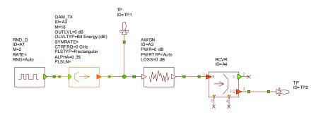
10 Double-click the RND\_D block in the system diagram and verify that the M parameter is **2**.
