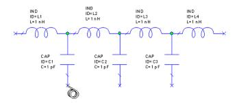
2 Click, then drag the wire past the bottom node of CAP C2, then onto the bottom node of CAP C3, and click to place the wire.
