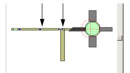
3 Move the routing tool to the desired point and click to place. (Right-click to delete the last point; press the **Esc** key to cancel the activity.)
