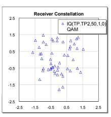
The received constellation does not appear as expected because the power spectral density of the noise source is set to 0 dB. Note that the time waveform of the complex baseband signal does not show eight samples per symbol as specified in the System Simulator Options dialog box.
