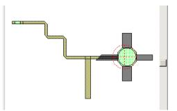
**TIP:** MLIN is a straight element with a width you can change in the layout. You can edit the MTRACE2 elements in the layout to create jogs and bends and chamfered corners. You can edit the MCTRACE element to create jogs and bends with rounded corners.
