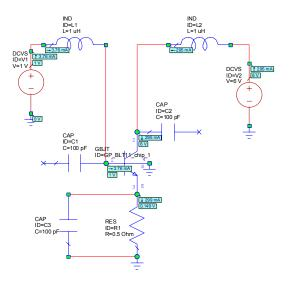
7 Connect a wire between the bottom node of CAP C3 and ground.
