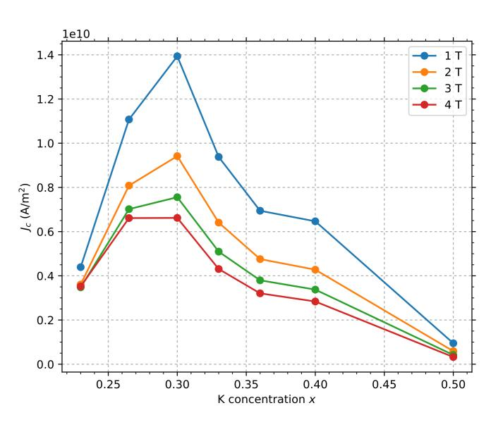
• Introduction of defects from fast neutron irradiation  $\Rightarrow$  increase of  $J_c$  over the whole doping range.  $J_c$  at  ${\bf 5}$   ${\bf K}$  and different applied fields:
