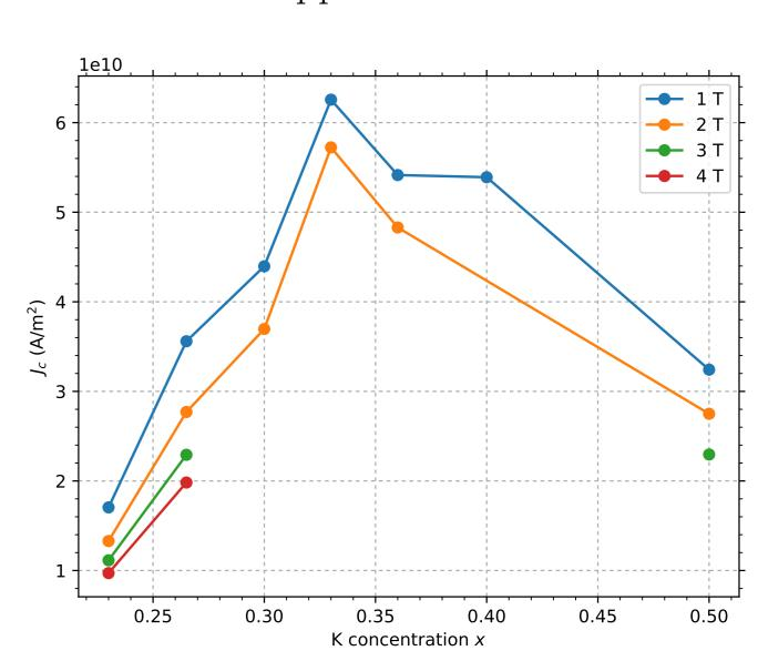
• Enhancement of  $J_c$  due to fast neutron irradiation as a function of the K concentration:
