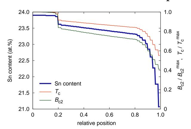
The simulation results shown here were obtained using the Sn concentration profile on the left. Similar to the distribution measured by SEM-EDX, the Sn content exhibits a small plateau near the sub-element core, then decreases linearly towards the outside, and drops steeply near the barrier.
