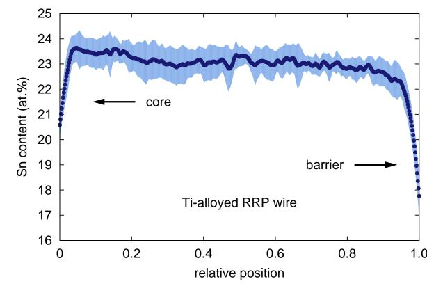
Scanning electron microscopy studies revealed a Sn concentration gradient of approx. 0.1 at.%/µm within the sub-elements of stateof-the-art Nb<sub>3</sub>Sn wires. This A-15 inhomogeneity causes a gradient in  $T_c$  (and consequently  $B_{c2}$ ), which can be probed for instance by AC magnetometry and scanning Hall probe microscopy. [3]
