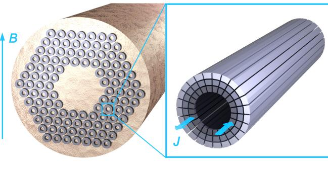
We simulate  $J_c(B)$  of Nb<sub>3</sub>Sn wires for both magnetometry and transport in perpendicularly applied field. Assuming all sub-elements within a wire are identical, the behavior of one of them is simulated.
