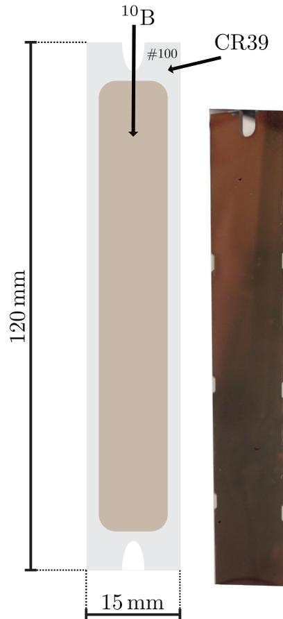
**Figure 8.1.:** On the left: CR39, <sup>10</sup>B detector dimensions. On the right: Photo of a CR39 plate detector with <sup>10</sup>B coating.
